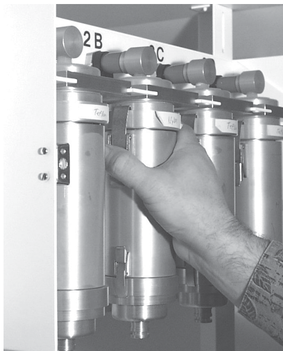
Figure 4-21. The inlet port on the ChemComb should fit securely inside the hose connection.
