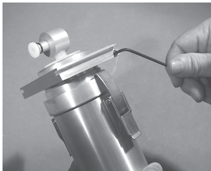
Figure 4-17. Tighten the collar's screw with a 7/64 hex wrench.
