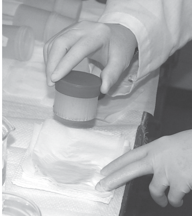
Figure 3-33. Gently tap the open end of the denuder on a stack of clean Kimwipes to remove any liquid bubbles in the denuder tubes.
