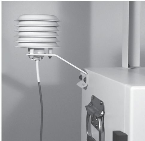
Figure 2-68. Ambient temperature probe assembly mounted on the enclosure.
