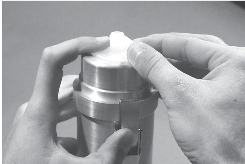
Figure 4-3. Applying Teflon tape to the plastic hose connection insert.
