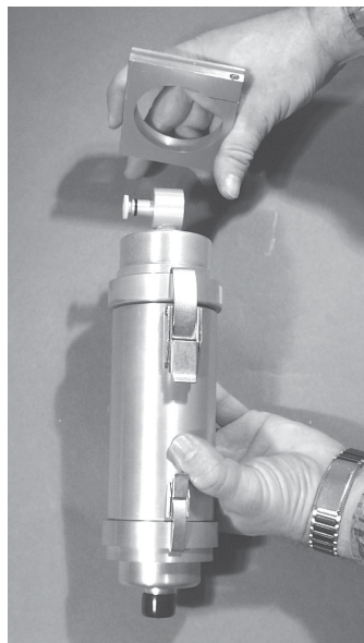
Figures 4-14 (left) and 4-15 (right). Sliding the collar onto the top rim (filter pack outlet port) of a ChemComb cartridge.
