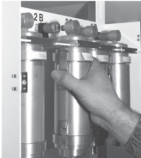
Figure 4-20. Sliding the ChemComb cartridge onto the tray.
