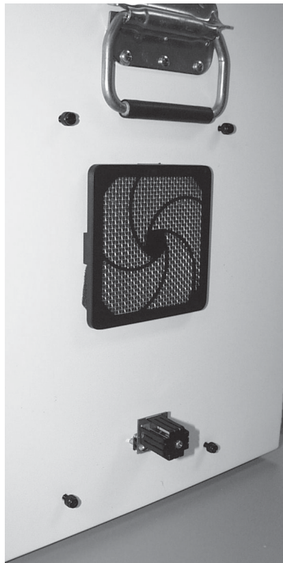
Figure 2-4. Relative humidity sensor installed on right side panel of the unit.
