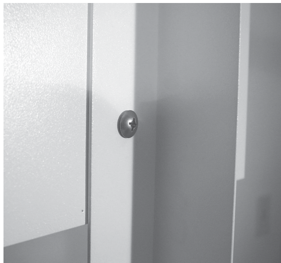
Figure 2-43. Insert the screws in the bottom holes of the shelter box.
