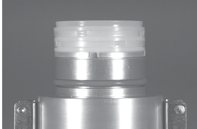
Figure 3-47. Three plastic filter screens installed on the body of a ChemComb cartridge.
