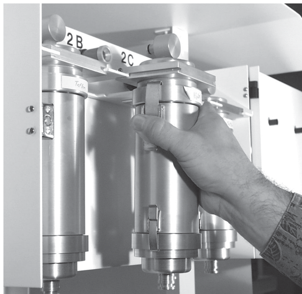
Figure 4-19. Aligning the groove of the collar on the ChemComb with the edges of the tray inside the shelter box.
