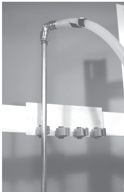
Figure 2-26. Push the pipe into the clip on the hose clip plate.
