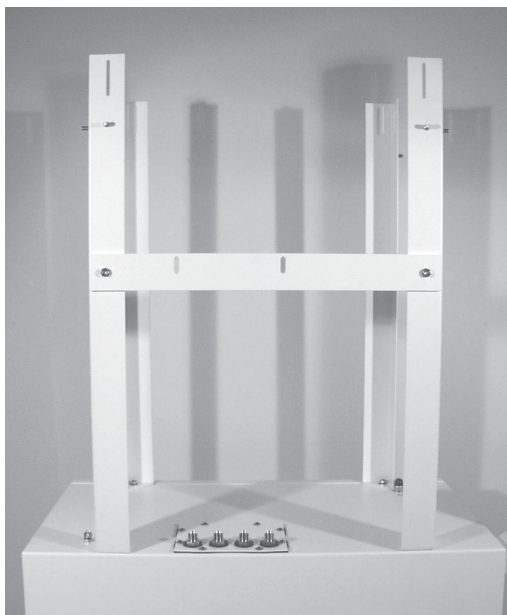
Figure 2-10. Hose assembly mounting plate positioned on the shelter legs.
