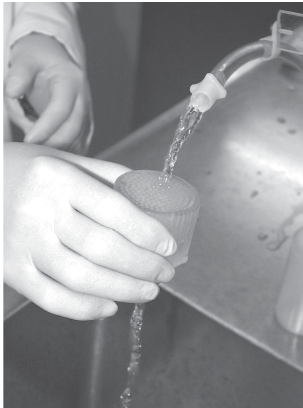
Figure 3-19. Flushing the HC with distilled water.
