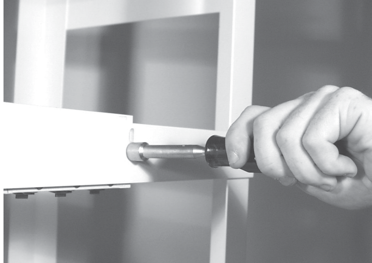
Figure 2-23. Secure the hose clip plate to the hose assembly mounting plate.
