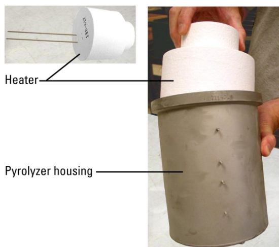
Figure 8-7. Insert replacement heater into housing
