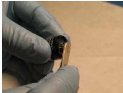
Figure 7–11. Pressing Down the PID Lamp
