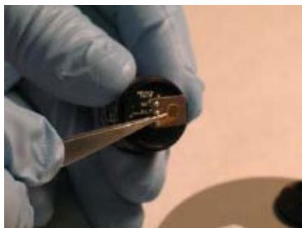
Figure 7-7. Removing the Cell Assembly
