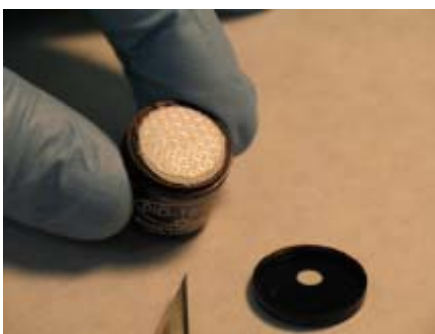
Figure 7-5. Removing the Filter Media
