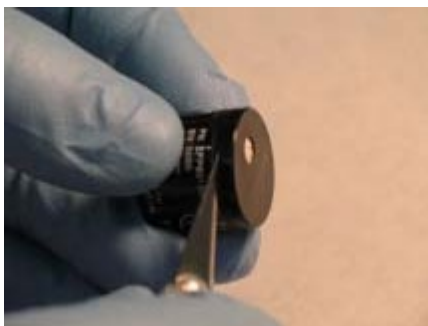
Figure 7-4. Removing the Filter Cap
