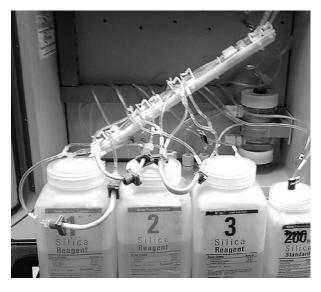
4. Remove/unscrew left tubing panel standoff screw.
