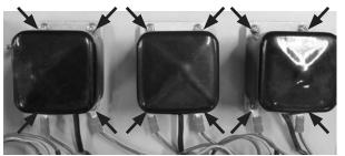
10. These four screws are for the pump head, remove them and replace with new pump head. Repeat procedure for the next two pump heads.
