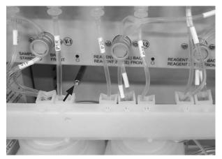
5. Remove bottom two hinge screws below pump fluidic panel.
