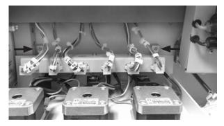
9. Take out the panel and at the back of the panel, loosen all 12 screws on three pump monitors.
