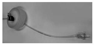
2. Place a cable tie on the tube to secure the check valve after inserting into the tubing.
