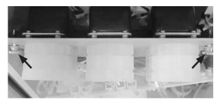
7. Disconnect all electrical pump and valve connectors by unplugging the 6 white connectors.
