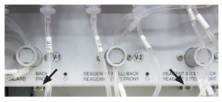
6. Loosen two metal thumb screws and swing down pump panel.
