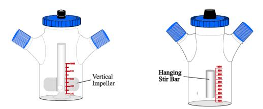
**Note:** Spinning speed needs to be optimized based on the impeller blade used. Start at the lowest spinning speed and incrementally increase the speed until it is optimized to achieve 24–30 hours doubling time, good cell viability, and low cell clumping.
