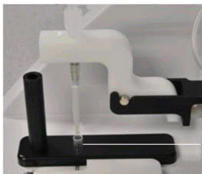
Install a new, opened 0.2-mL PCR tube into the hole of the Tip Loader
