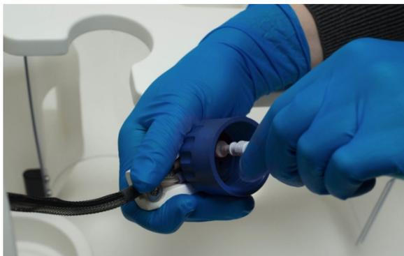
7. Immediately attach the prepared Wash 2 Bottle in the W2 position and tighten the cap. Press **Next**.
