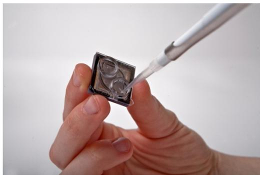
2. Insert the pipette tip firmly into the loading port and remove as much liquid as possible from the loading port. Discard the liquid.
