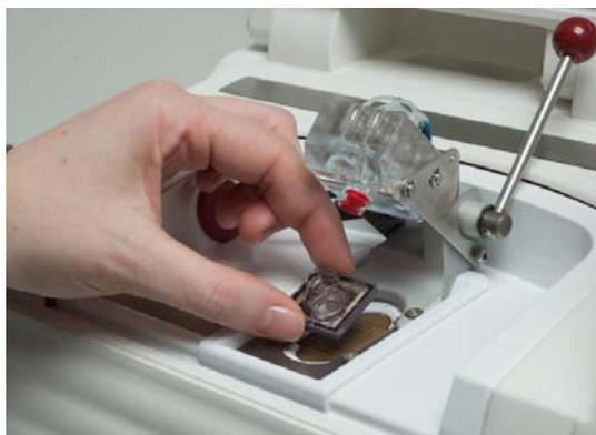
5. When prompted, use the barcode scanner to scan the barcode located on the chip package, or press **Change** to enter the barcode manually.
