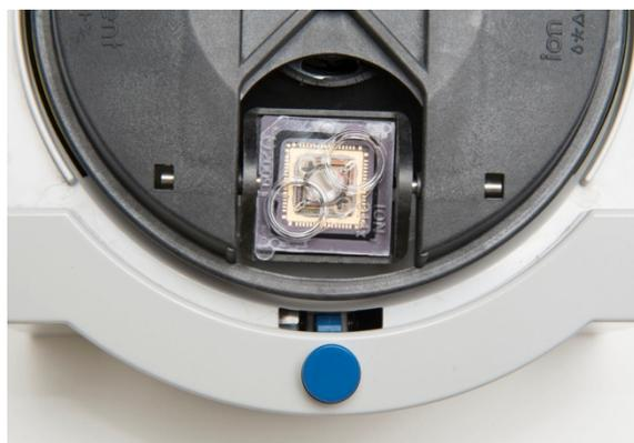
9. Repeat the chip mixing in step 7, then spin for 30 seconds **with the chip tab pointing in** (toward the center of the MiniFuge).
