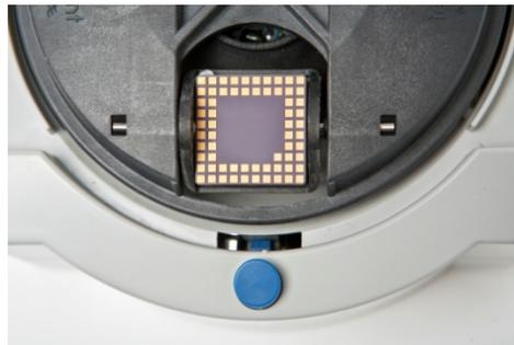
4. Centrifuge for 5 seconds to completely empty the chip. Remove the chip from the bucket and wipe off any liquid on the bucket.
