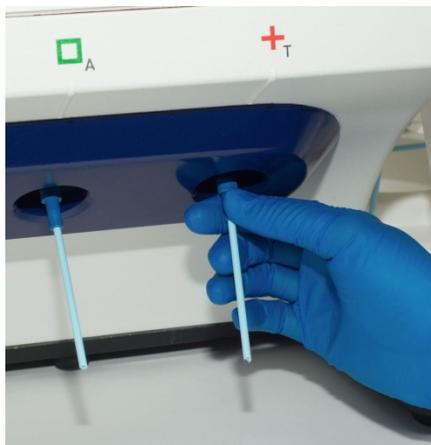
3. Attach each Reagent Bottle to the correct dNTP port and tighten firmly until snug. The correct order of the Reagent Bottles on the Ion PGM™ System is dGTP, dCTP, dATP, and dTTP (left to right when facing the instrument).
