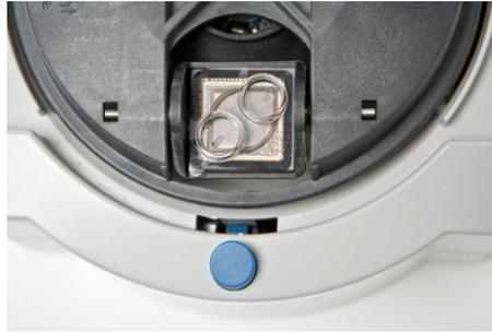
9. Repeat the chip mixing in step 7 one more time, then spin for 30 seconds **with the chip tab pointing in** (toward the center of the MiniFuge).
