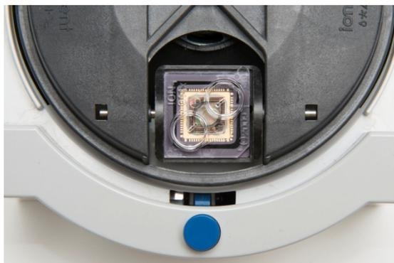
6. Centrifuge for 30 seconds, then remove the chip from the centrifuge bucket.
