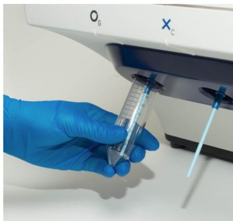
**Note:** The Ion PGM™ System checks the pressure of the Reagent Bottles and Wash Bottles. If a bottle leaks, you are prompted to check that it is tightly attached to the instrument. If it continues to leak, it should be replaced. If the instrument still does not pass the leak check, contact Technical Support.
