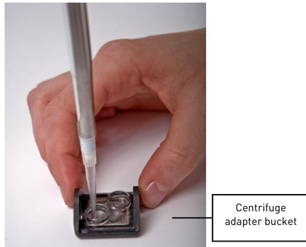
1. Place the Ion PGM™ Chip back in the centrifuge adapter bucket and place the bucket on a flat, stable surface such as a benchtop.
