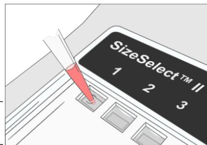
3. Load 25  $\mu$ L of ready-to-use E-Gel™ Sizing DNA Ladder into the marker well.
