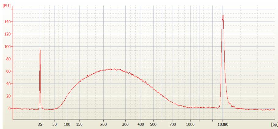
Panel A, Optimal fragmentation profile: 1 µg of *E. coli* DH10B DNA was fragmented with the Ion Xpress™ Plus Fragment Library Kit with a reaction time that was adjusted for 200-base-read libraries. Analysis was performed using the Agilent™ High Sensitivity DNA Kit. Peaks at 35 bp and 10,380 bp represent low- and high-molecular weight markers.
