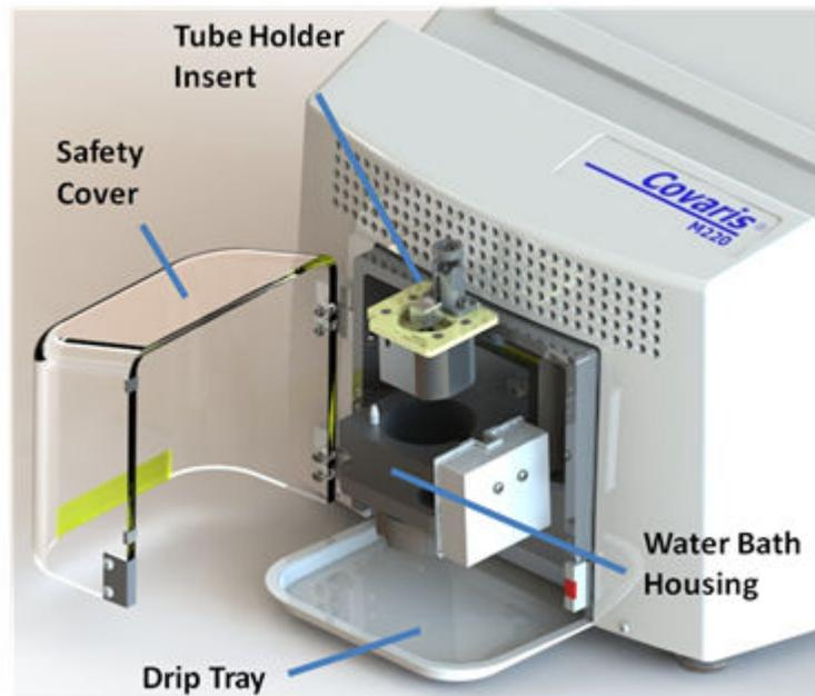
1. Open the safety cover, then place the Tube Holder (Covaris™ M220 Holder XTU) into the water bath housing.
