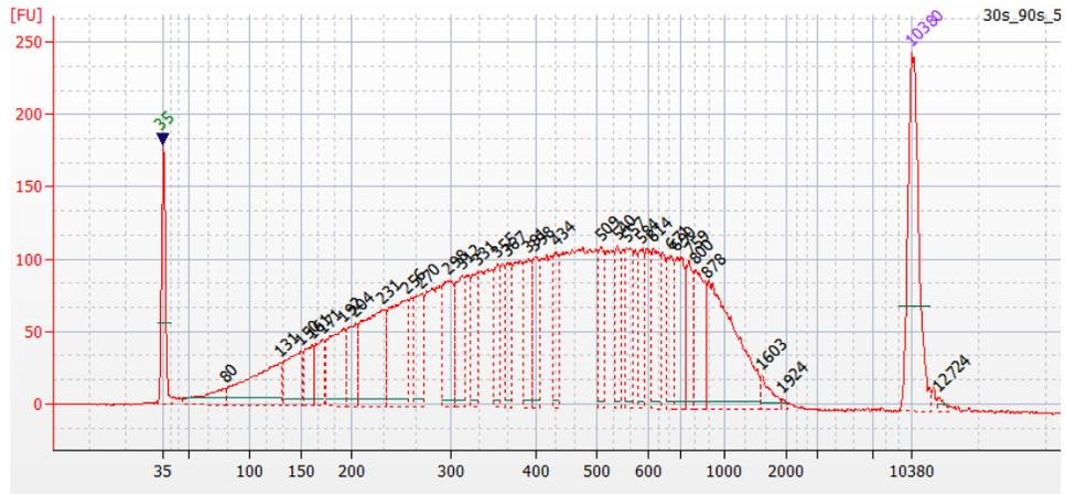
1 µg of *E. coli* DH10B DNA was fragmented with the Bioruptor™ NGS System for 20 minutes. Analysis was with the Agilent™ High Sensitivity DNA Kit. Peaks at 35 bp and 10380 bp represent low- and high-molecular weight markers.
