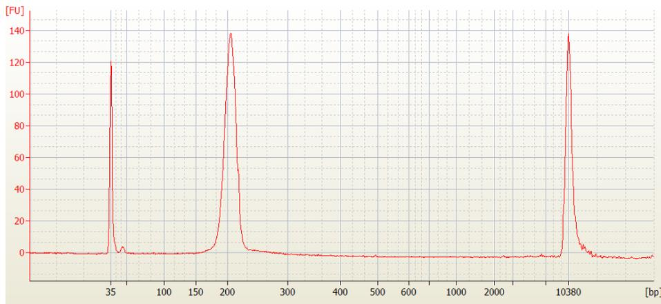
1  $\mu\text{g}$  of *E. coli* DH10B DNA was fragmented with the Ion Shear™ Plus Reagents with a reaction time adjusted for 100-base-read libraries. An unamplified library was prepared from the fragmented DNA and size-selected with the 2% E-Gel™ SizeSelect™ II Agarose Gel for 100-base-read libraries (200-bp length), as described in this user guide. Analysis was with the Agilent™ High Sensitivity DNA Kit. Peaks at 35 bp and 10380 bp represent low- and high-molecular weight markers.
