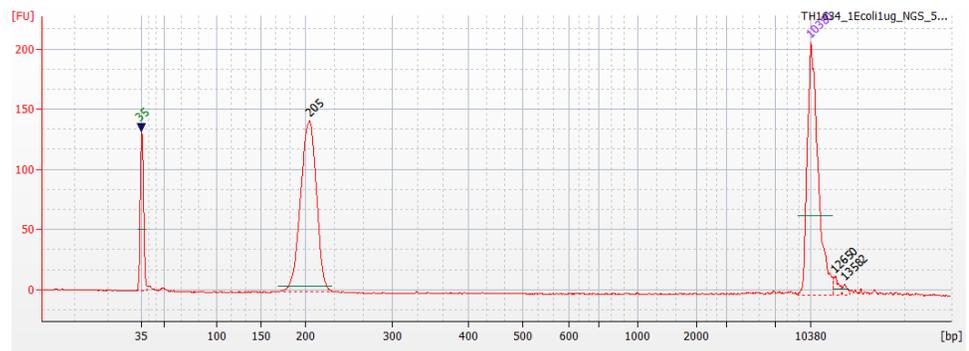
*E. coli* DH10B DNA was fragmented with the Bioruptor™ NGS System for 17 minutes, then size-selected with the Pippin Prep™ instrument.
