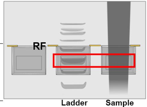
2. Tap **Done** to end the protocol and stop the gel, then recover the sample with a pipette into a clean 1.5-mL Eppendorf LoBind™ tube.
