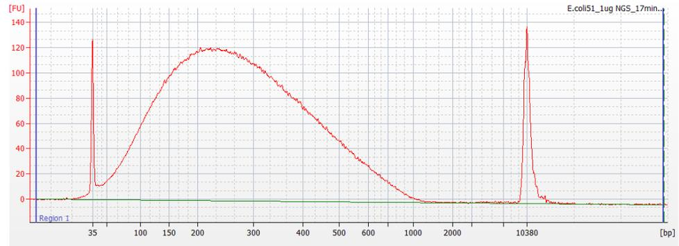
1 µg of *E. coli* DH10B DNA was fragmented with the Bioruptor™ NGS System for 17 minutes. Analysis was with the Agilent™ High Sensitivity DNA Kit. Peaks at 35 bp and 10380 bp represent low- and high-molecular weight markers.
