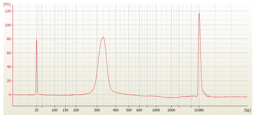
Panel A, 1 µg of *E. coli* DH10B DNA was fragmented with the Ion Shear™ Plus Reagents with a reaction time adjusted for 200-base-read libraries. An unamplified library was prepared from the fragmented DNA and size-selected with the 2% E-Gel™ SizeSelect™ II Agarose Gel for 200-base-read libraries (330-bp length), as described in this user guide. Analysis was with the Agilent™ High Sensitivity DNA Kit.
