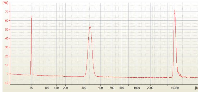
1 µg of *E. coli* DH10B DNA was fragmented with the Ion Xpress™ Plus Fragment Library Kit with a reaction time adjusted for 200-base-read libraries. An unamplified library was prepared from the fragmented DNA and size-selected with the Pippin Prep™ instrument for 200-base-read libraries (330-bp length), as described in this user guide. Analysis was with the Agilent™ High Sensitivity DNA Kit. Peaks at 35 bp and 10380 bp represent low- and high-molecular weight markers.
