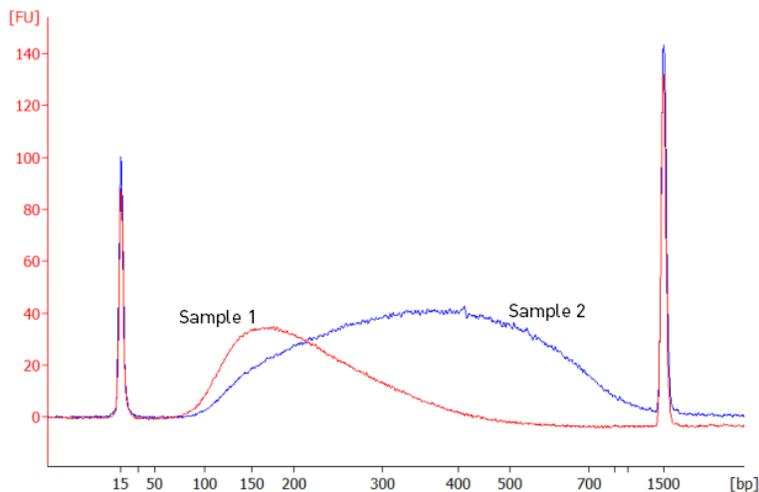
Panel B, Over-, and under-digestion profiles: Examples of over-digested (Sample 1, red) and under-digested (Sample 2, blue) gDNA fragments for a 200-base-read library. Either of these fragmentation profiles can be used for library construction. The expected library yield is greater than library yield from optimally fragmented DNA using either the Bioruptor™ or Covaris™ systems, due to the higher ligation efficiency of fragments generated with Ion Xpress™ Plus Fragment Library Kit.
