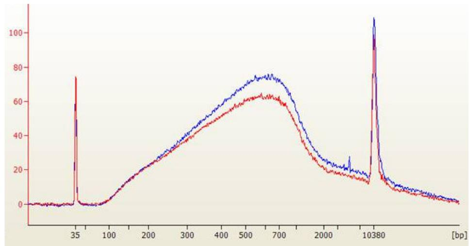
1 µg of human gDNA was fragmented with the Ion Xpress™ Plus Fragment Library Kit with a reaction time that was adjusted for 500-base-read libraries. Analysis was with the Agilent™ High Sensitivity DNA Kit. Peaks at 35 bp and 10,380 bp represent low- and high-molecular weight markers.
