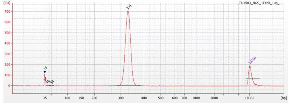
*E. coli* DH10B DNA was fragmented with the Bioruptor™ NGS System for 17 minutes.
