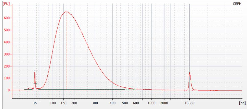
Panel B, Fragment profile of 1 µg of human gDNA CEPH Individual 1347-02 supplied in the Ion Proton™ Controls Kit (Cat. No. 4478328) for Ion Proton™ System sequencing.
