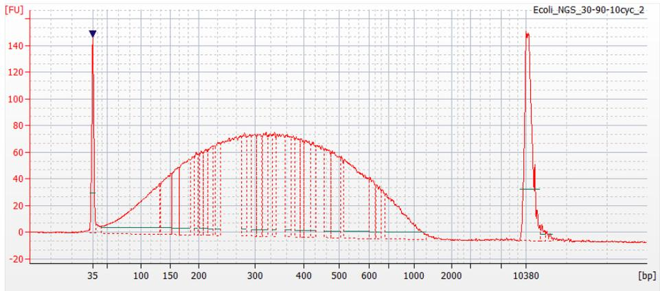
1 µg of *E. coli* DH10B DNA was fragmented with the Bioruptor™ NGS System for 20 minutes. Analysis was with the Agilent™ High Sensitivity DNA Kit. Peaks at 35 bp and 10380 bp represent low- and high-molecular weight markers.
