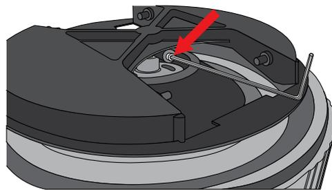
**Note:** A newer version of the rotor lacks a set screw. In this case, simply press the rotor firmly onto the motor shaft to install.
