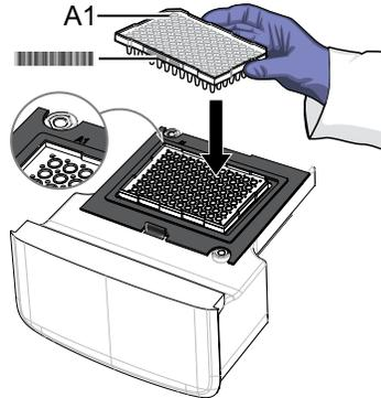
**IMPORTANT!** Plates should be loaded and unloaded by trained operators who have been warned of the moving parts hazard.
