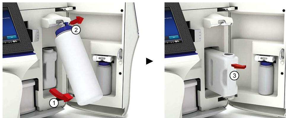
3. Reinstall the empty waste reservoir and the *used* Ion S5™ Wash Solution bottle.
