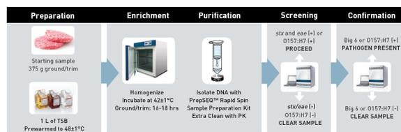
**Figure 1** RapidFinder™ *E. coli* STEC detection workflow (spin column method)
