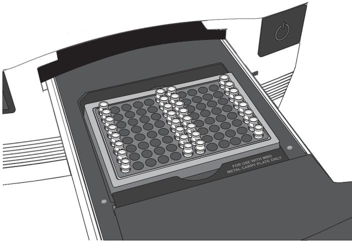
**Figure 4 7500 Fast instrument tube layout** RapidFinder™ Express Software directs the user to load empty strip tubes in column 1 (far left) and column 12 (far right), if needed. The empty capped 8-tube strips evenly distribute the clamping load applied to the sample tube strips during processing, thereby minimizing the risk of collapsing any tubes.
