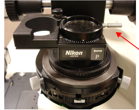
Figure 34 DIC polarizer in position.
