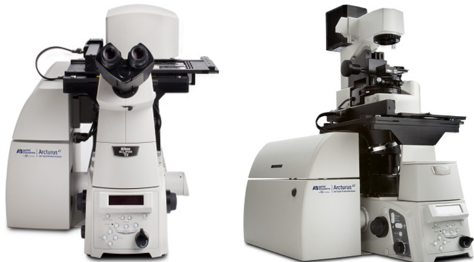
Figure 60 Arcturus XT Instrument with LED tower and with Nikon TM tower.
