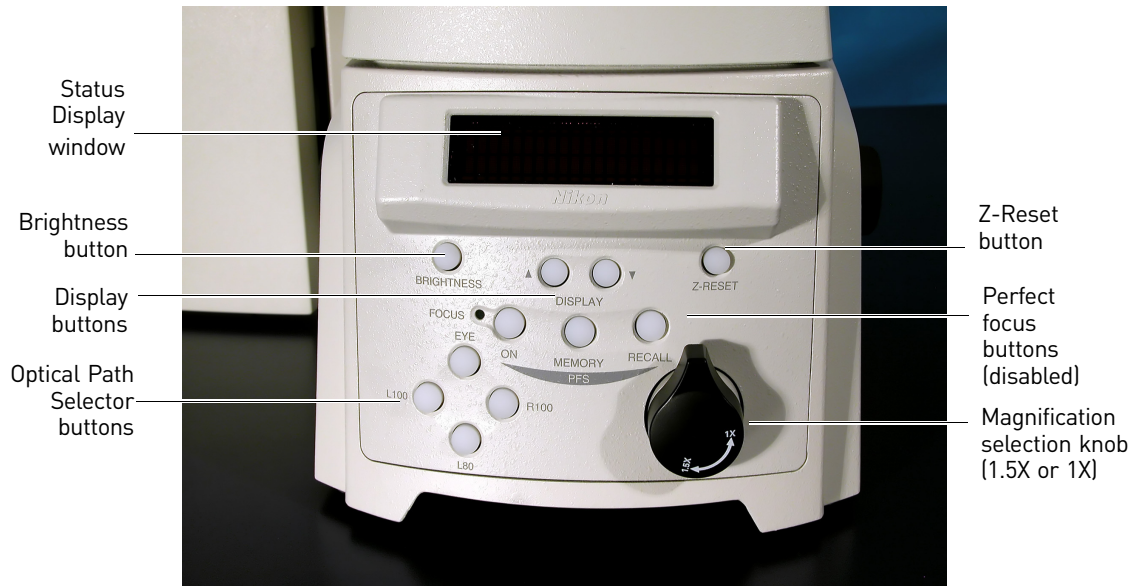
Figure 12 Nikon™ Eclipse™ Ti-E front operation panel.
