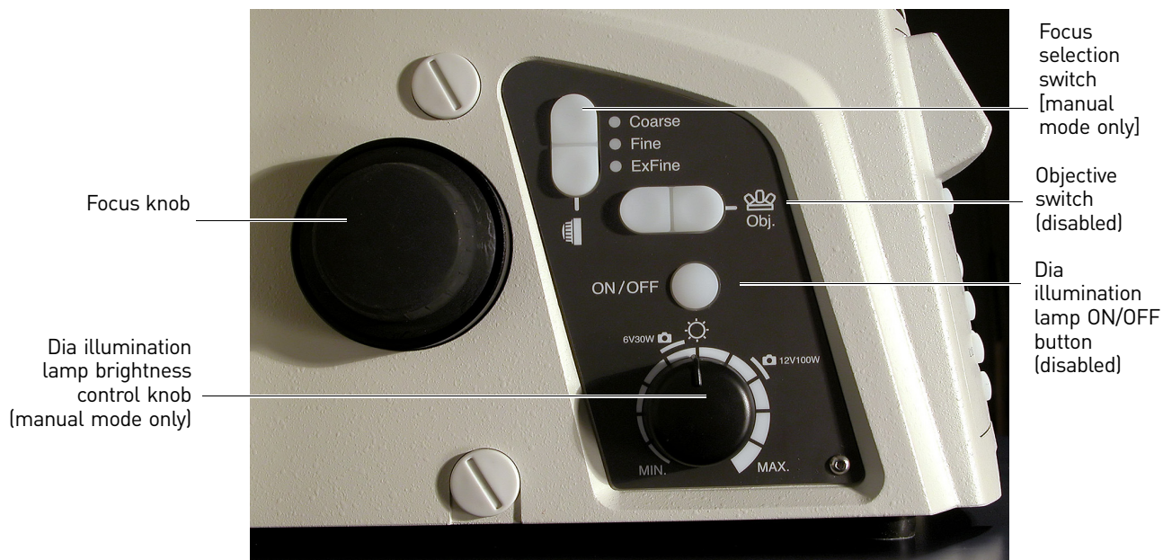
Figure 13 Nikon Eclipse Ti-E left operation panel.
