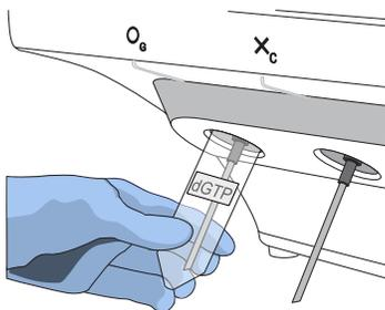
**Note:** The instrument checks the pressure of the Reagent Bottles and Wash Bottles. If a bottle leaks, check that it is tightly attached to the instrument. If it continues to leak, replace it. If the instrument still does not pass the leak check, contact Technical Support.
