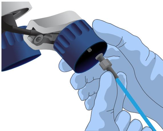
5. Immediately attach the prepared Wash 2 Bottle in the W2 position, then tighten the cap. Press **Next**.
