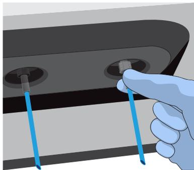
3. Attach each prepared Reagent Bottle to the correct dNTP port (e.g., the dGTP tube on the port marked "G") and tighten firmly by hand until snug. Press **Next**.
