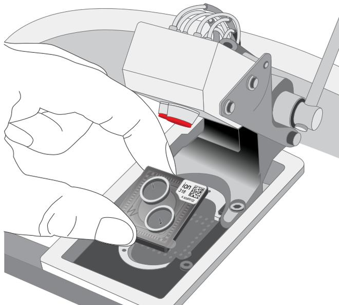
7. Press **Chip Check**. During the initial part of Chip Check, visually inspect the chip in the clamp for leaks.
