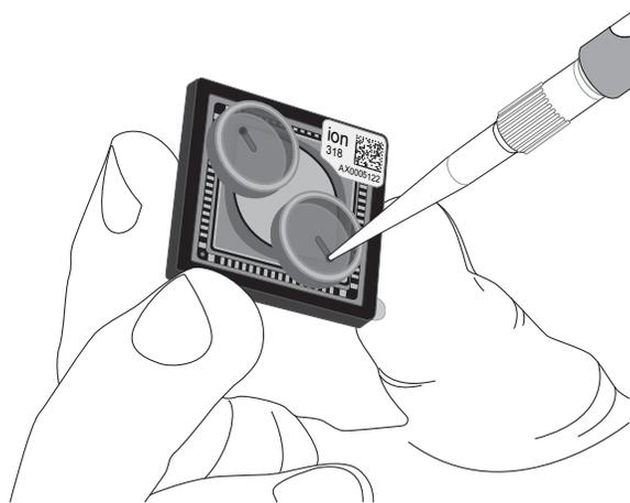
3. Insert the pipette tip firmly into the loading port, then remove as much liquid as possible from the loading port. Discard the liquid.
