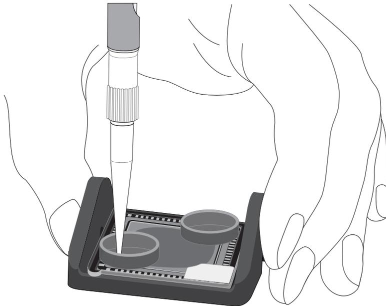
3. With the pipette unlocked, apply gentle pressure between the tip and chip and slowly dial down the pipette (~1  $\mu\text{L}$  per second) to deposit the ISPs. To avoid introducing bubbles into the chip, leave a small amount in the pipette tip (~0.5  $\mu\text{L}$ ).
