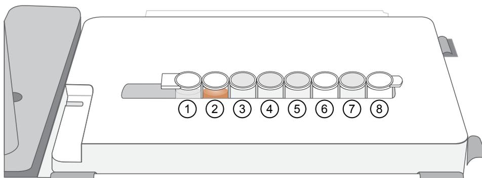
4. Ensure that the square-shaped tab is on the left, then insert the filled 8-well strip with the 8-well strip pushed all the way to the right end of the slot of the Tray.
