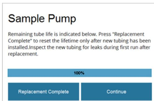
**IMPORTANT!** Inspect the new tubing for leaks during the first run after replacement.
