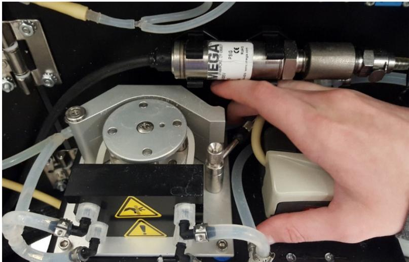
7. Swing the locking lever counterclockwise and engage it with the slot in the clamping bracket to secure the sheath pump tubing within the pump roller assembly.
