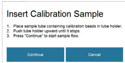
8. Push the tube holder upward until it stops, then press **Continue** to start the sample flow.
