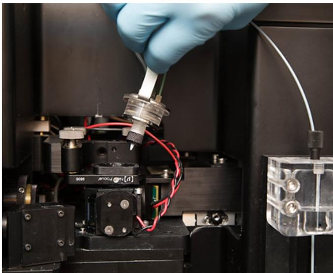
2. Unscrew the small black cap that secures the nozzle tip to the nozzle assembly using the torque wrench provided with the instrument.
