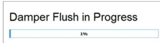
19. At the completion of the first and second damper flush cycles, the instrument prompts you to place a new sample tube containing 3 mL of sheath fluid in the sample tube holder in the up position.
