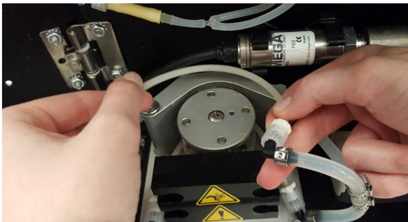
8. After you have removed both sheath pump tubes from the pump roller assembly, twist and pull apart the fittings to disconnect the sheath pump tubes from the fluid lines (clear lines). Discard the used sheath pump tubing.
