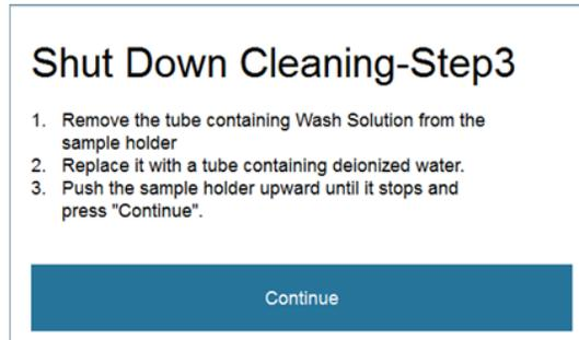
8. Move the sample tube holder up until it stops, then press **Continue** to initiate the Shut Down Cleaning – Step 3.
