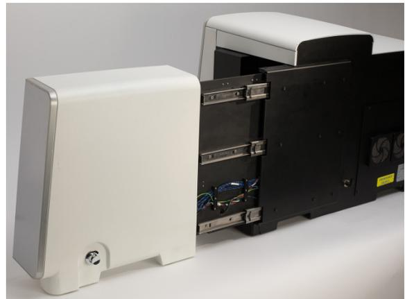
Rear view with fluidics compartment door fully open
