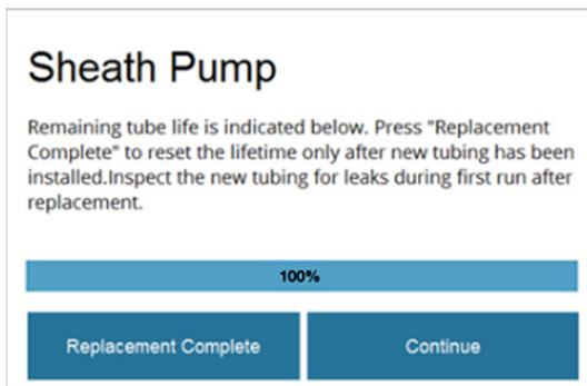
11. After replacing the sheath pump and sheath tubing, sheath fluid must flow for 20 minutes to calibrate the new tubing. When prompted, prompted, press **Continue** to start the flow.
