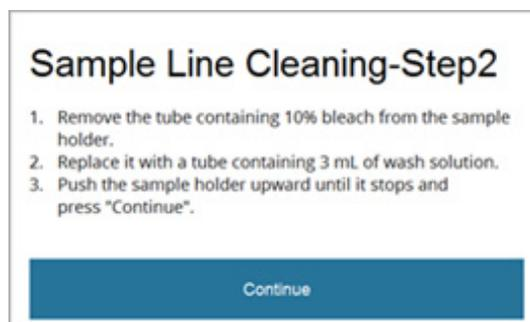
6. Move the sample tube holder up until it stops, then press **Continue** to initiate the second step of the cleaning process.
