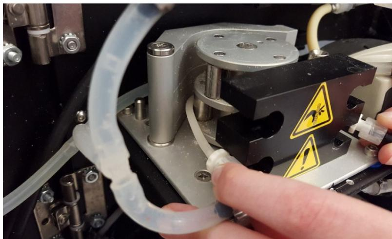
3. Insert the fittings into the bottom slots in the pump assembly to secure them.
