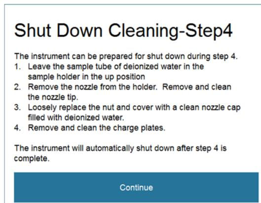
10. Leave the sample tube of deionized water in the sample tube holder in the up position, then press **Continue** to initiate the Shut Down Cleaning – Step 4.
