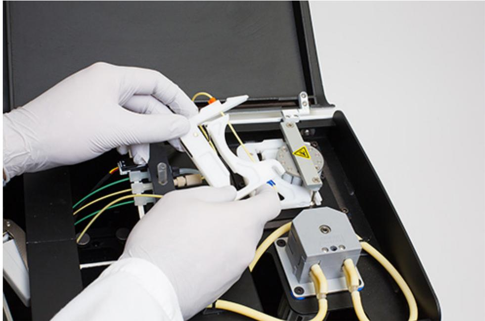
3. Remove the tubing from the shoe by pulling on the blue and orange stoppers attached to the tubing line and moving the line away from the shoe.
