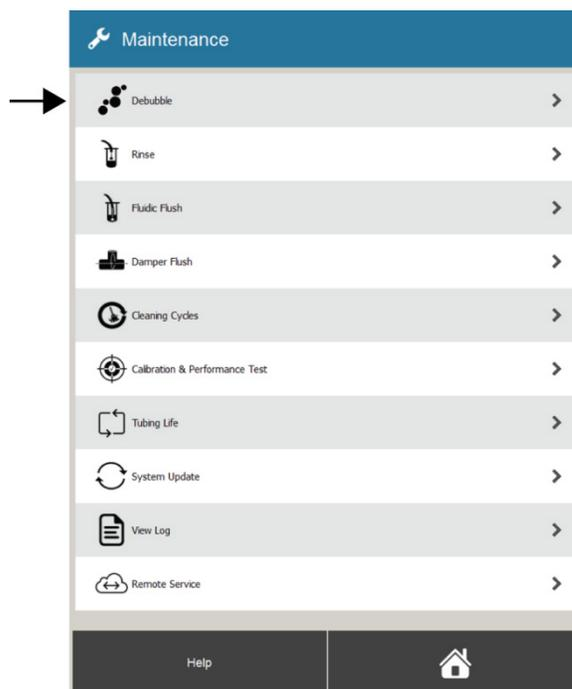
The instrument performs the Debubble procedure automatically, which takes approximately 2 minutes to complete.
