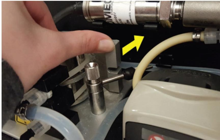
6. Gently pull the fittings that connect the tubing to the sheath fluid lines towards you, then out to the side until all four fittings are freed from the pump assembly.
