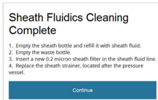
23. To complete the sheath fluidics cleaning procedure, replace the 0.2- $\mu$ m sheath inlet filter in the sheath fluid line with a new filter (see page 117), then press **Continue** to return to the Cleaning cycles menu.
