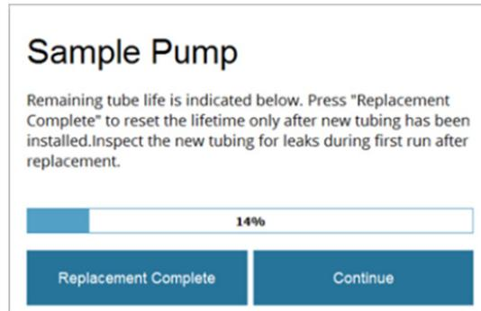
2. Click **Replacement Complete** to reset the tubing life counter to 100% and return to the Tubing Life screen.
