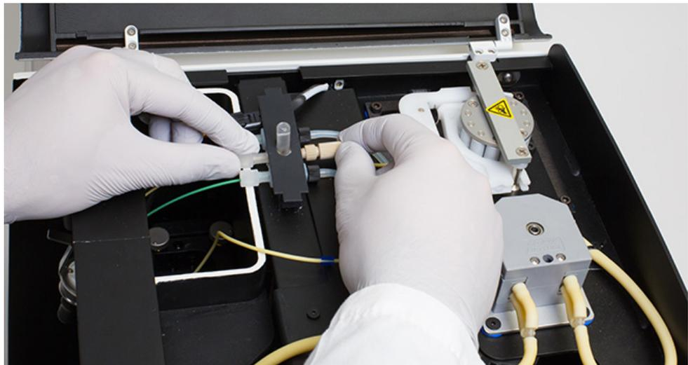
5. Remove the bracket that secures the sample tube dampener and the fluidic lines to the instrument.
