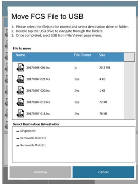
3. Double-tap the USB drive that appears on **Destination Drive/Folder** list to navigate through its folders and select the desired destination folder.
