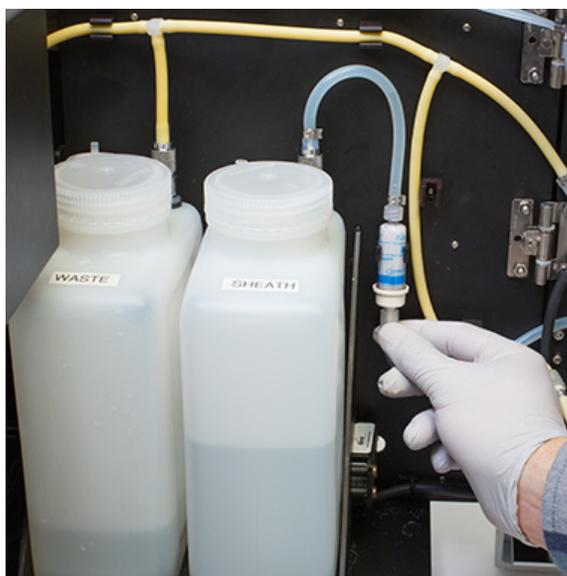
2. Remove the sheath inlet filter from the sheath line by disconnecting the Luer fittings on each end.
