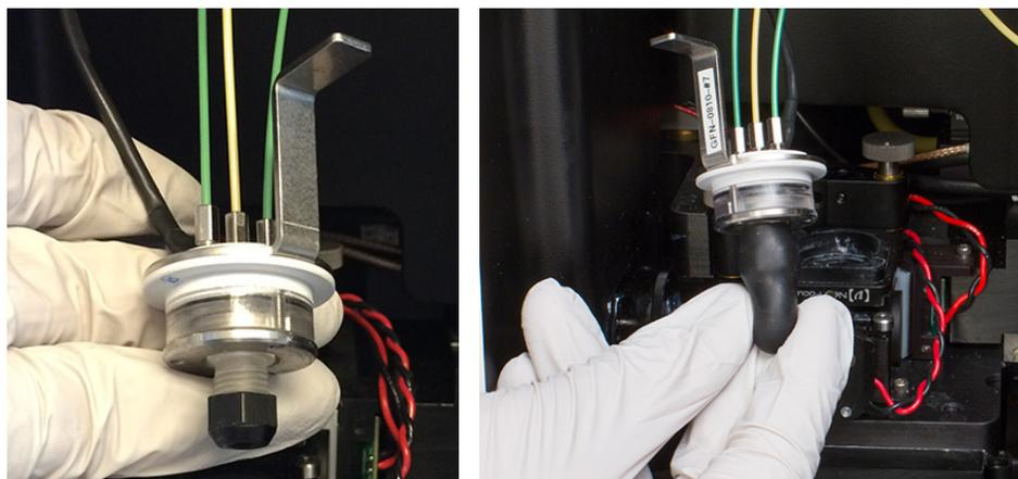
7. If you have removed the nozzle tip after performing the Shut Down operation (page 88), store the nozzle tip in the detergent solution at room temperature until the next time you need to use the instrument.
