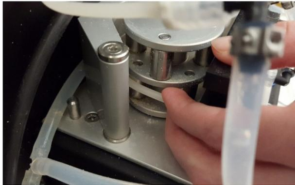
5. Repeat the process for the top set of the sheath pump tubing, gently sliding it into position and centering it within the top rollers.
