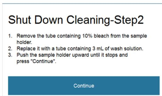
6. Move the sample tube holder up until it stops, then press **Continue** to initiate the Shut Down Cleaning – Step 2.
