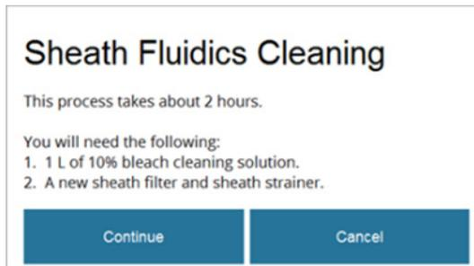
The instrument will pressurize the fluidics system and initiate the sheath fluidics cleaning.
