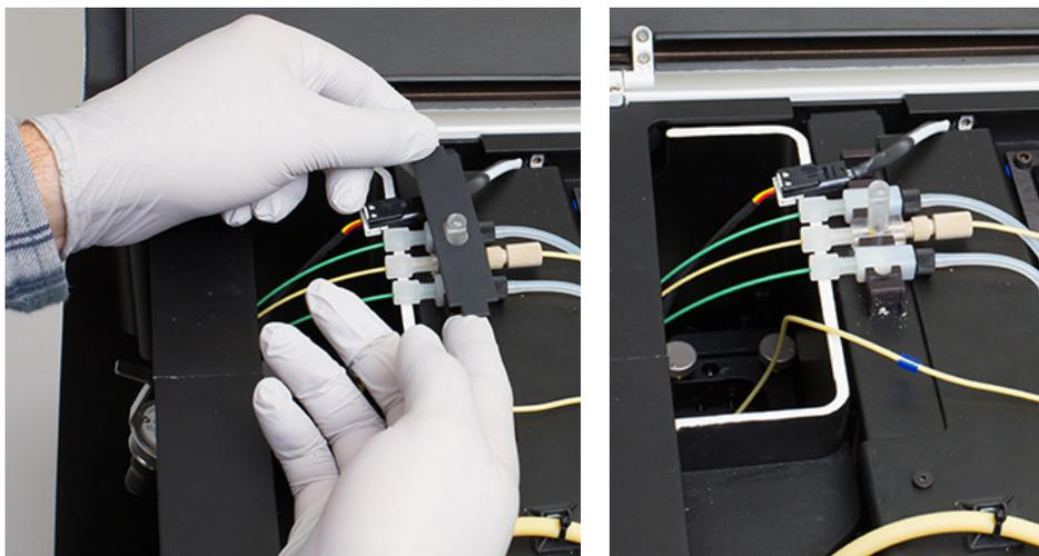
6. Unscrew the sample pump dampener and detach from the instrument.
