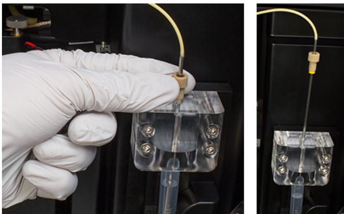
8. Remove the dampener and the sample pump tubing from the instrument.
