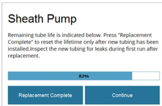
10. In the Sheath Pump Life dialog, press **Replacement Complete** to reset the sheath pump tube life counter to 100%.
