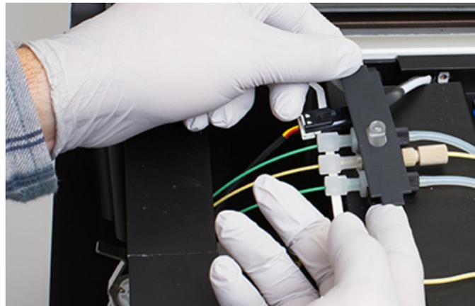
3. Insert the sample line through the screw and the clear Lucite block that secures the sample injection port to the instrument. When the sample line is positioned correctly, tighten the screw.
