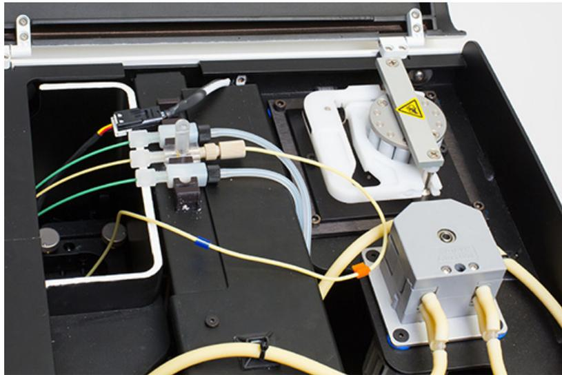
2. Make sure that the sample pulse dampener is upright, then attach the bracket that secures the sample tube dampener and the fluidic lines to the instrument.
