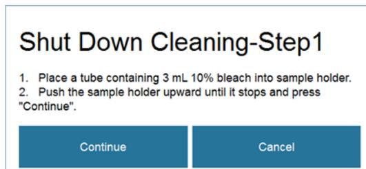
4. Move the sample tube holder up until it stops, then press **Continue** to start the Shut Down Cleaning – Step 1.
