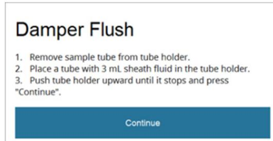
20. After the completion of the third damper flush, the instrument prompts you to perform a rinse. When prompted, remove the sample tube containing the sheath fluid and replace it with an empty sample tube.
