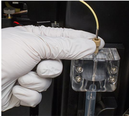
4. Insert the sample pump tubing into the shoe, making sure that the tubing remains slack.
