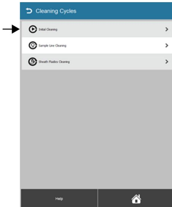
However, if the instrument remains idle for more than 30 minutes, you will be prompted to perform the initial cleaning again to prepare the sample line for further runs.
