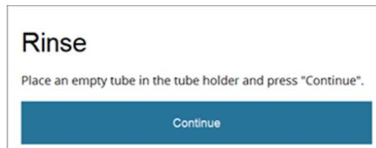
21. With the sample tube holder in the down position, press **Continue** to initiate the final rinse. At the completion of the rinse, the instrument drains the fluidics lines and internal reservoirs into the waste container.
