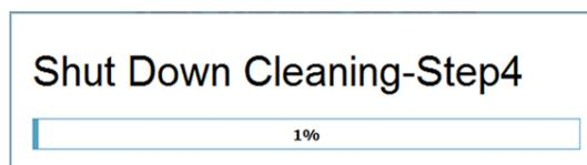
11. After completing the Shut Down Cleaning – Step 4, the instrument turns off the fluid stream, the deflection plates, and the laser, then powers itself off.
