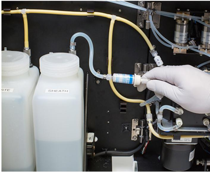
3. Attach the replacement 0.2- $\mu\text{m}$  sheath inlet filter (Cat. No. A33307) by connecting the Luer fittings to the sheath lines on each end.
