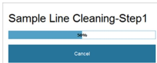
5. When prompted, remove the tube containing the 10% bleach solution from the sample tube holder, and replace it with a tube containing Attune™ Wash Solution.
