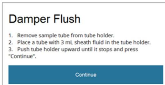
6. Move the sample tube holder up until it stops, then press **Continue** to begin the damper flush.
