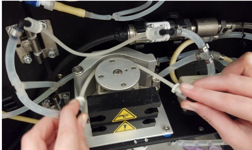
2. Gently slide the bottom set of the sheath pump tubing into position between the pump rollers and the clamping bracket.
