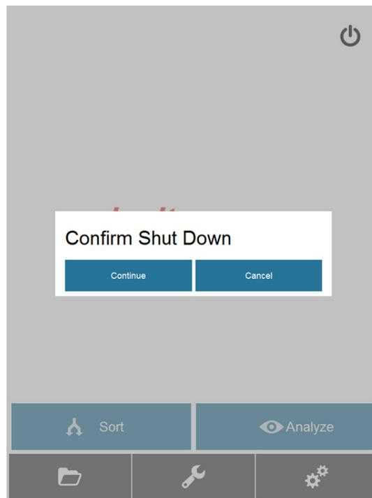
2. Press **Continue** to confirm the Shut Down. The instrument initiates the Shut Down procedure.
