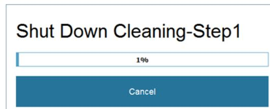
5. When prompted, remove the tube containing the 10% bleach solution from the sample tube holder, and replace with a tube containing Attune™ Wash Solution.
