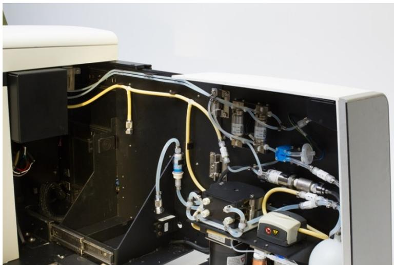
3. Unscrew the lid and fill the sheath fluid container with the appropriate solution. The sheath fluid container has 2 L capacity, sufficient to process 5 mL of sample. Do not overfill past the 2 L line on the bottle.
