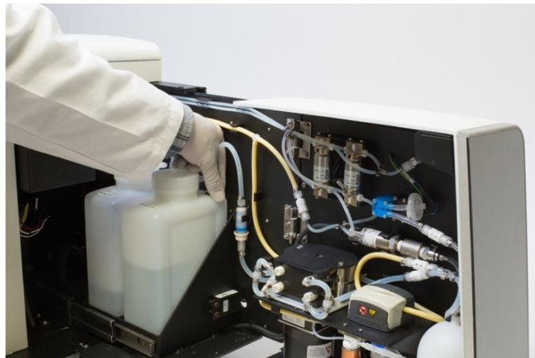
2. After detaching the fluid lines from the containers, slightly lift and pull out the containers from the fluidics compartment.
