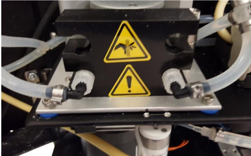
4. Align the sheath pump tubing to the center of bottom rollers, keeping it away from the edges where it could possibly get pinched or caught in a gap.
