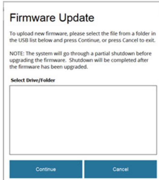
3. Select the latest iSort™ firmware file from the USB list on the Firmware Update screen, then click **Continue**. The system will go through a partial Shut Down before upgrading the firmware automatically. When the firmware is upgraded, the instrument will complete the Shut Down operation.
