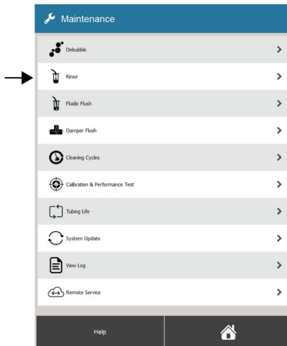
2. Replace the sample tube in the sample tube holder with an empty tube, then press **Continue**. The instrument performs the rinse automatically, which takes approximately 30 seconds to complete.
