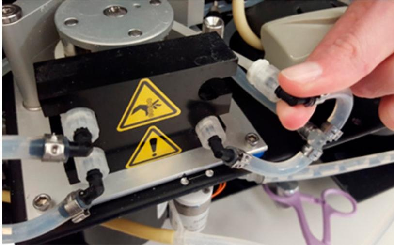
7. Gently lift the sheath pump tubing and remove it from the pump roller assembly.
