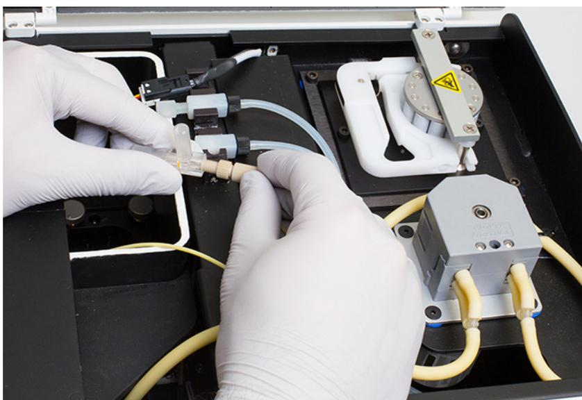
7. Unscrew the screw above the Lucite block that secures the sample line to the instrument.
