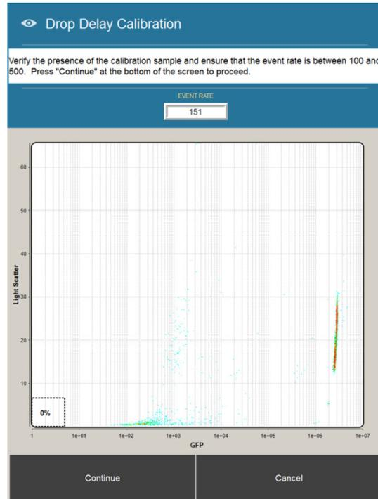
12. Ensure that the event rate counter located above the scatter plot registers an event rate of between 100 and 500, then press **Continue**.
