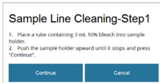
4. Move the sample tube holder up until it stops, then press **Continue** to initiate the first step of the cleaning process.
