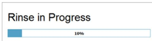
5. When prompted, remove the empty sample tube from the sample tube holder and replace it with a tube containing 3 mL of sheath fluid.
