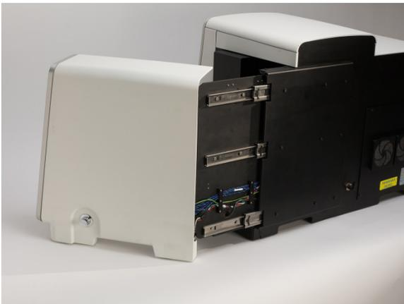
Rear view with fluidics compartment door partially open
