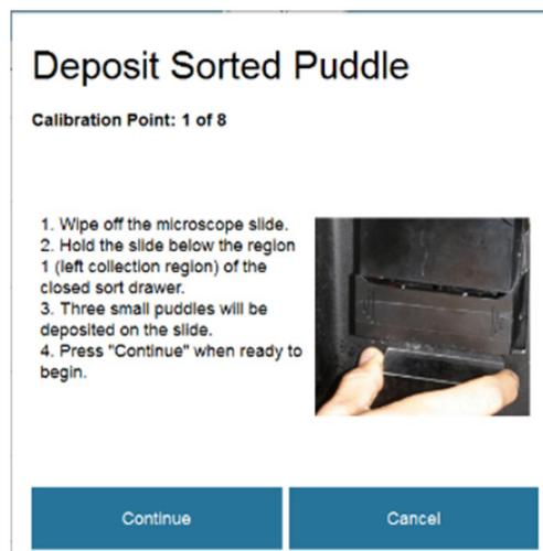
14. When prompted, examine the puddles deposited on the slide under a fluorescent microscope for the first calibration point:
