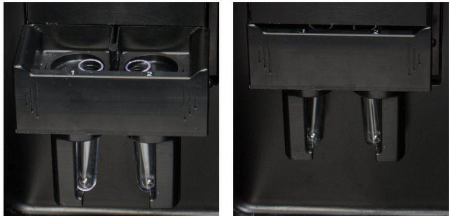
2. Close the sorting compartment door to minimize interfering light and exposure to aerosols, then press **Continue**.
