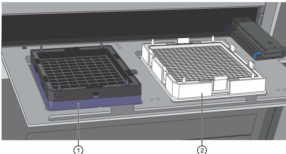
**Figure 43** Array plate with blue protective base and the hybridization tray aligned properly loaded into drawer 6.
