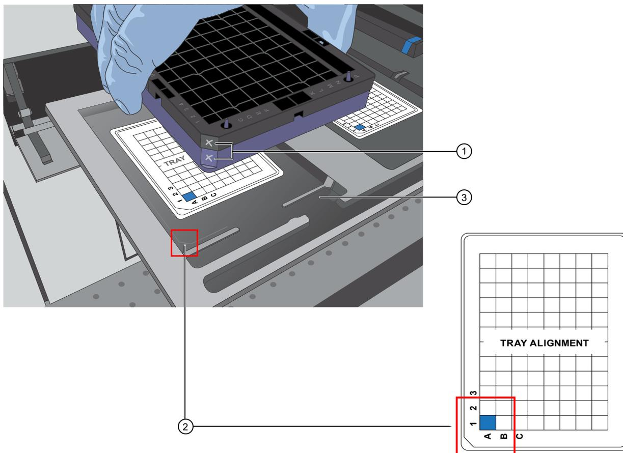
**Figure 42 Notched corners marked and aligned with tray alignment guide.**
