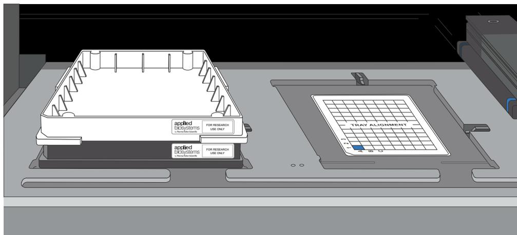
Figure 37 Drawer 2: Scan tray with cover on left side.
