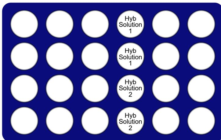
**Figure 20 Placement of reagents on chilled reagent block for the resuspension and hybridization preparation step.**
