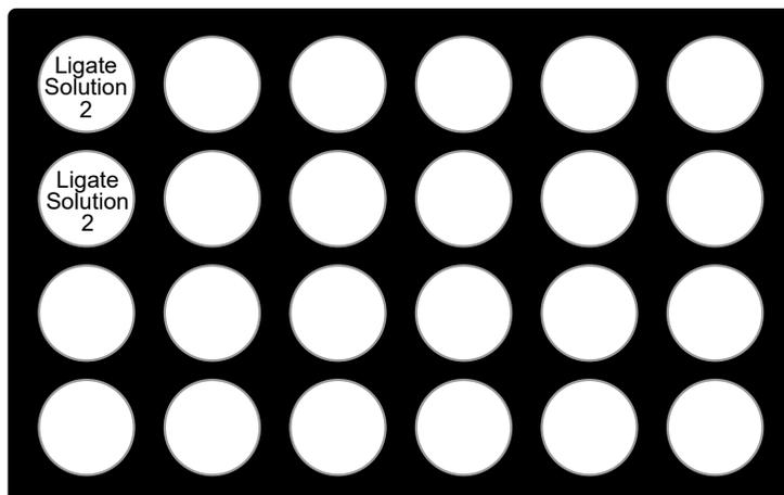
Figure 28 Placement on reagents on 24-position tube rack for GeneTitan™ reagent preparation.
