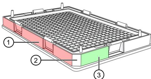
Figure 49 Correct area to label a GeneTitan™ 384 Layout Hybridization Tray.
