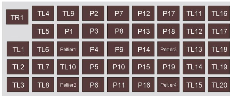
Figure 13 Deck positions on the Biomek™ i7 Automated Workstation.
