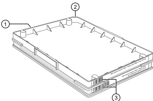
**Figure 44** Example shows consumables that must be rotated and loaded on the drawer so that the barcodes face into the instrument.
