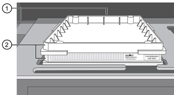
**Figure 45** Example of properly loaded GeneTitan™ tray consumables. A GeneTitan™ stain tray and the stain tray cover are shown in this example.
