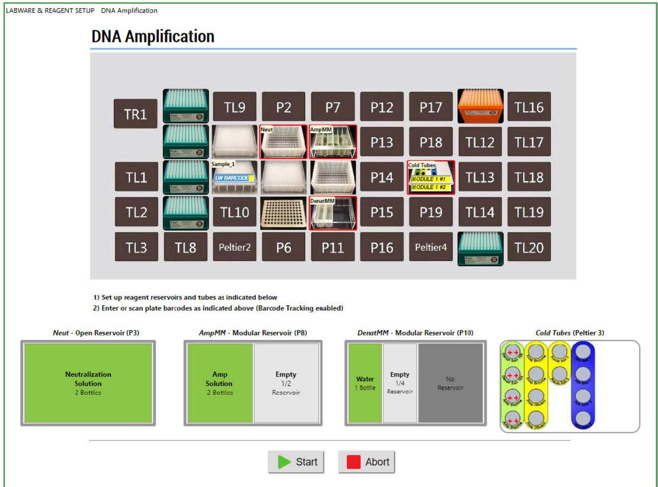
Figure 12 DNA amplification step deck layout.
