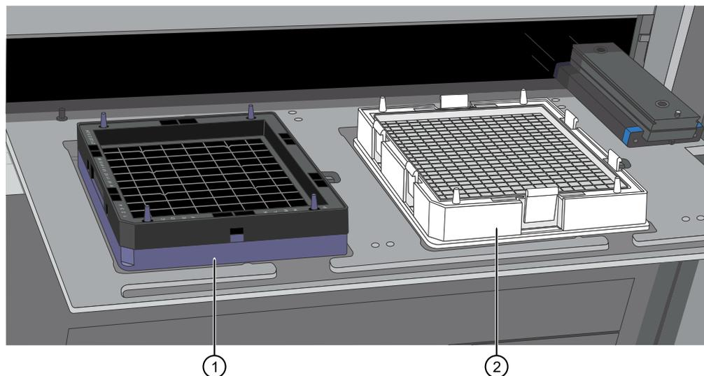
Figure 32 Array plate on protective blue base and the hybridization tray properly loaded into drawer 6.
