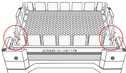
Figure 6 Thermoshake 384 Deepwell Plate Adapter orientation on the Biomek™ i7 deck.
