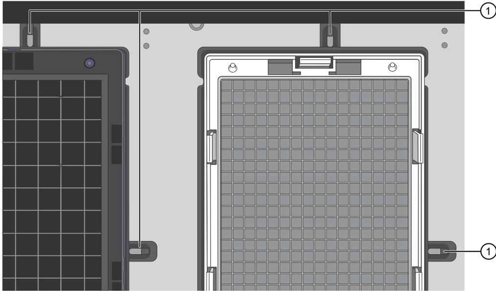
Figure 47 Place trays on the drawer when the tabs, or fingers, are retracted.
