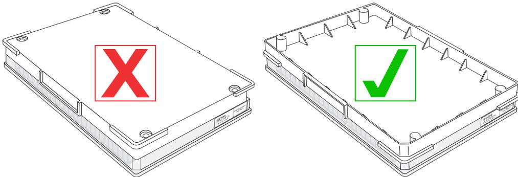
Figure 48 Placement of covers on trays.
