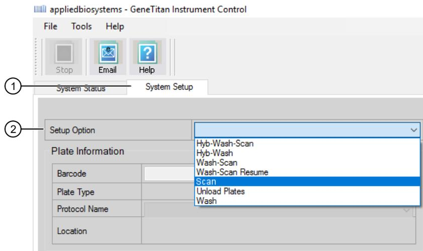
Figure 36 Scan setup option to process a second array plate.
