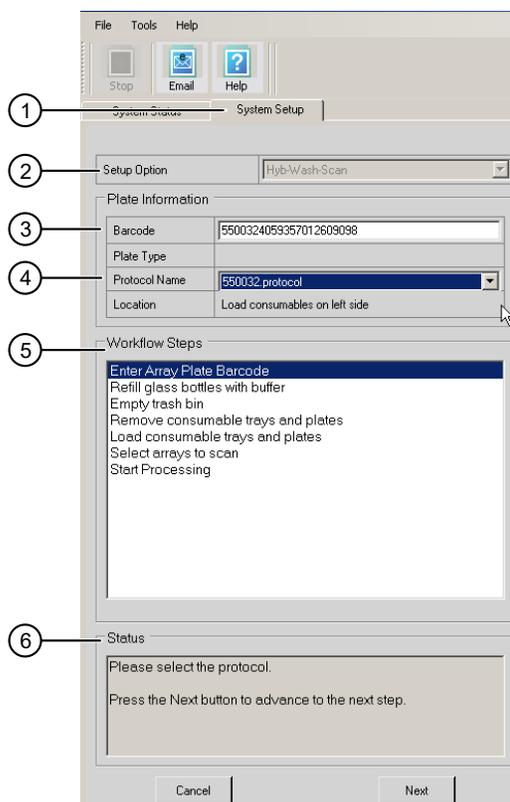
Figure 30 System Setup tab
