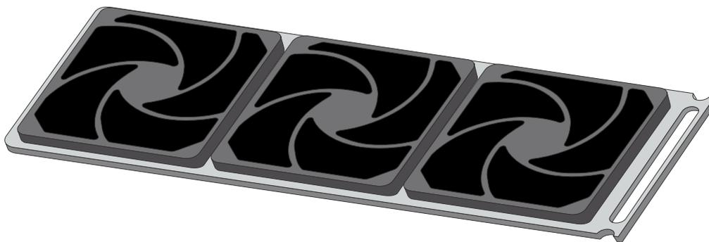
Figure 55 GeneTitan™ fan filter cartridge.
