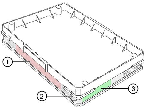
Figure 50 Correct area to label a GeneTitan™ 384 Layout Reagent Tray.
