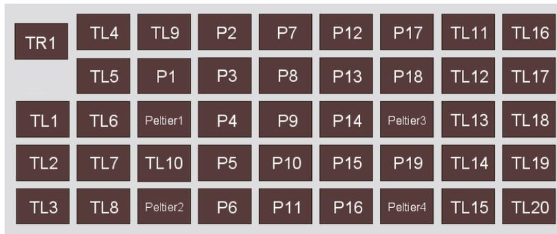
Figure 16 Deck positions on the Biomek™ i7 Automated Workstation.
