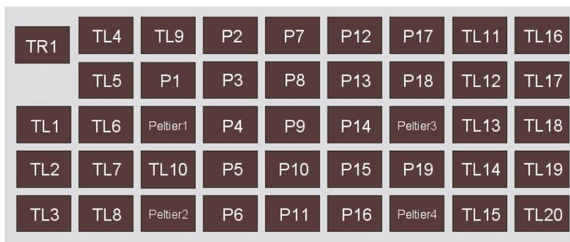
Figure 26 Deck positions on the Biomek™ i7 Automated Workstation.
