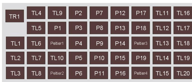
Figure 22 Deck positions on the Biomek™ i7 Automated Workstation
