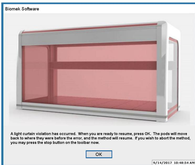
Figure 4 A message window is displayed when the light curtain has been penetrated.
