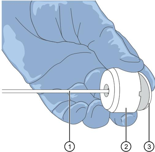
**Figure 56** Components of the reagent buffer supply line and filter.
