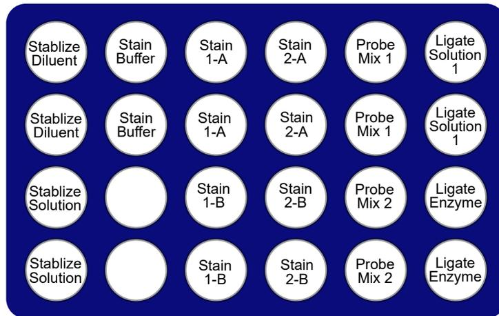
**Figure 27 Reagent cold block for GeneTitan™ reagent preparation.**
