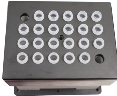
Figure 8 Hole alignment between the tube adapter and cover.
