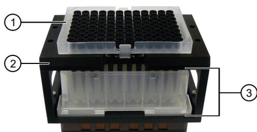
**Figure 8** Tip isolator setup.
