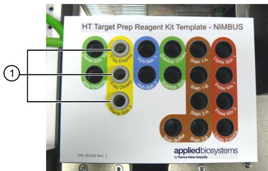
1. Three fragmentation reagent tubes that are inserted into tube block.
