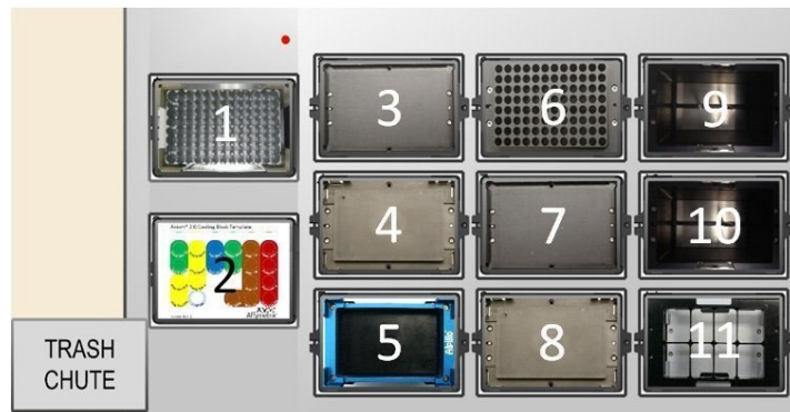
Figure 2 NIMBUS™ Instrument deck configuration for the Automated HT Target Preparation Solution method.
