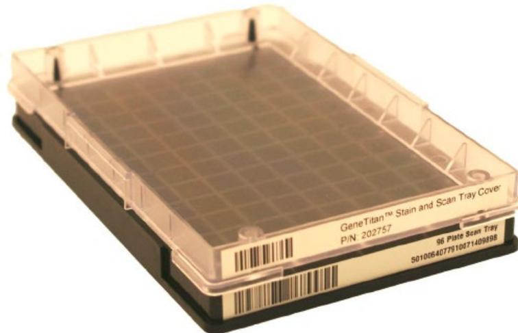
Figure 1.8 Stain Tray with Cover. Deionize the cover and the tray.
