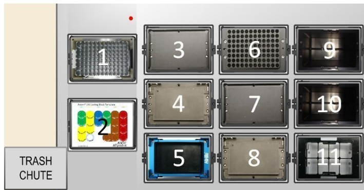
Figure 1 NIMBUS™ Instrument deck configuration for the Axiom™ 96 Sample Automated Target Preparation Solution method.
