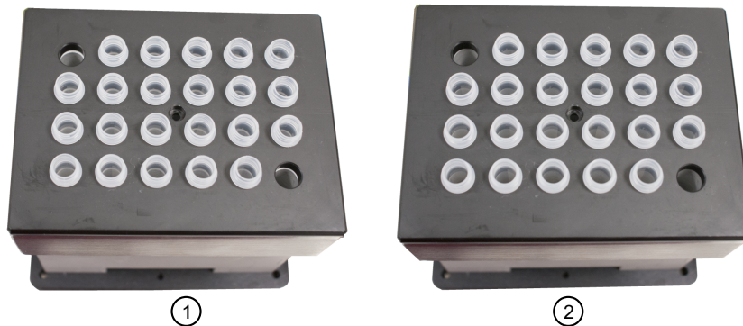
Figure 8 Hole alignment between the tube adapter and cover.
