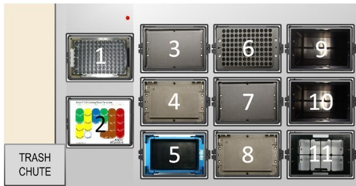
Figure 2 NIMBUS™ Instrument deck configuration for the Axiom™ 96 Sample Automated Target Preparation Solution method.
