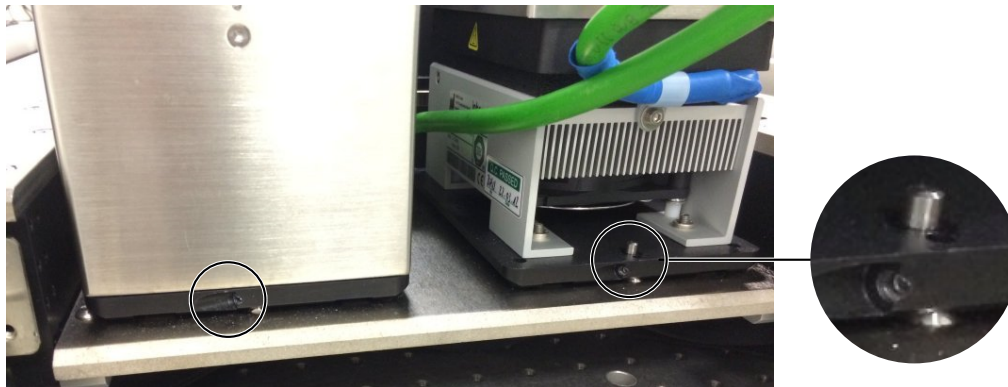
Figure 4 Each device has only 1 set screw.
