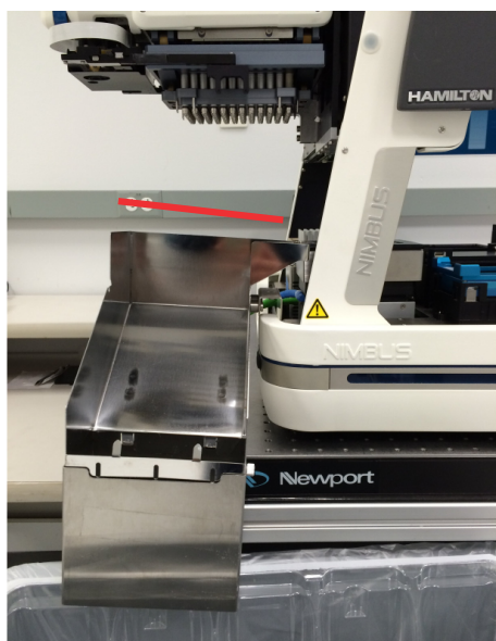
① Example of a trash chute that is not level.
