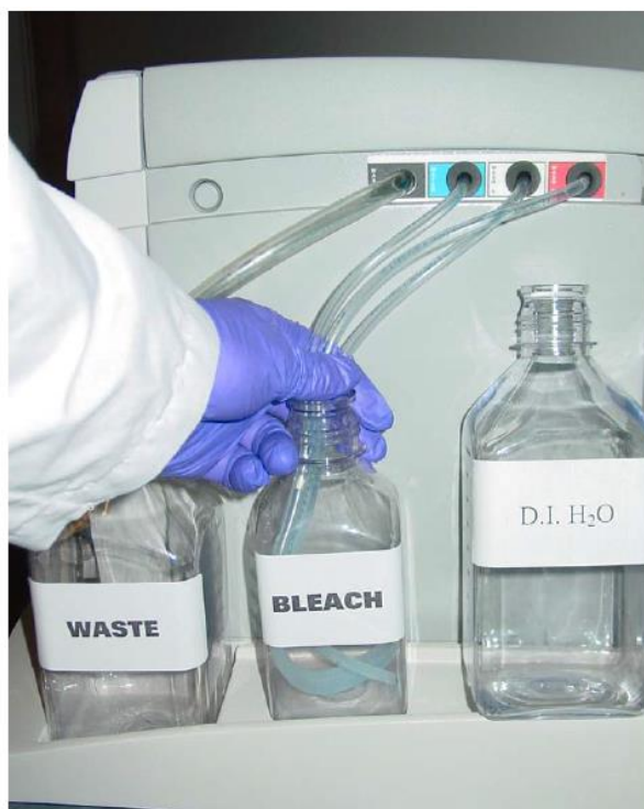
Figure 9.2 The bleach cycle. Immerse the tubes into the 0.525% sodium hypochlorite solution. The waste line remains in the waste bottle
