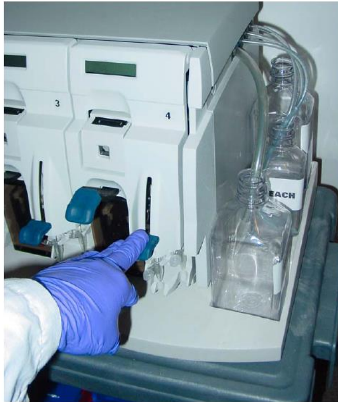
Figure 9.4 Press down on the needle levers to start the bleach protocol
