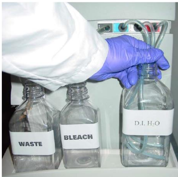
Figure 9.5 Immerse the three wash and water lines in the DI water bottle
