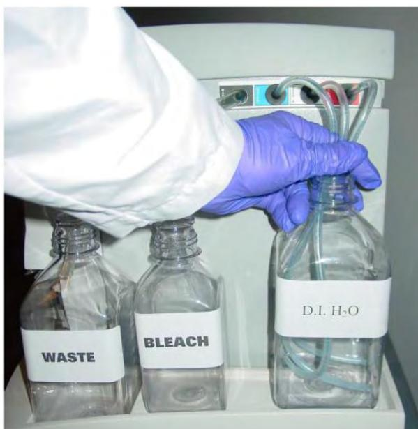
3. Press down on the needle levers to begin the rinse cycle. The fluidics station will empty the lines and rinse the needles.
