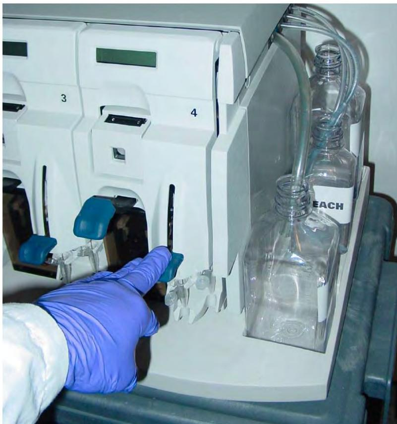
10. The fluidics station will begin the protocol and begin to empty the lines and perform the cleaning cycles using bleach solution.
