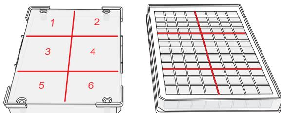
**Figure 56** Deionization zones for GeneTitan™ 96-format trays and covers.
