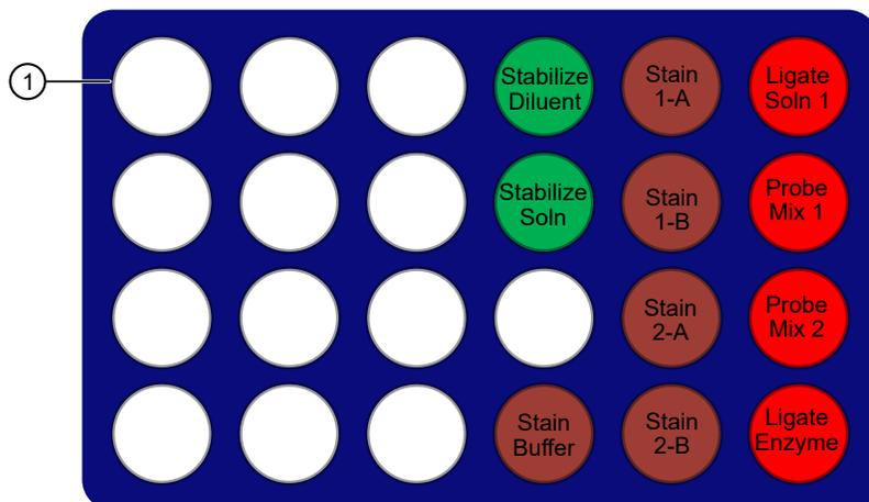
Figure 19 Placement of reagents in cooling block for GeneTitan reagent trays preparation—part 1. Diagram of the cooling block without the reagent template.
