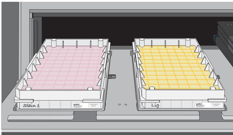
Figure 31 Drawer 3, left side: Stain 1 tray with cover. Drawer 3, right side: Ligation tray with cover.
