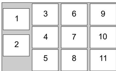
Figure 17 NIMBUS® Instrument deck positions.
