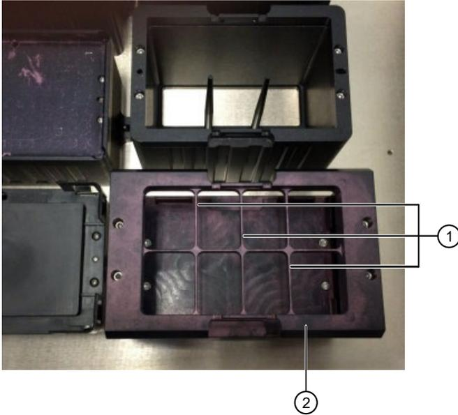
Figure 63 Tip Isolator on NIMBUS® Target Preparation Instrument deck.
