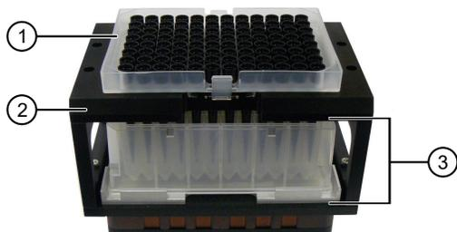
Figure 11 Tip isolator setup.
