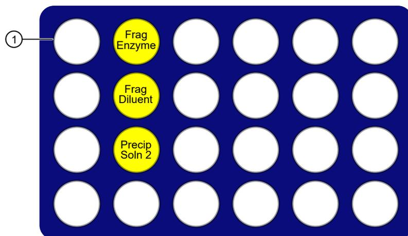
Figure 12 Placement of reagents in cooling block for fragmentation. Diagram of the cooling block without the reagent template.
