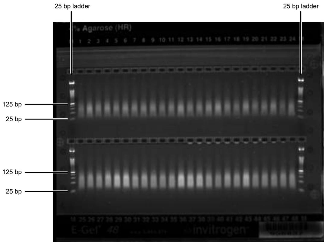
Figure 58 Fragments fall between 125 bp and 25 bp on a successful gel image.
