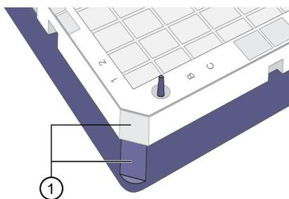
Figure 43 Notched corners aligned.
