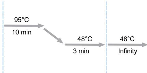
Figure 6 Axiom 2.0 Plus Denature thermal cycler protocol (Stage 5).
