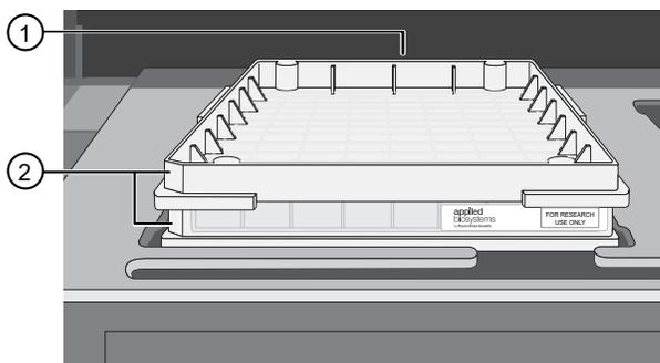
**Figure 48** Example of properly loaded GeneTitan™ tray consumables. A GeneTitan™ stain tray and the stain tray cover are shown in this example.
