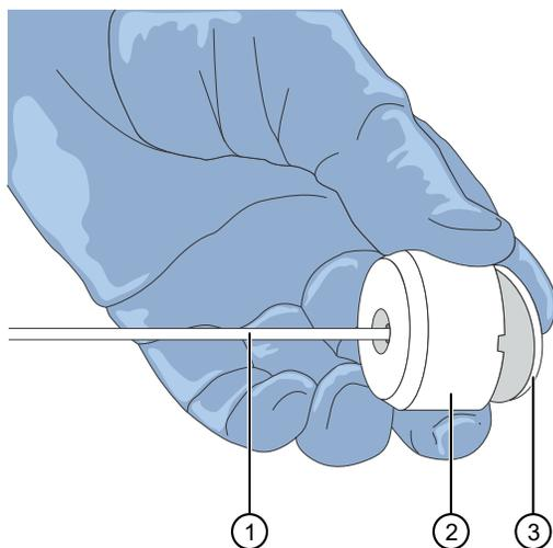
Figure 61 Components of the reagent buffer supply line and filter.
