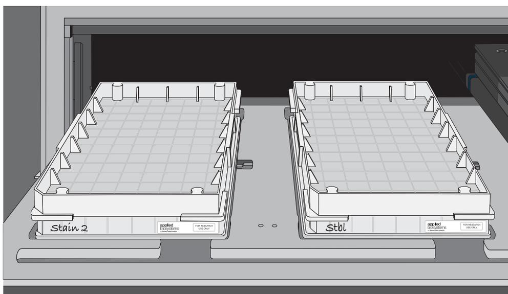
Figure 32 Drawer 4, left side: Stain 2 Tray with cover. Drawer 4 right side: Stabilization Tray.
