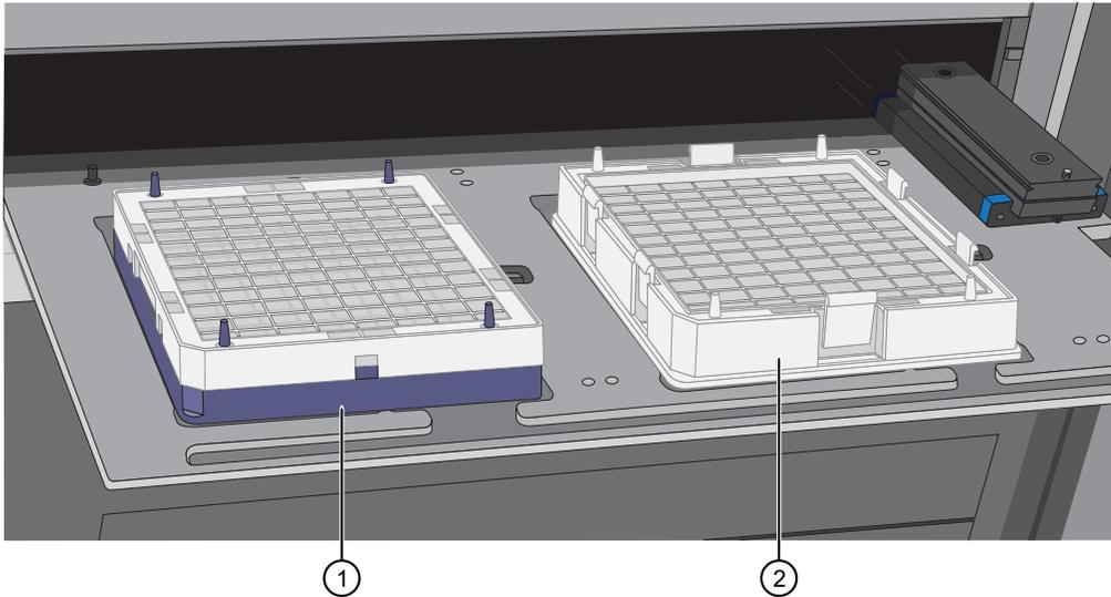
Figure 45 Array plate with protective blue base and the hybridization tray aligned properly loaded into drawer 6.
