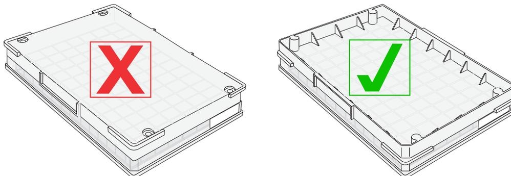
Figure 51 Placement of covers on trays.
