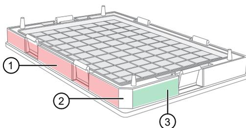
Figure 52 Correct area to label the GeneTitan™ 96-layout hybridization tray.
