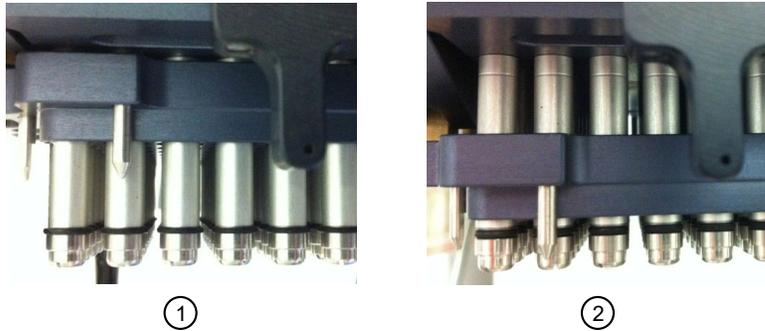
**Figure 62** O-rings shown in a squeezed and relaxed state.
