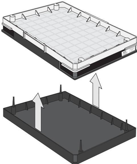
Figure 46 Remove the scan tray and cover from the base before loading in the GeneTitan™ Instrument.
