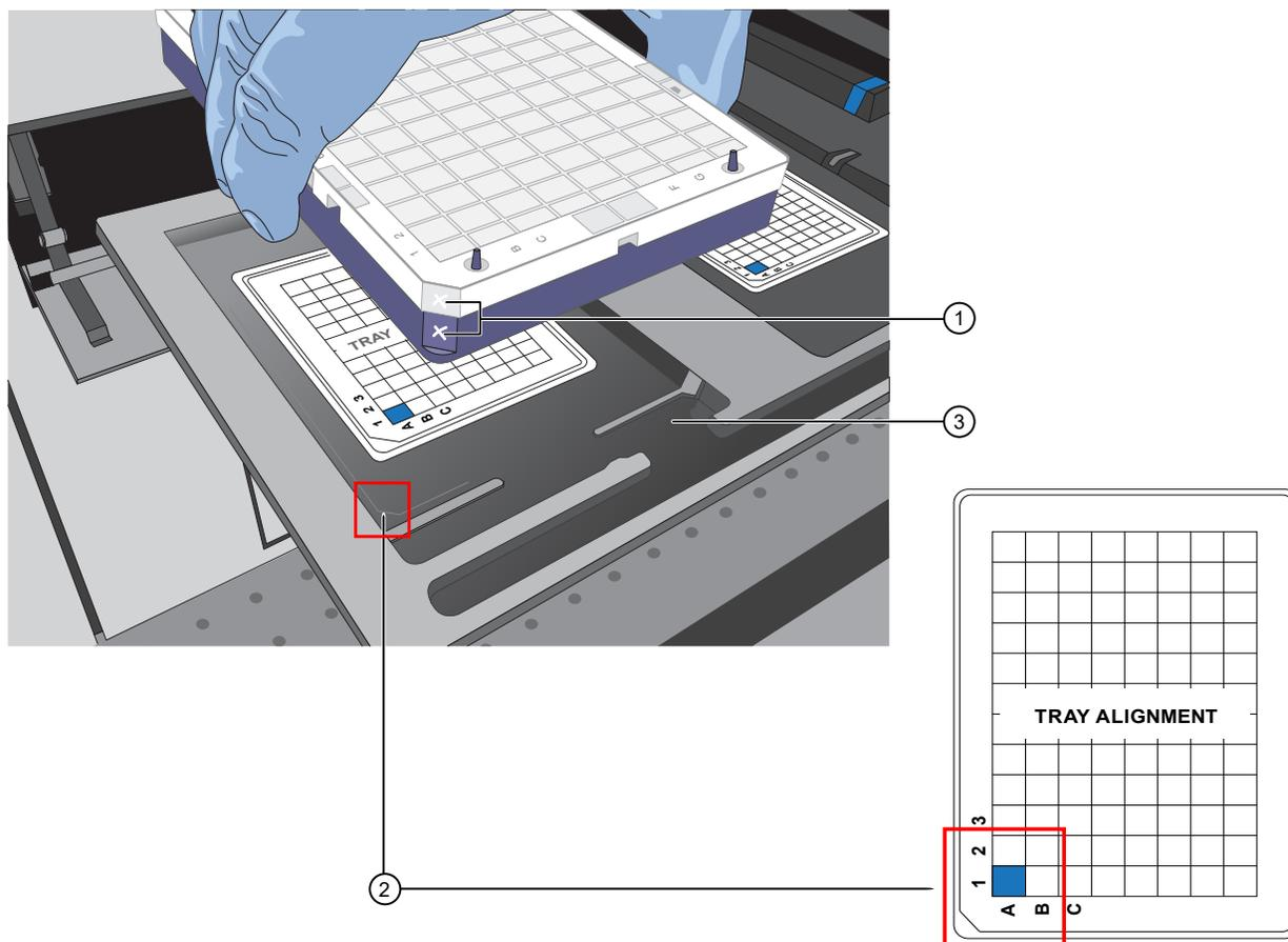
**Figure 44** Notched corners marked and aligned with tray alignment guide.
