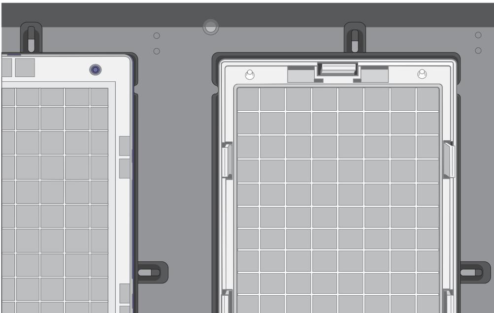
Figure 50 Trays are placed on the drawer when the tabs, or fingers, are retracted.
