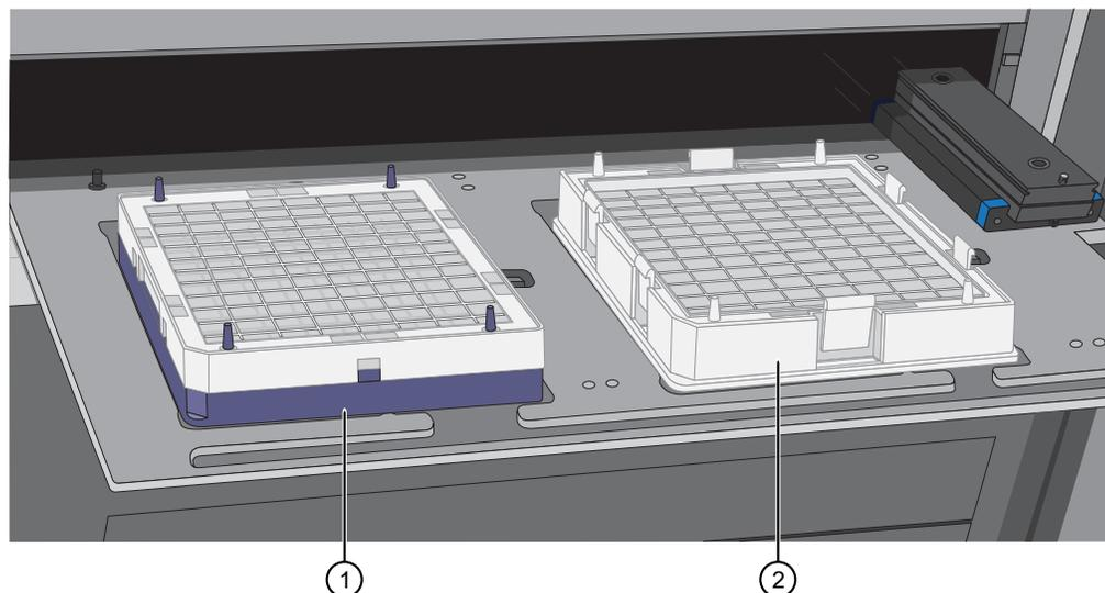
Figure 25 Array plate on protective blue base and the hybridization tray properly loaded into drawer 6.
