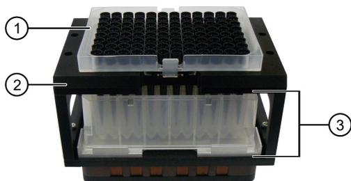
**Figure 8** Tip isolator setup.
