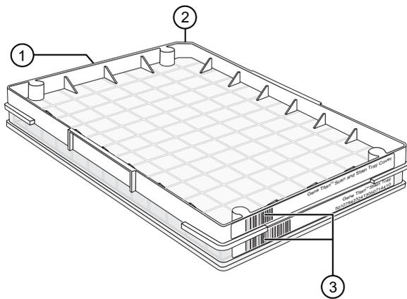
**Figure 47** Example shows consumables that must be rotated and loaded on the drawer so that the barcodes face into the instrument.
