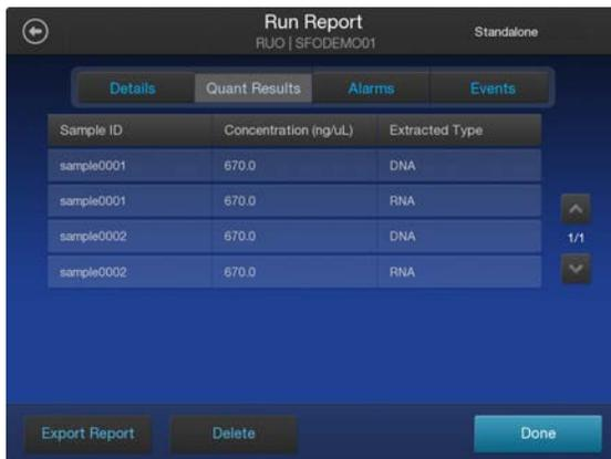
6. Insert a USB drive into the USB port on the front of the instrument, then tap **Export Report**. Navigate to the file destination, then tap **Save**.
