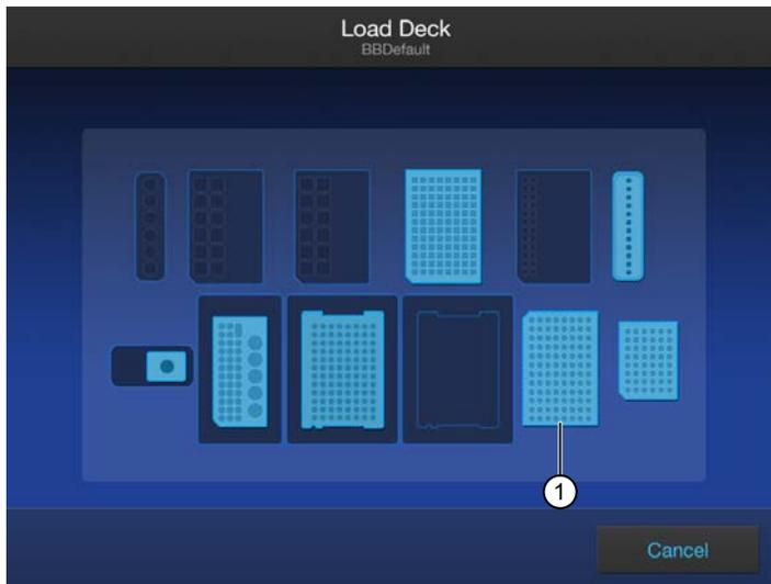
① 96-Well Nucleic Acid Output Plate, only needed when performing the purification in integrated configuration.
