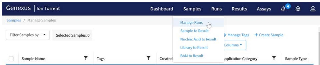
Runs plans that are created in Genexus™ Software contain the settings that are used in sample purification, library preparation, templating, sequencing, and analysis, including sample information and plate location, assays, and barcodes. Run plans are used to track samples, consumables, and chips throughout purification, library preparation, templating, sequencing, and data analysis.
