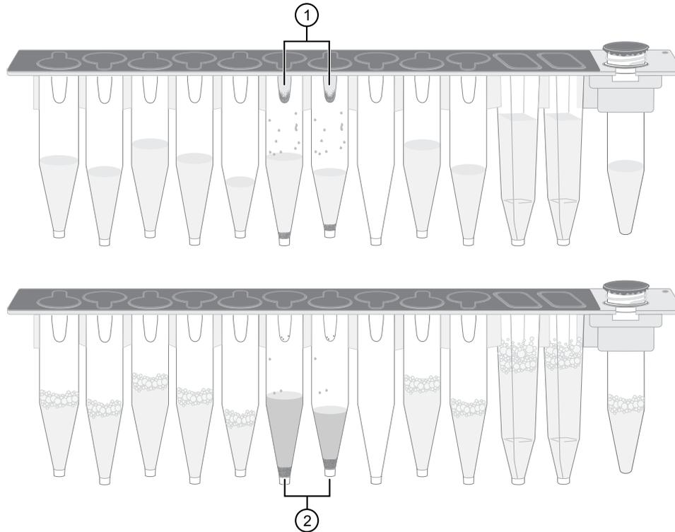
Example Genexus™ Strip 3-GX5™ before (upper) and after (lower) inversion. The carrier has been removed to show tube contents more easily.
