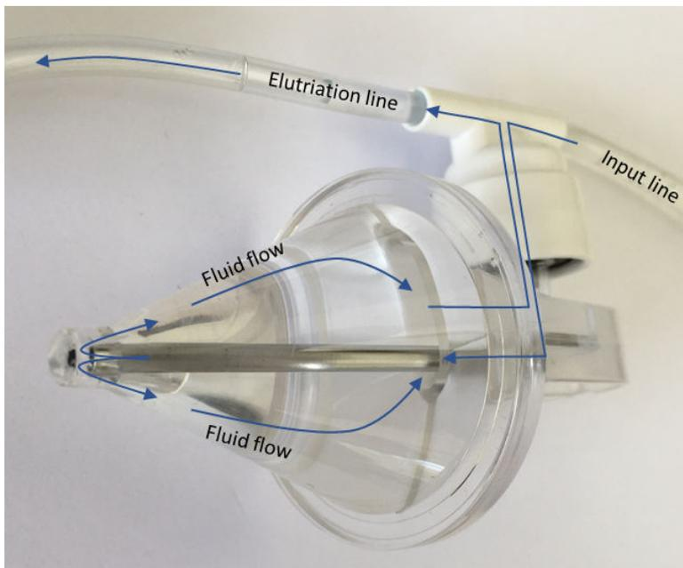
Cells that reach the rear section of the CFC Chamber will accelerate as the diameter reduces and exit via a hole in the back of the CFC Chamber.
