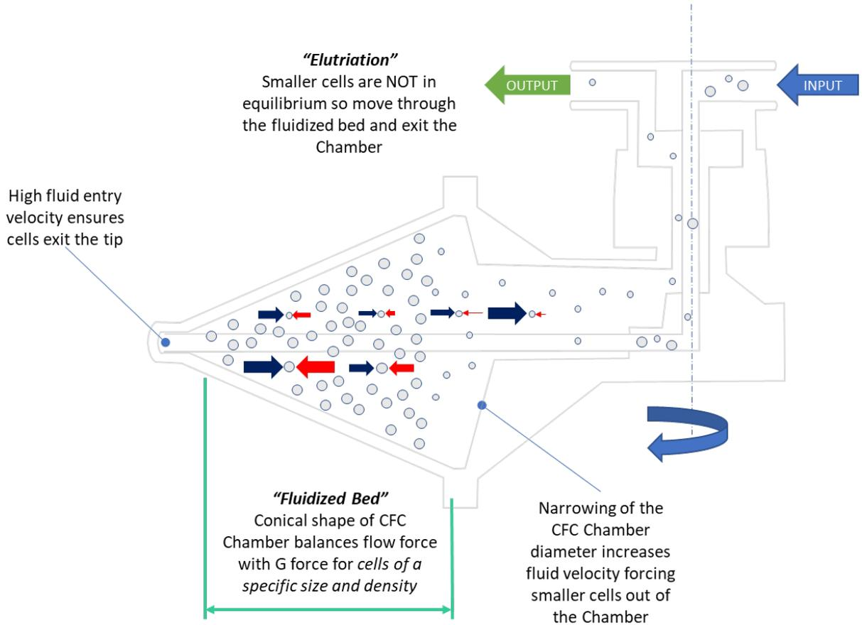
For a specific set of processing conditions (G force and flow rate), a larger cell can be in a stable state in the fluidized bed whilst a smaller cell is not stable and will be washed (elutriated) from the bed.
