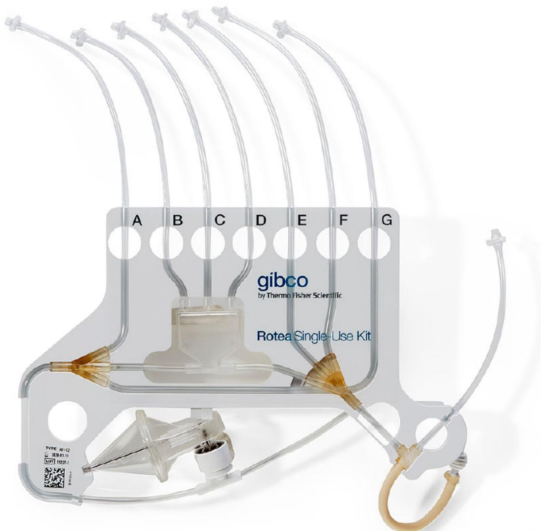
Lines A and G of the Single-Use Kit direct elutriated material (media and cells) to either a waste bag or intermediate bag for subsequent processing.
