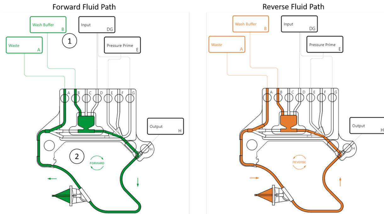
Define the fluid path used in each step using the Single-Use Kit diagram.
