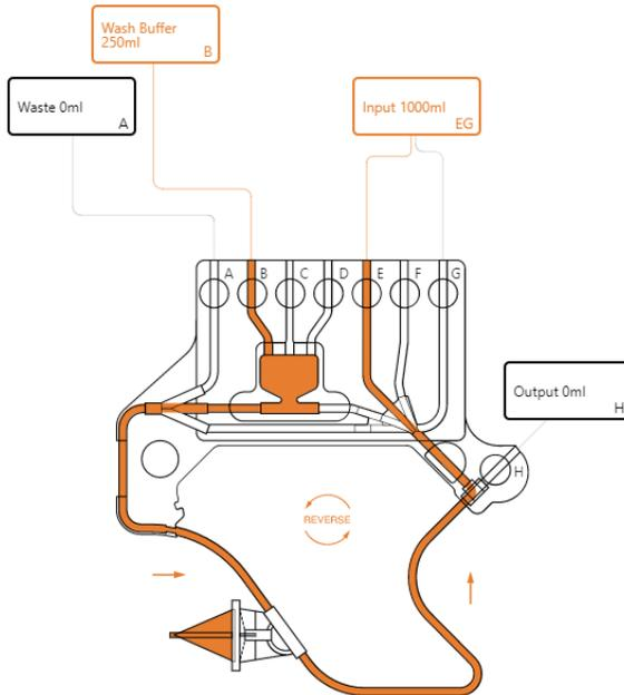
After recovering the concentrate from the previous bite, rinse media connected to lines B, C or D is directed to the input bag, re-priming the input line for the next bite.
