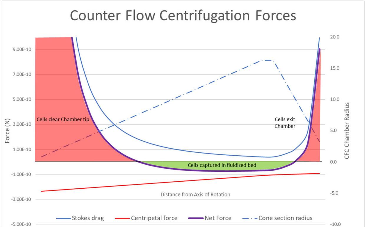
The graph shows the forces acting on a particle at different radial positions.
