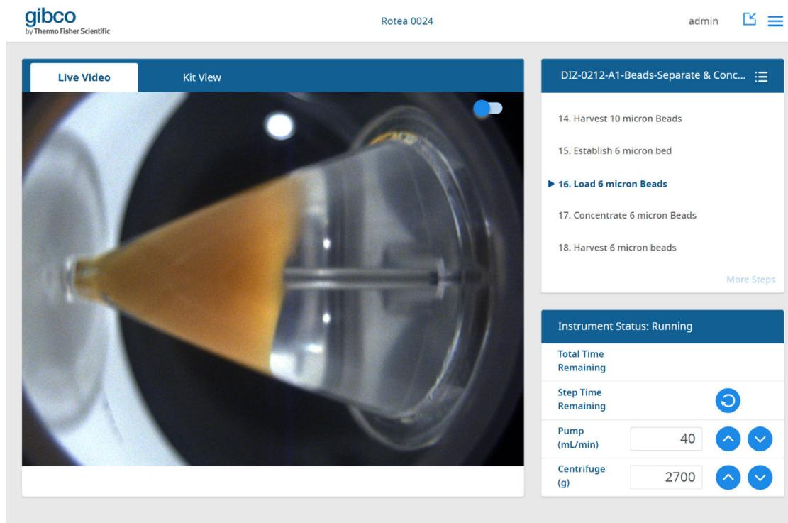
Further optimisation of the settings can be performed based on observation of the fluidized bed using the integrated camera and in-process sampling as adjustments are made to G force and flow rate.
