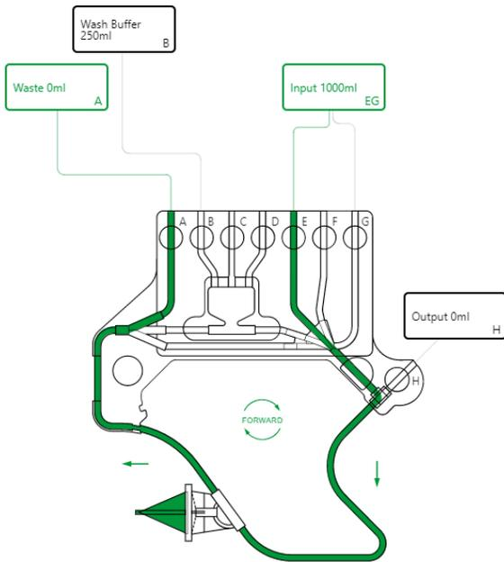
Use one of lines E, F or H as the product input line to take a bite from the input bag and build the fluidized bed.
