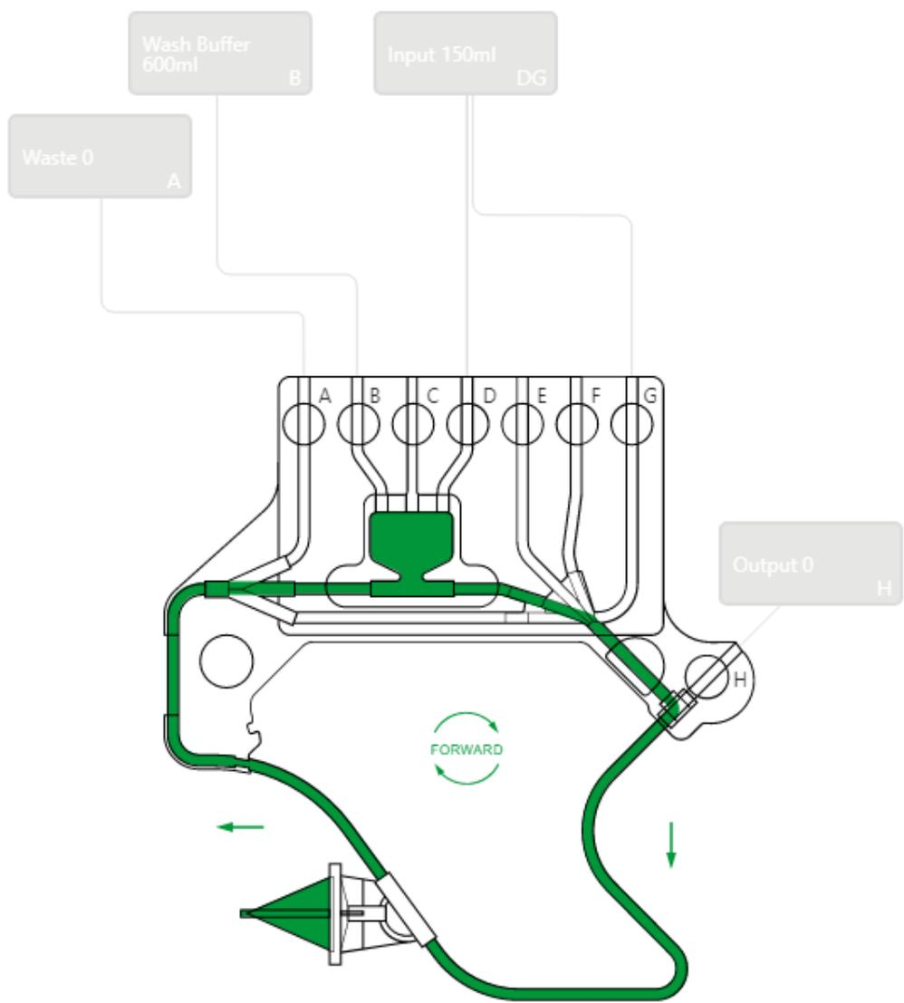
3. **Fill Bubble Trap**– enables the Bubble Trap to be re-primed during a protocol without disrupting the fluidized bed. Only bags connected to lines B, C and D are available for selection for this step type.
