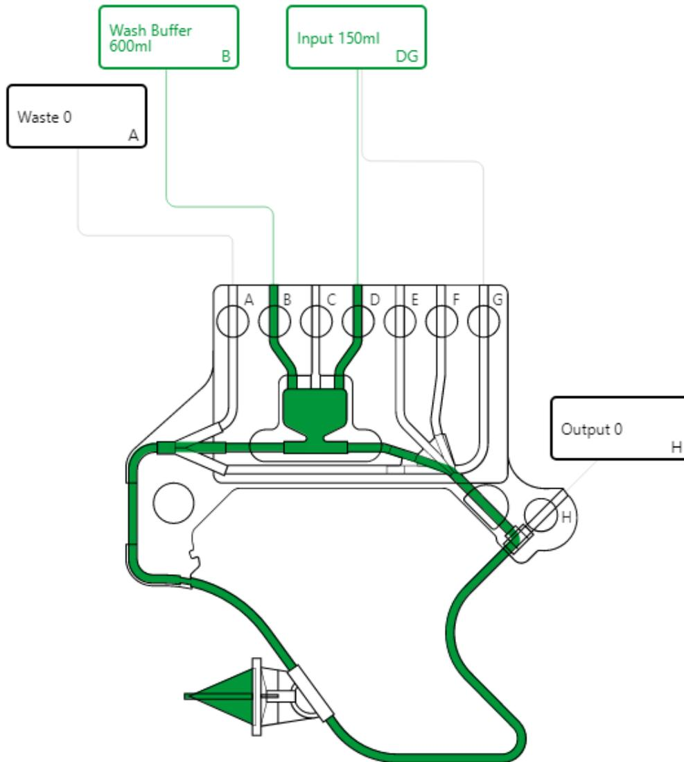
4. **Pressure Prime** – primes lines E and/or F when they are not connected to a bag to minimize losses to these lines during a **Harvest** step.
