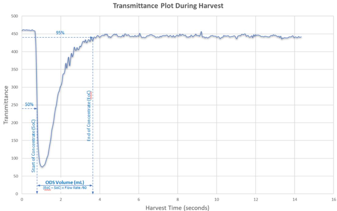
When product is being recovered from the chamber, a high density “slug” of cells is drawn out by the pump. The OD Sensor detects this as a sudden drop in transmittance.
