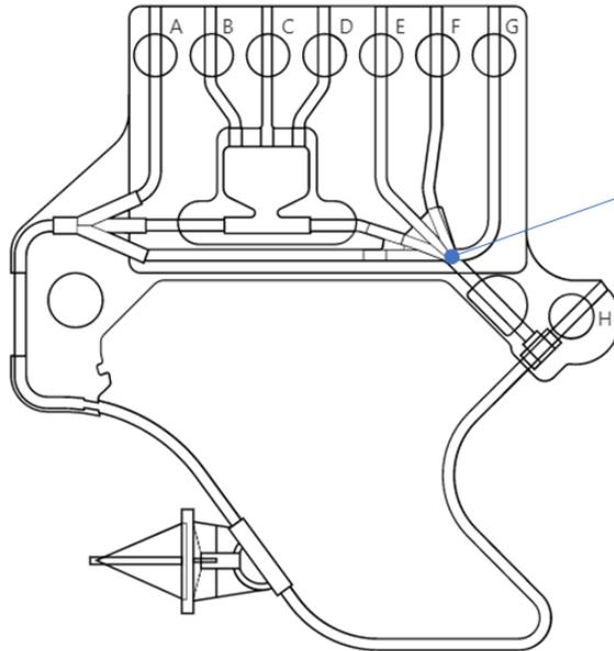
**Note:** Line G is equivalent to Line A and runs **underneath** lines E & F without connecting to them.
