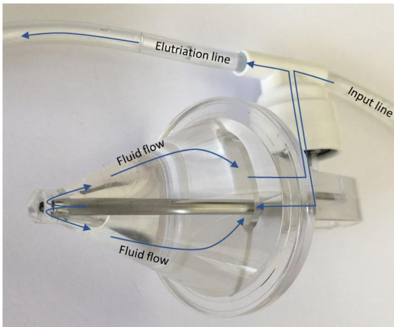
Media containing both large and small cells enters the Rotary Coupling via the input line and flows into the CFC Chamber, exiting at the tip of the stainless-steel Dip Tube.
