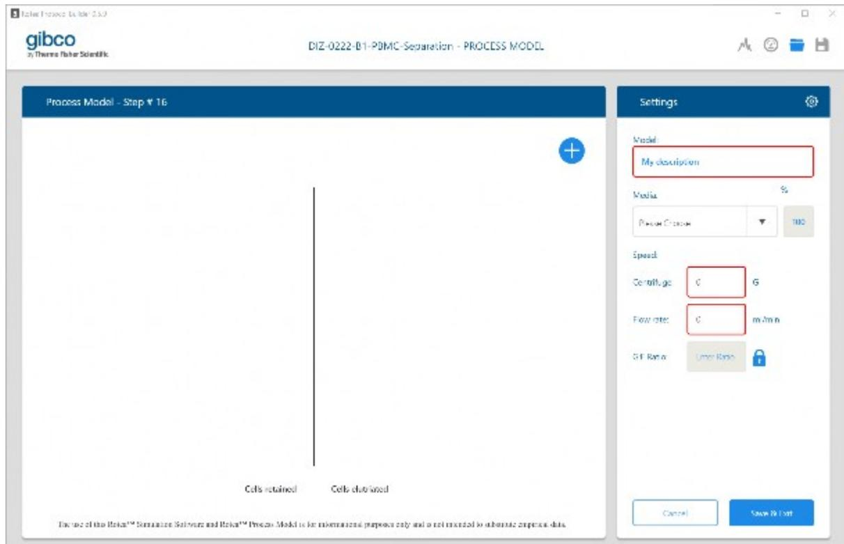
The vertical line in the middle of the panel represents the zero-force line i.e. where the centripetal and Stokes drag force on the particle are in equilibrium. This means that:
