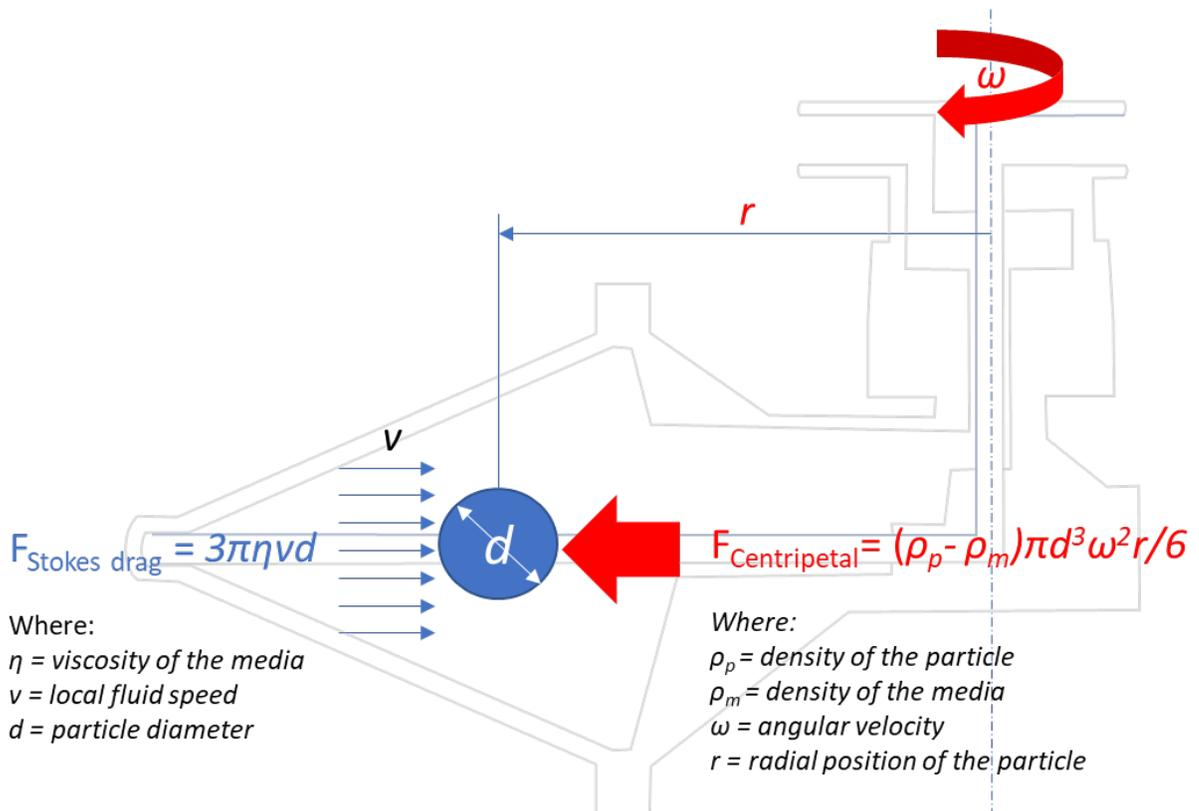
$$F_{\text{Net}} = F_{\text{Centripetal}} - F_{\text{Stokes drag}}$$
