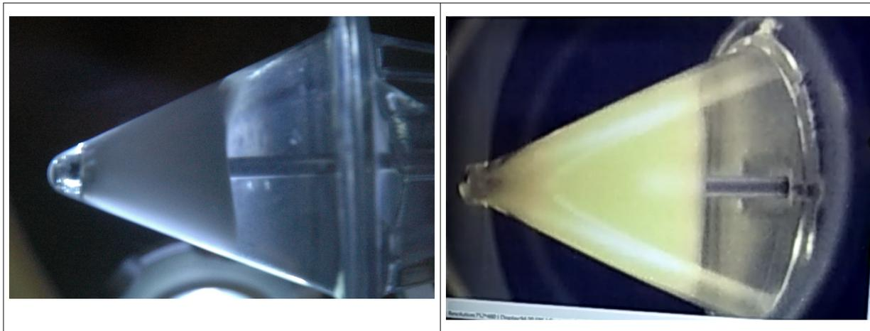
Examples of fluidized beds highlight predicted behavior. The left image is of beads. The very clear zone in the tip clearly reflects the expected clear zone highlighted by the red zone in the chart. The image on the right is CHO cells with a well-formed bed.
