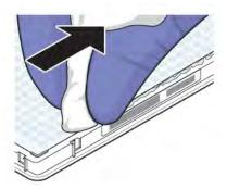
**IMPORTANT!** You must remove any excess glue from the plate.
