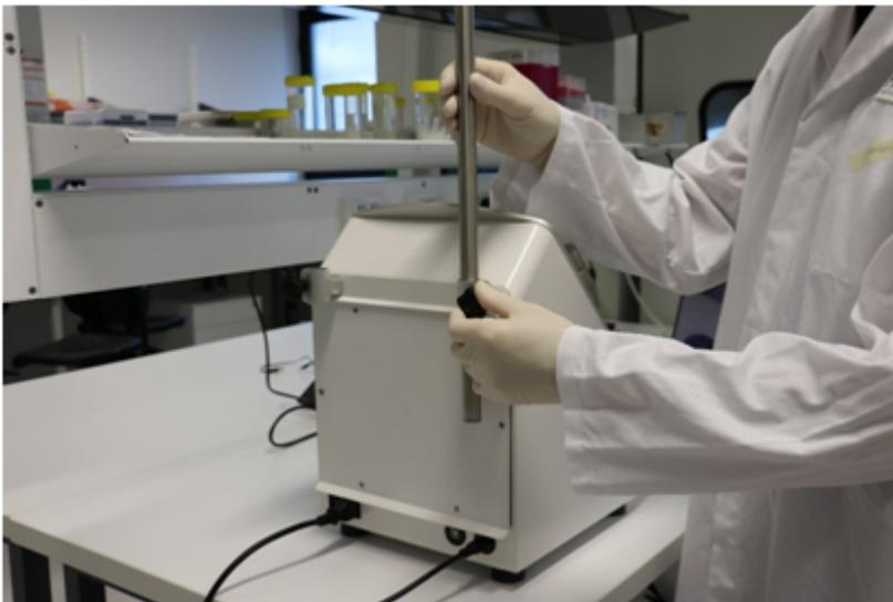
5. Adjust the instrument position on the bench where it is required.
