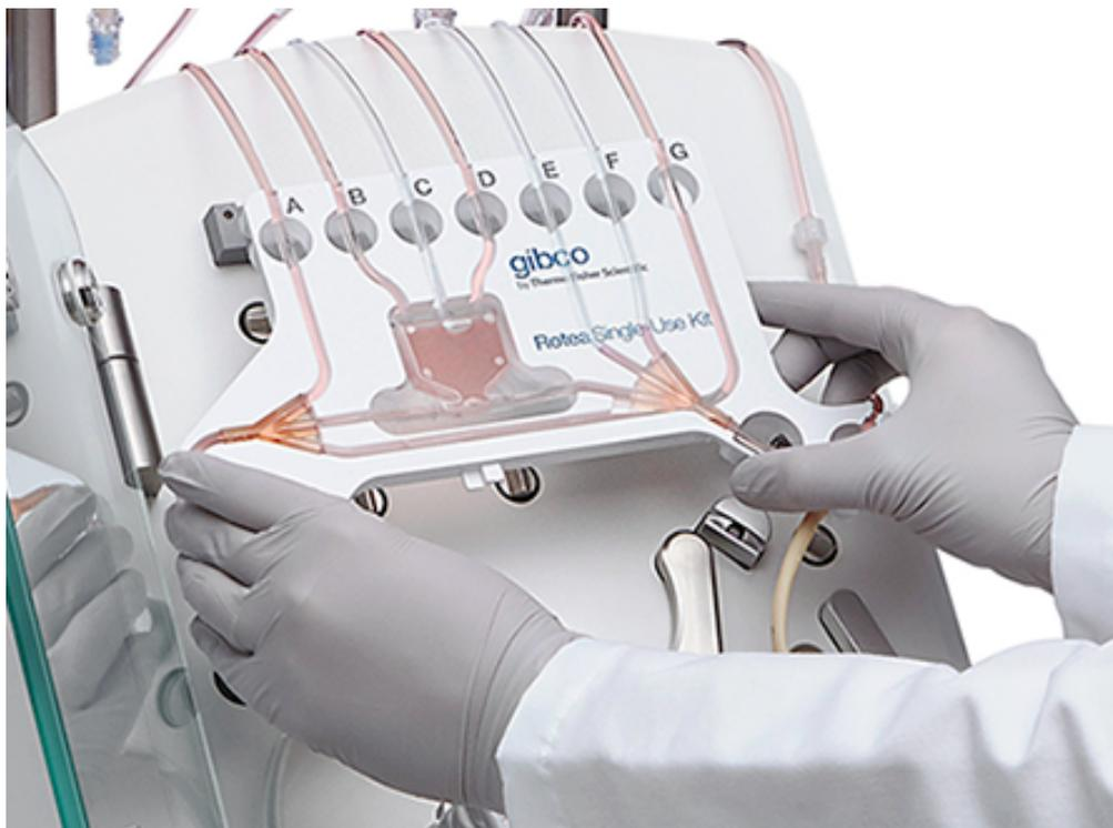
4. Install the CFC Chamber into the CFC Chamber Carrier.
