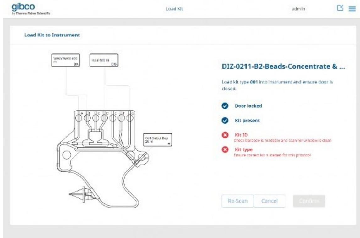
6. Manually confirm that the Single-Use Kit configuration matches the image and that manual clamps have been opened.
