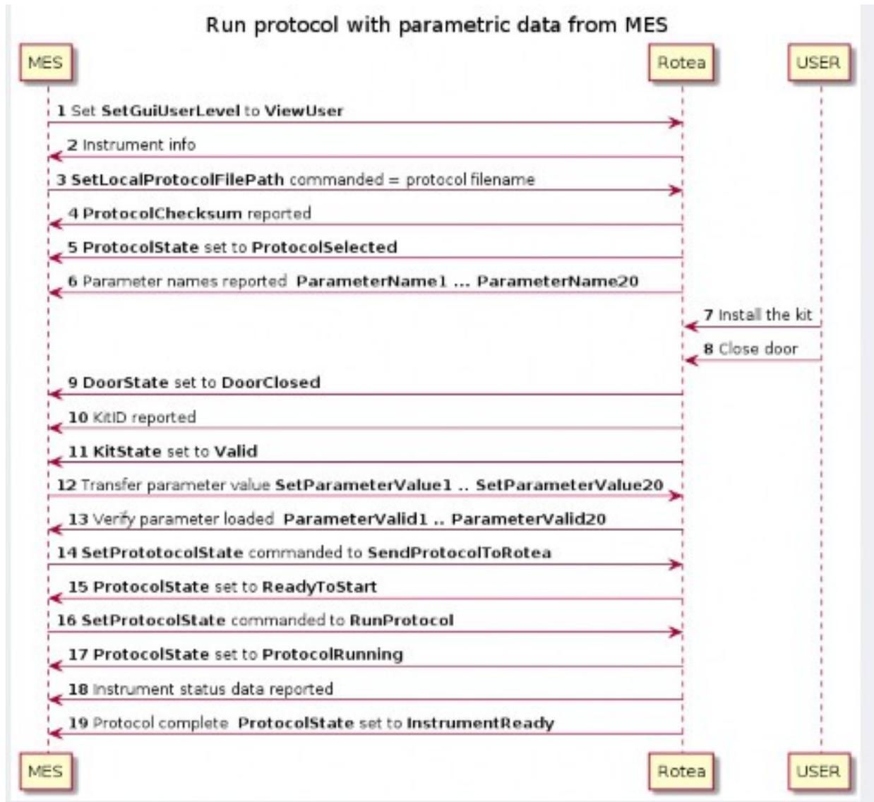
Figure 14 Run a simple protocol with parameters
