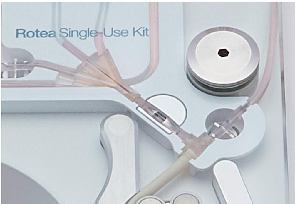
3. Rotate the hex key clockwise to unlatch the door. The total movement is 90 degrees to release the latch.
