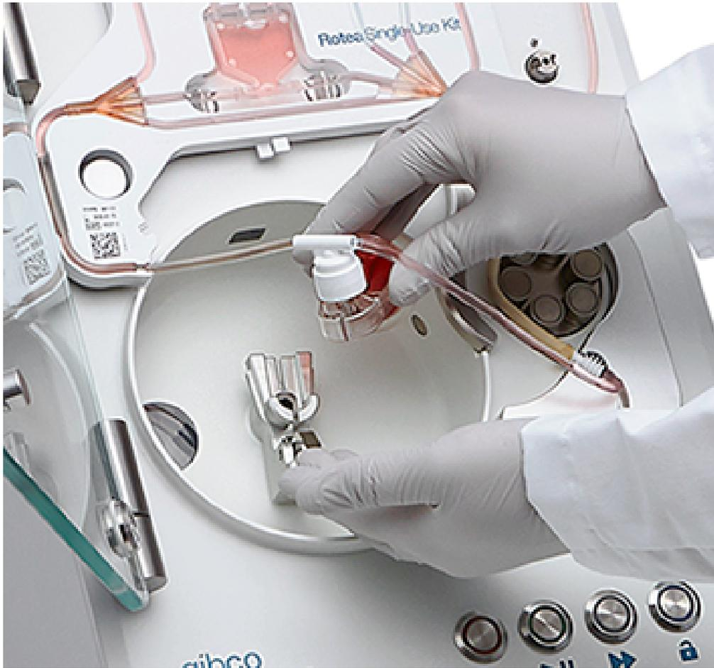
6. Gently raise the Carrier Frame drawing out the tubes from the Bubble Sensor.
