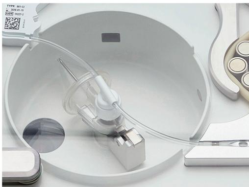
5. Insert tubes A, B, C, D, E, F & G into the corresponding slot in the Bubble Detector Strip and push downwards with fingers to fully engage each tube in the slot.
