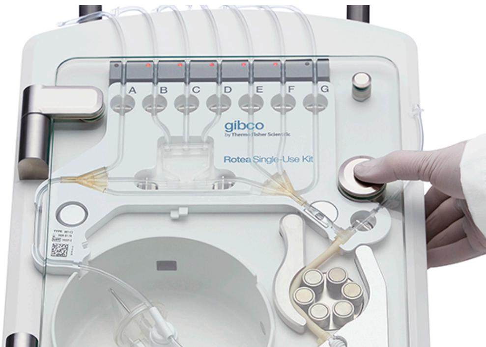
4. (auto): Closing the door initiates the following automatic system checks. The status of each system check is displayed on the Rotea™ GUI with  indicating correct installation of the Single-Use Kit.
