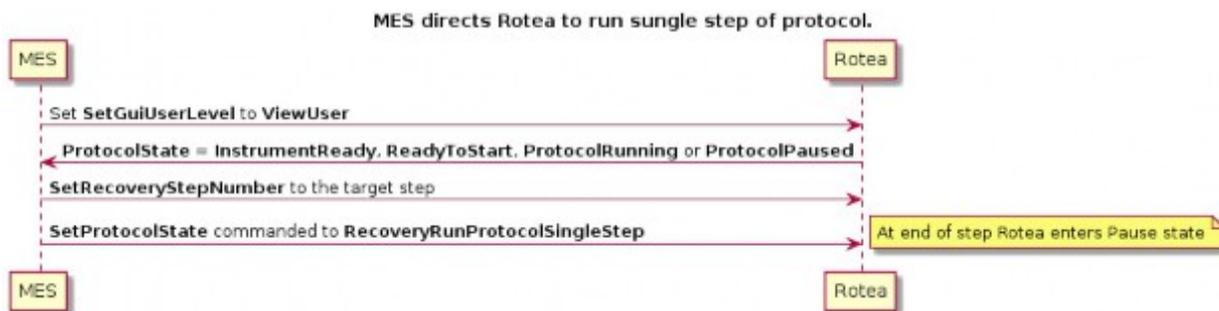
Figure 16 Perform single step recovery operation from OPC-UA while running a protocol
