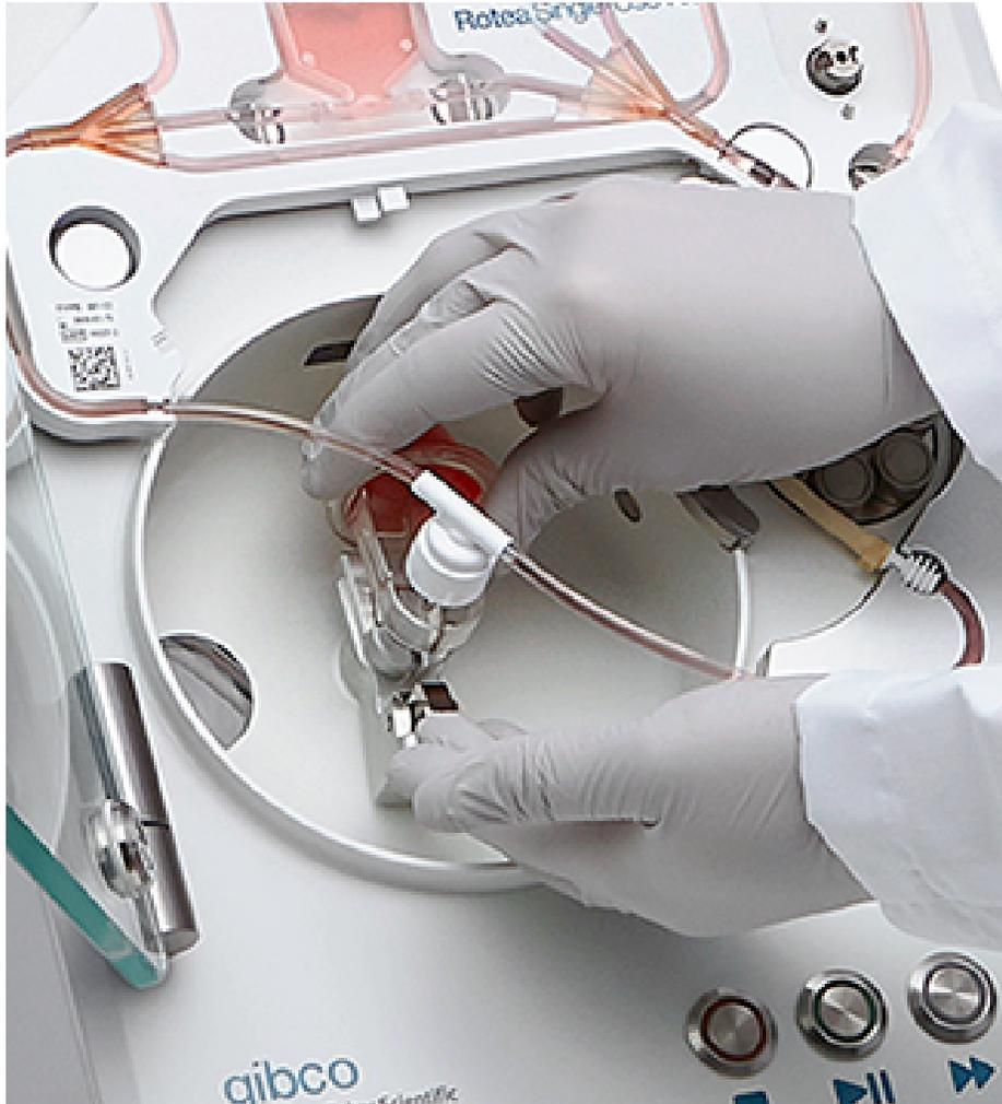
4. Lift CFC Chamber clear of the Centrifuge Carrier.
