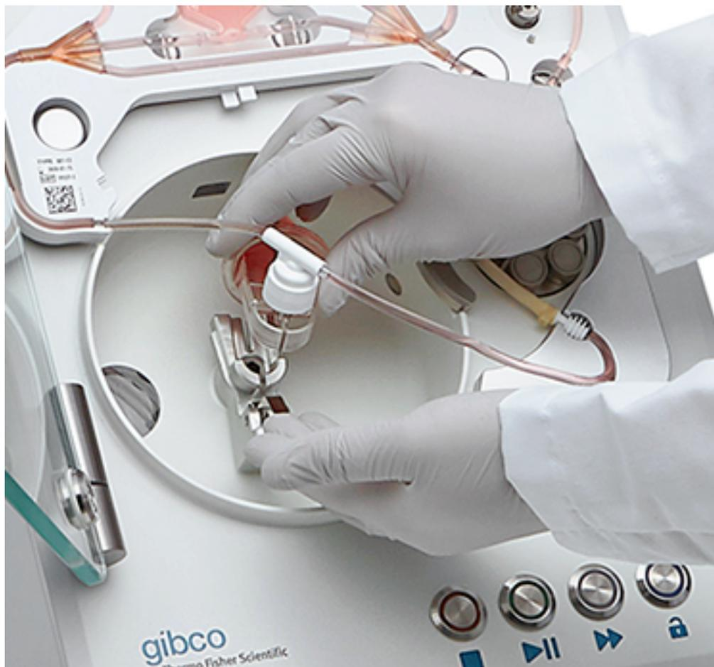
5. Remove the tubing from the Sensor Block and Peristaltic Pump.
