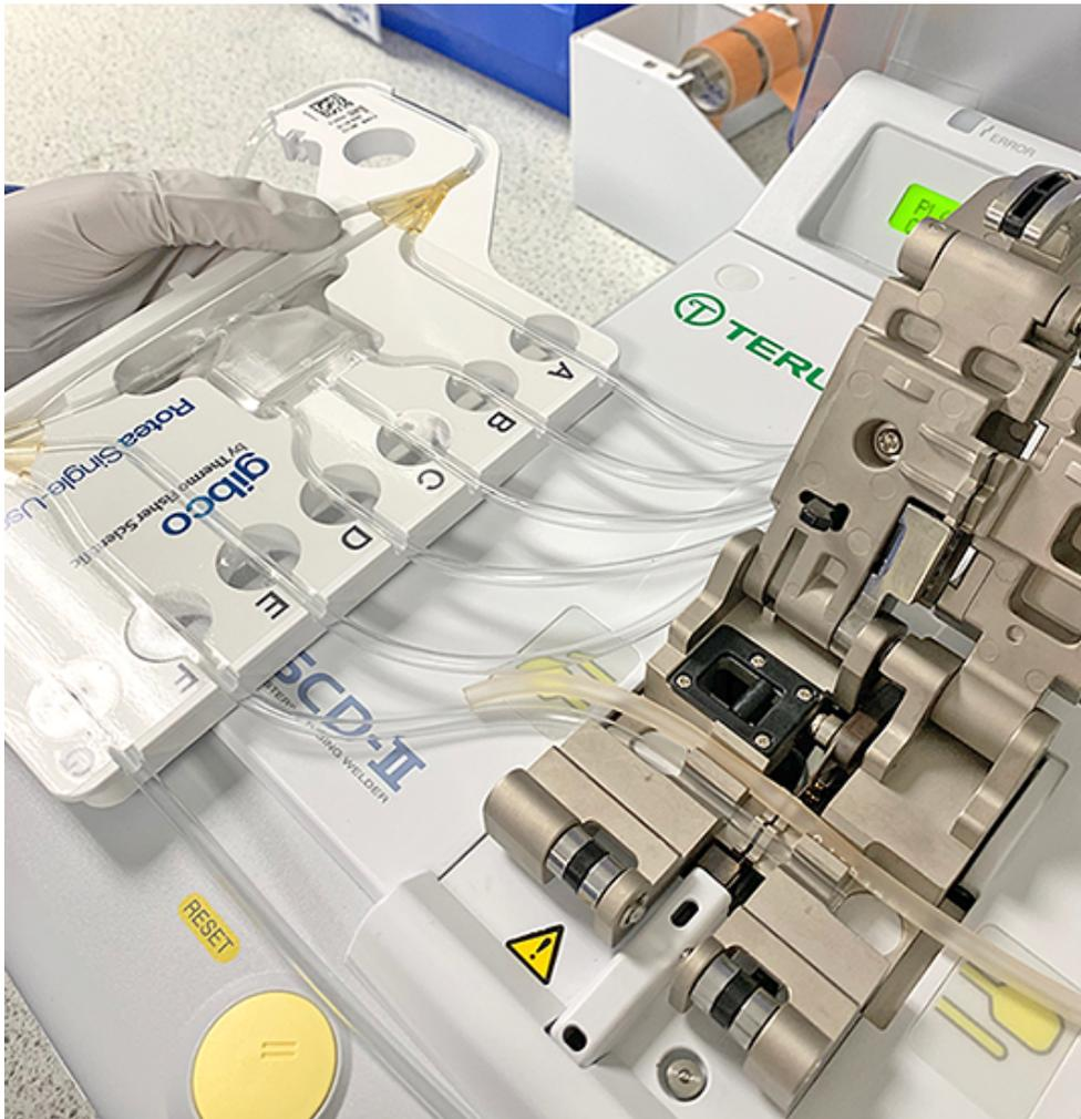
Figure 8 TSCD II Sterile Tubing Welder (TerumoBCT)
