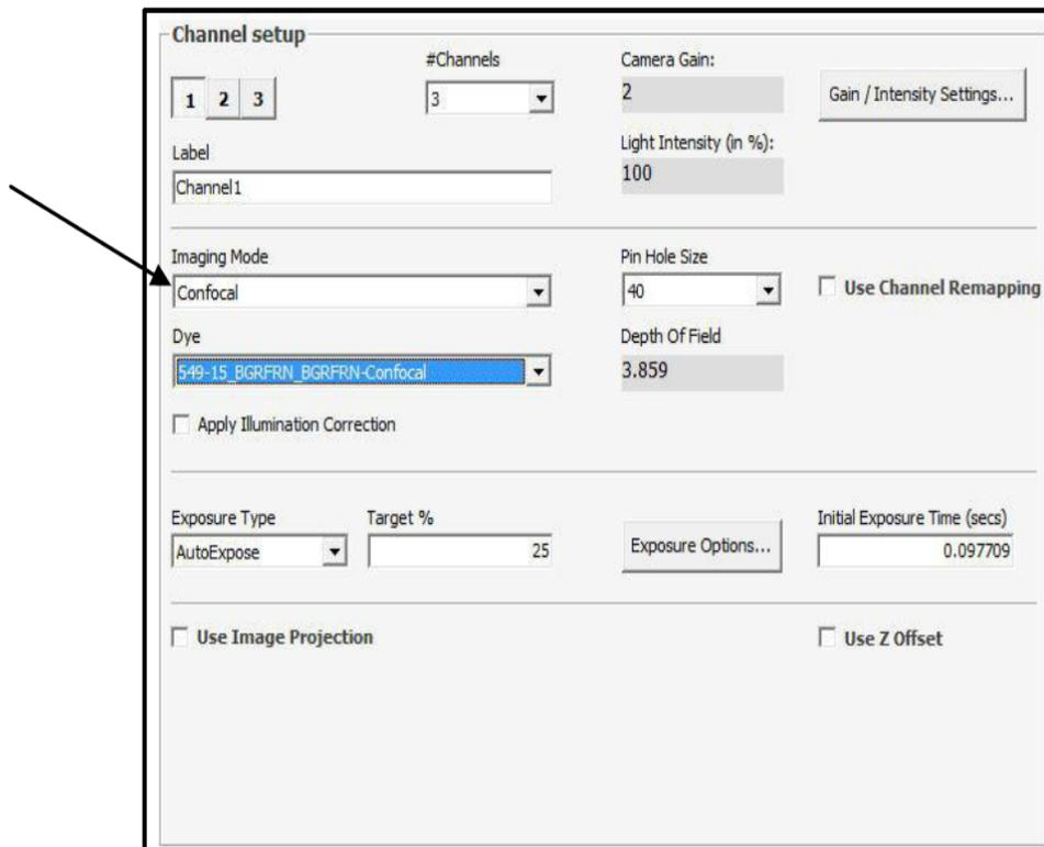
3. The filter options are dependent on the **Imaging Mode** selection. Select the desired Confocal filter set from the **Dye** drop down menu.
