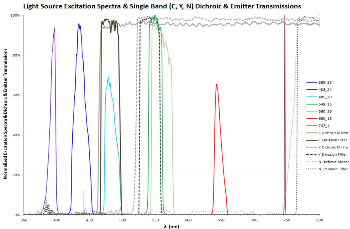
Figure 46 Single band matched C, Y, and N dichroic mirrors and emission filters transmission spectra, overlaid with the normalized spectral power distribution from the excitation 7-color light engine
