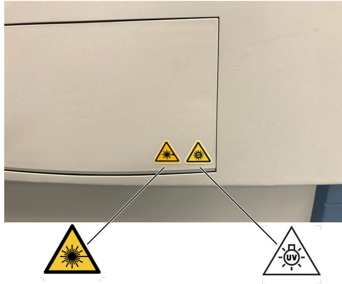
Figure 57 Label placement – CellInsight™ CX7 Pro HCS Reader front (front flipper door)
