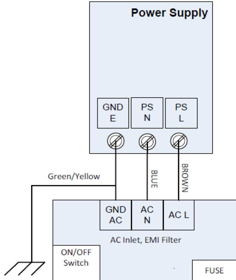
Figure 33 CellInsight™ CX7 Pro HCS Reader System Connection Diagram – Power A/C and D/C
