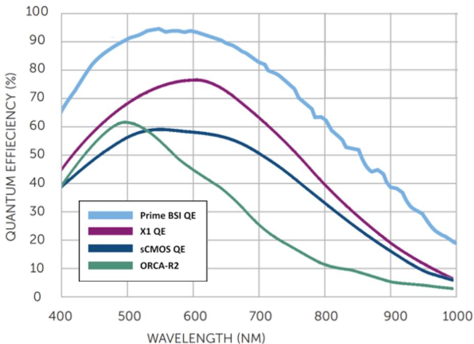
Figure 38 Camera quantum efficiency vs. wavelength
