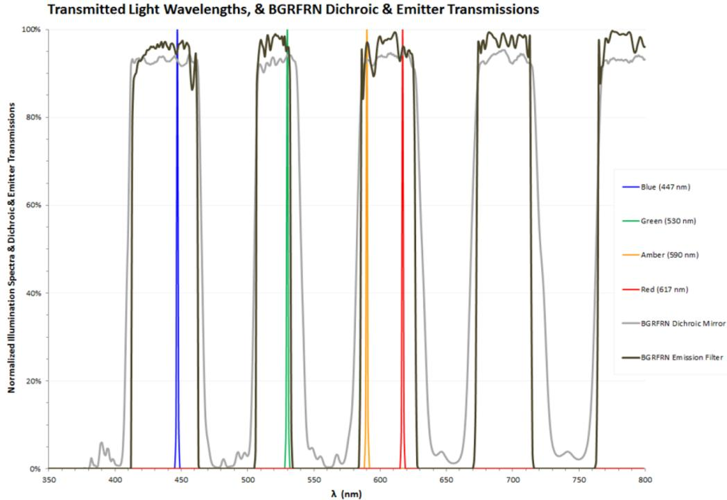
**Figure 52** Penta-band BGRFRN dichroic mirror and emission filter transmission spectra, overlaid with the normalized spectral power distribution from the transmitted light source’s four illumination colors
