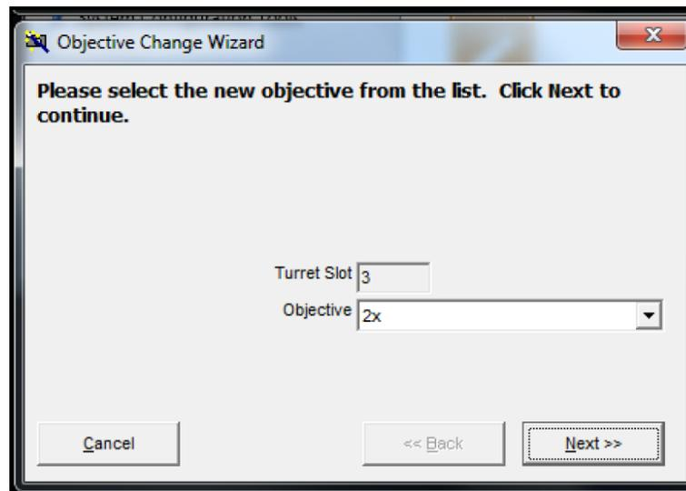
10. The following screen appears. Insert the new objective in the Load/Unload Position by following the instructions on screen. Close and lock the service door. Click **Next** to continue.
