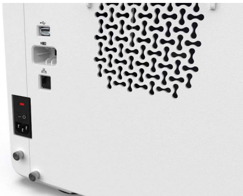
Figure 9 Turn off the instrument using the on/off switch or disconnecting mains power.
