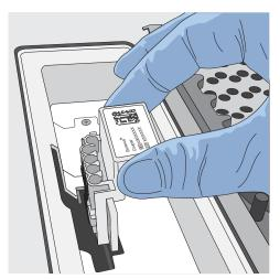
**Note:** A chip shuttle under the deck moves the installed chip to loading and sequencing positions during the run.
