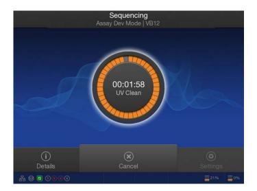
5. After UV cleaning, if all the chip lanes were used, the sequencing reagents bay doors unlock. Open the doors, remove used components from the bay and empty the Waste carboy, then tap **Next**.
