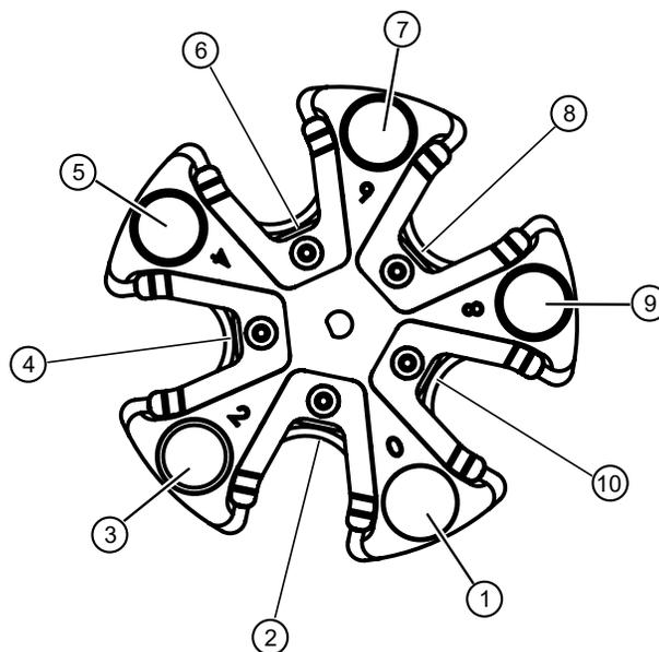
**Figure 8 Emission filter wheel**
