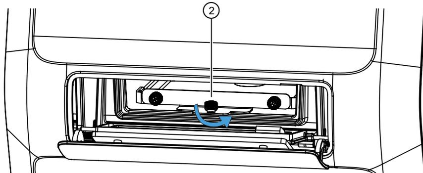
3. Pull the transport lock ③ until the plate carrier is fully out of the measurement chamber.
