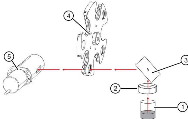
**Figure 9 Operating principle of luminometric measurement**
