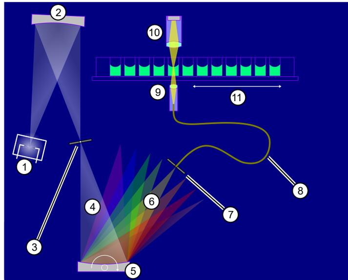
**Figure 5** Operating principle of absorbance measurement
