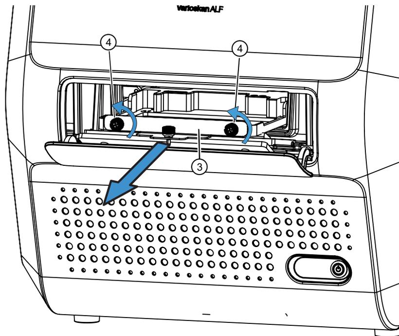
5. Push the plate carrier back into the measurement chamber and make sure that the measurement chamber door closes properly.
