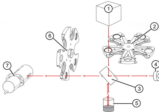
**Figure 6 Operating principle of fluorometric measurement**
