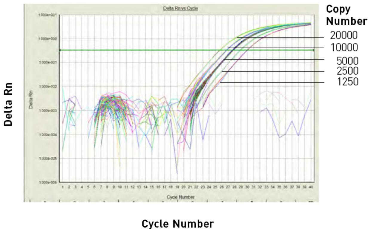
Figure 30 Amplification plot from a real-time run of an RNase P instrument verification plate
