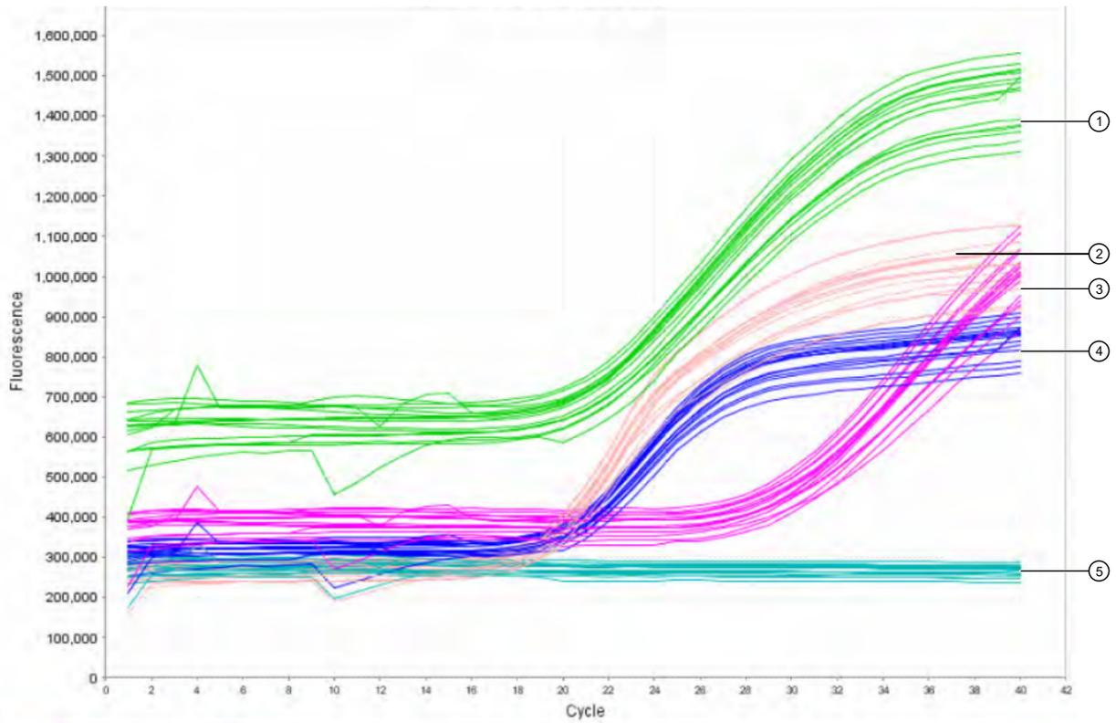
Figure 20 Multicomponent plot with noise between cycles 3-15
