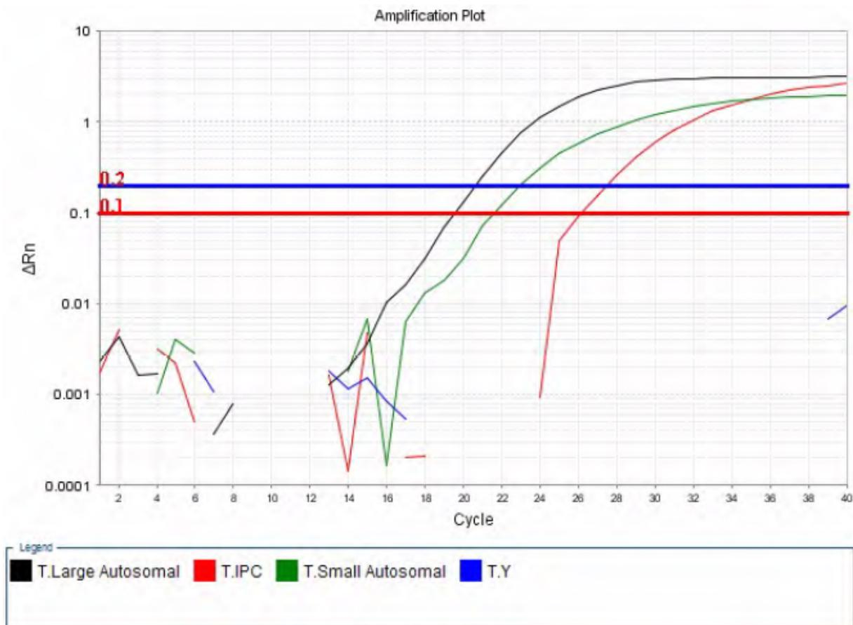
Figure 17 Typical female amplification plot (horizontal blue line= $C_T$  threshold for small autosomal, large autosomal and male targets; horizontal red line= $C_T$  threshold for IPC)
