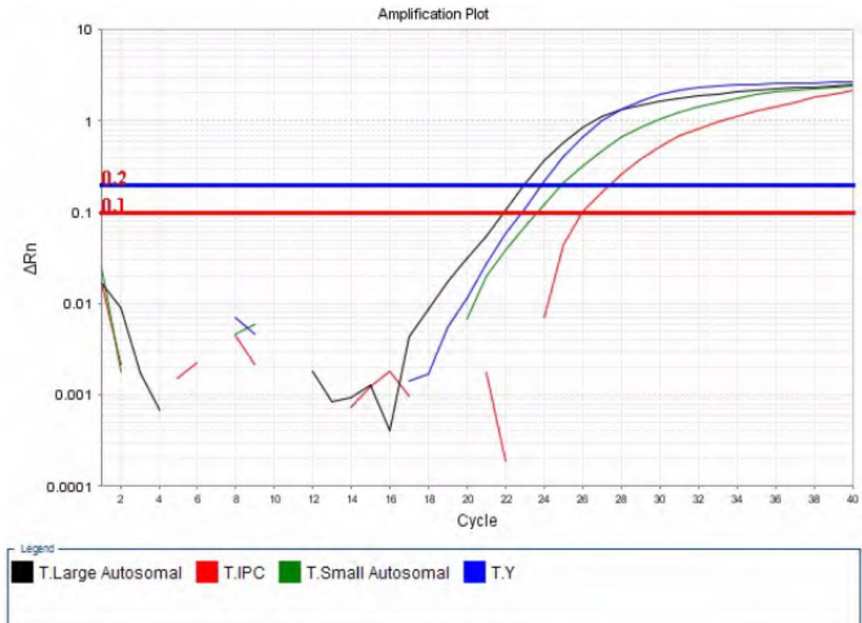
Figure 16 Typical male amplification plot (horizontal blue line indicates the  $C_T$  threshold for small autosomal, large autosomal and male targets; horizontal red line indicates the  $C_T$  threshold for IPC)
