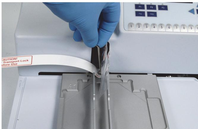
**Figure 11–48.** Fastening the transport lock
