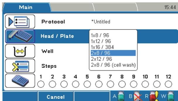
The default wash head setting is set in the **Settings** menu. When a one-column wash head (1x8 or 1x12) is used, the blank wash head should always be on the left of the wash head arm (viewed from the front).
