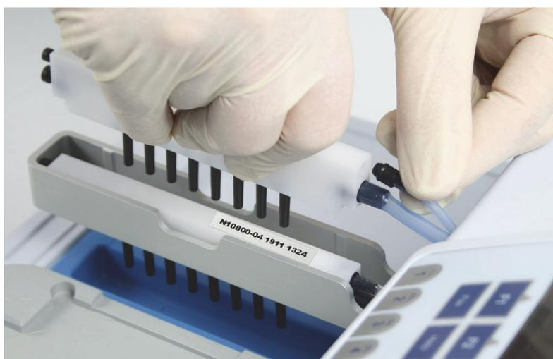
**Figure 2–10.** Fitting the wash heads to the connectors
