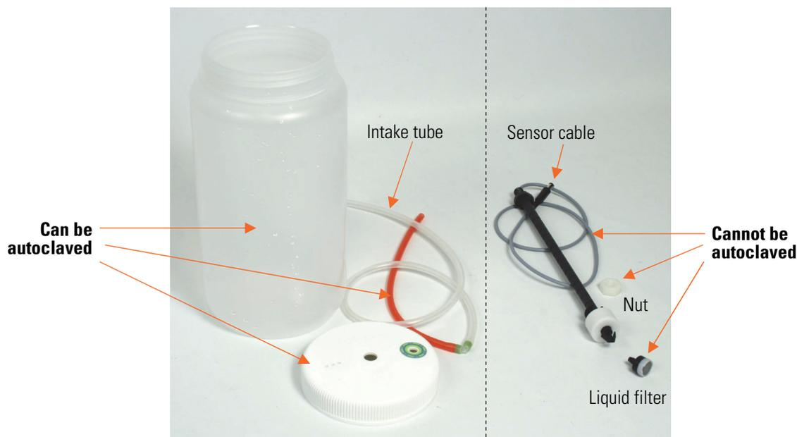
**Figure 11-44.** Autoclavable and un-autoclavable liquid bottle parts
