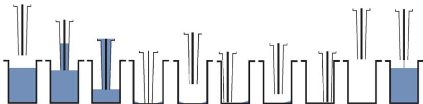
**Figure 1–5.** Principle of washing step (Sweep3)
