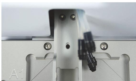
**Figure 11–47.** Aligning the plate carrier and wash head arm
