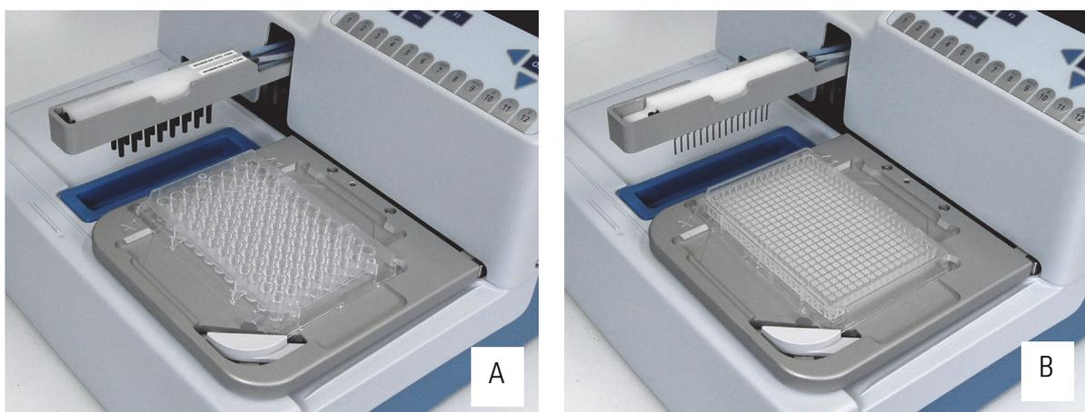
**Figure 5–31.** 2x8 orientation (A) and 1x16 orientation (B)
