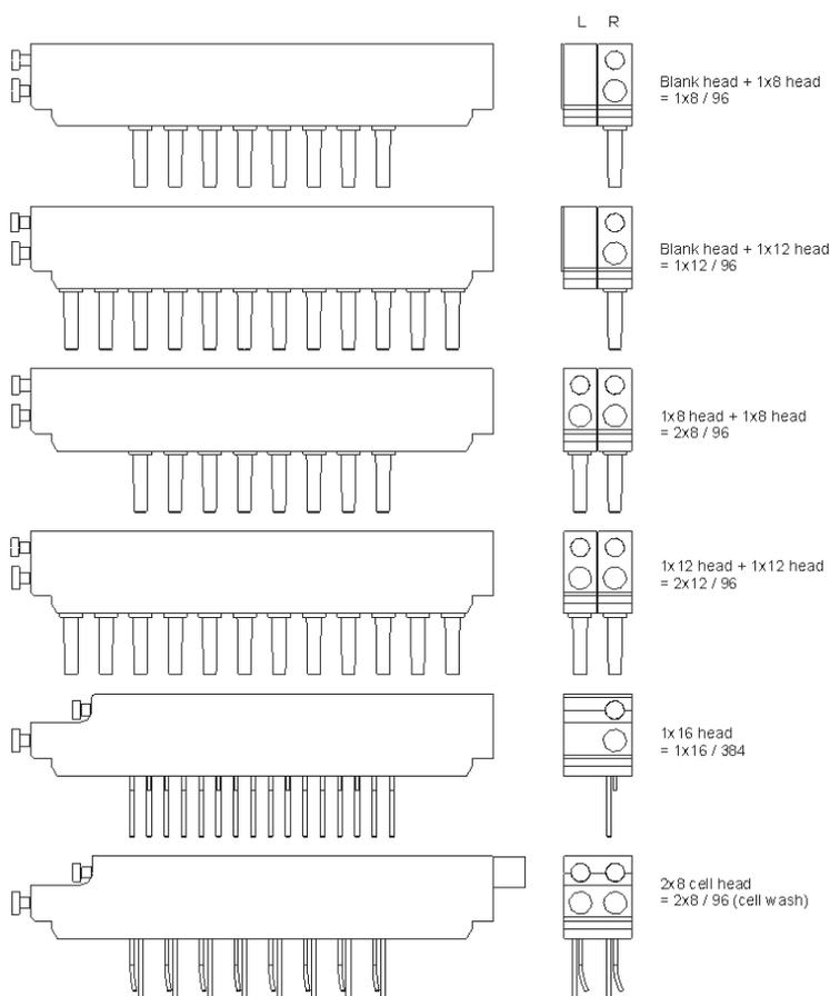
**Figure 3–29.** Configurations of Wellwash Versa wash heads
