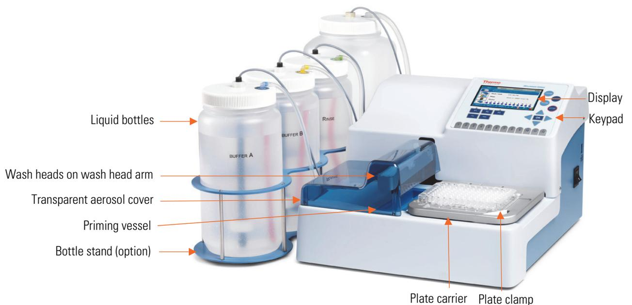
**Figure 3–24.** Wellwash Versa front view with accessories
