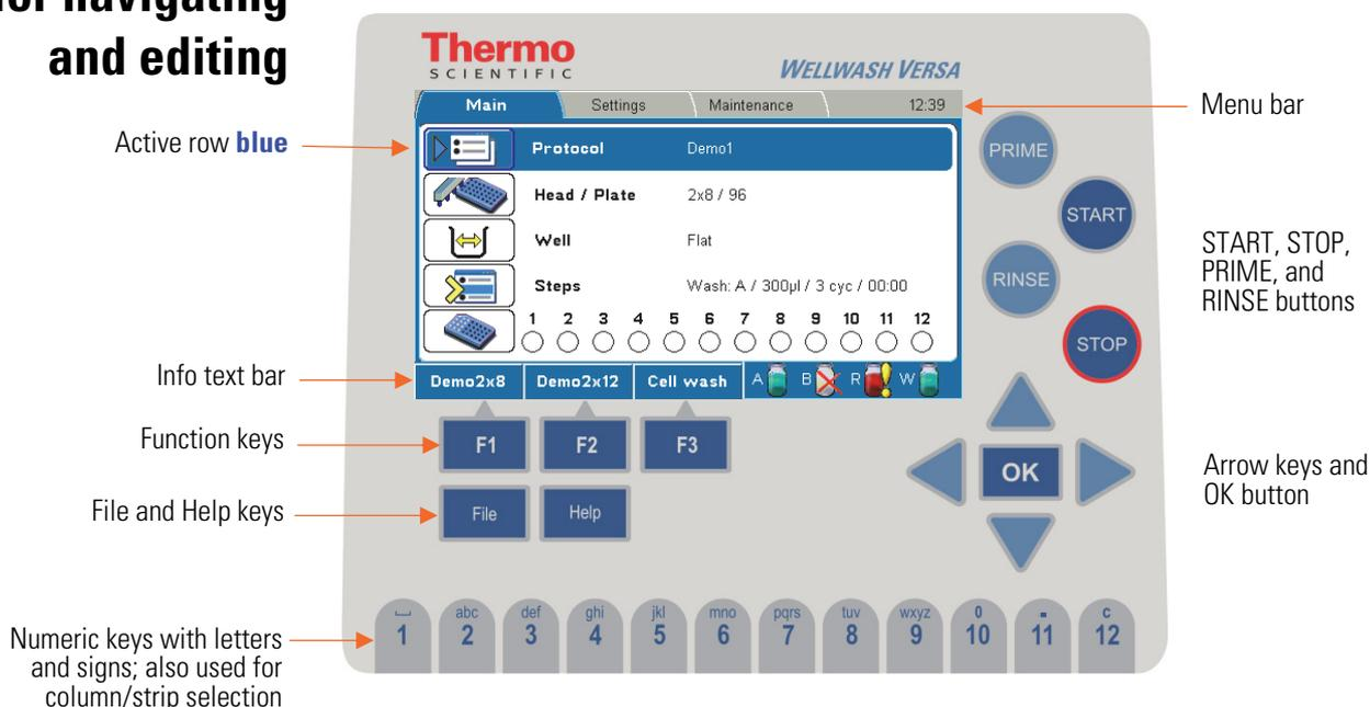
**Figure 4–30.** Keypad and display of the Wellwash Versa
