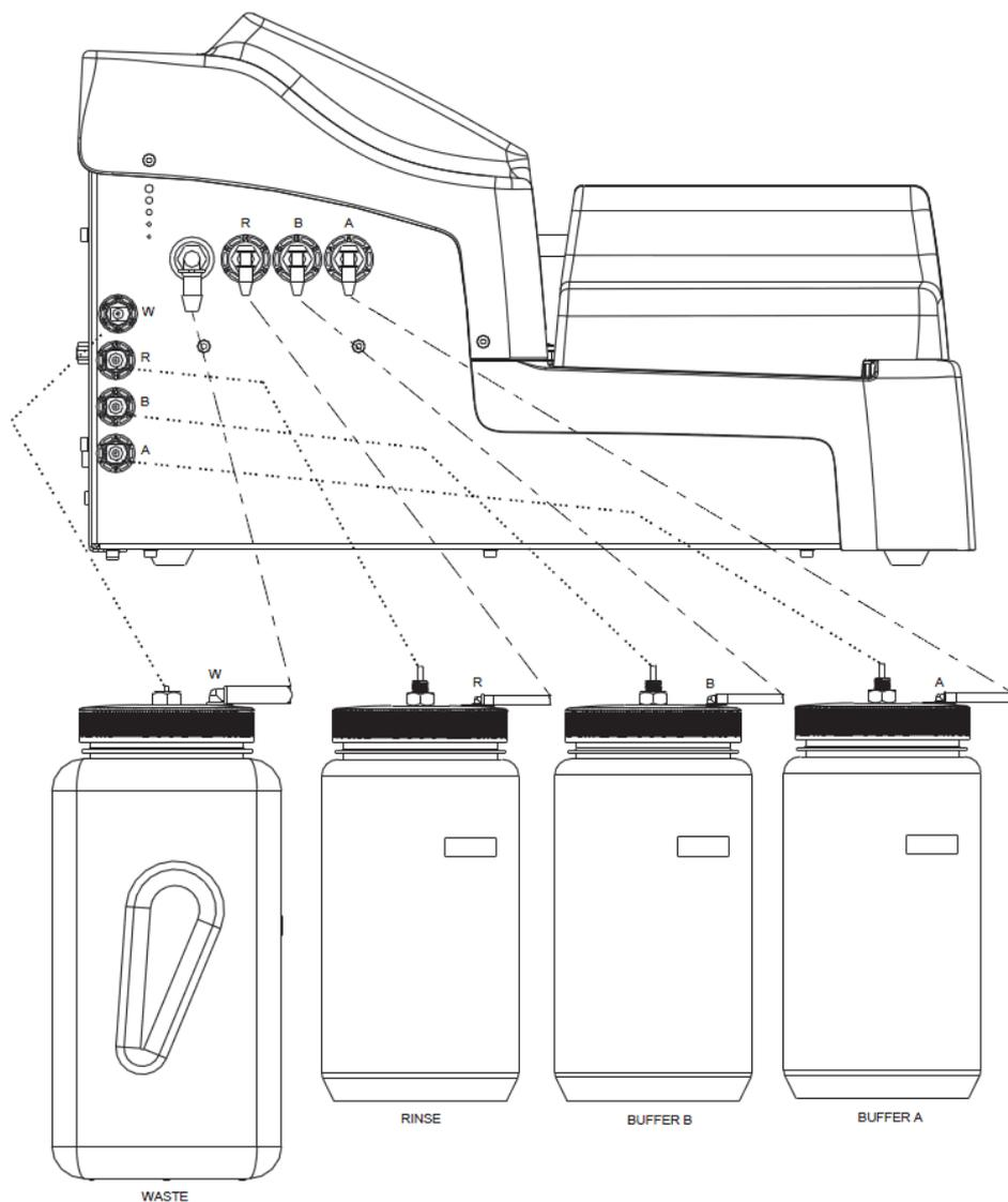
**Figure 2–17.** Wellwash Versa connection diagram
