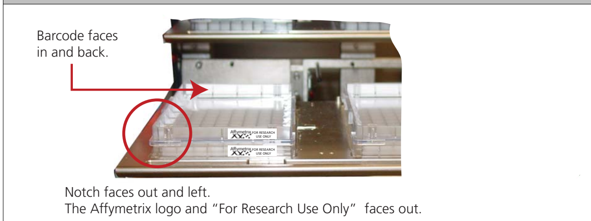
Figure 5.28 The Proper Installation of the GeneTitan Tray Consumables (the image shows the Stain Tray and the Stain Tray cover as an example)
