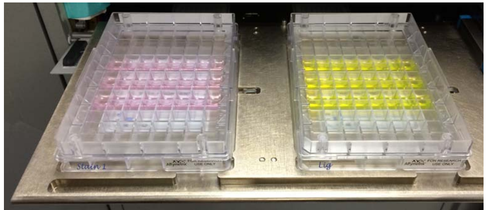
Figure 5.31 Stain 1 Tray and Ligation Tray Loaded in Drawer 3
