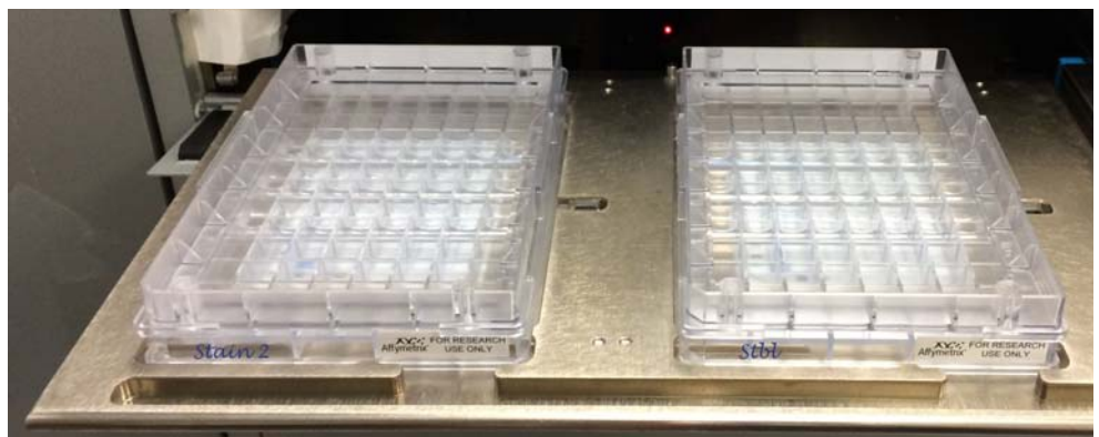
Figure 5.32 Stain 2 Tray and Stbl Tray Loaded in Drawer 4
