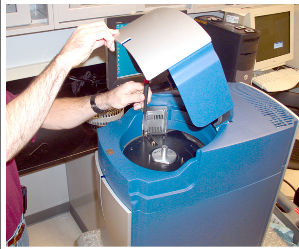
Figure 248 Locating the rescue hole
