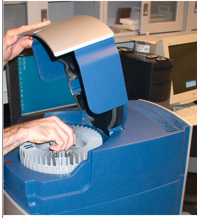
Figure 231 Inserting and turning the carousel. the carousel must be seated and flush with housing.
