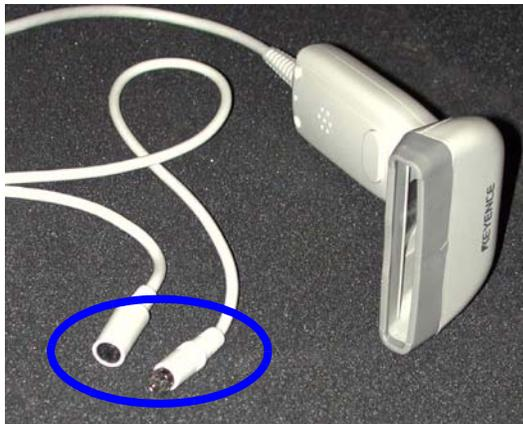
An external barcode reader can also be used with the 3730/3730*xl* Analyzer. The KEYENCE BL-80VE (see photo above) connects to the instrument computer keyboard. With this reader, you can scan barcodes into any text box in the Data Collection software.
