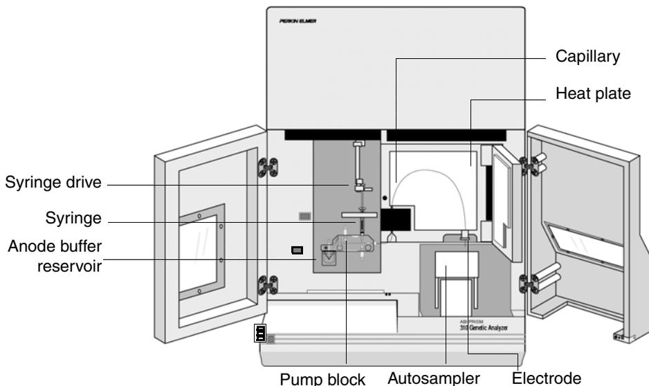
**Figure 8-1** ABI PRISM 310 Genetic Analyzer
