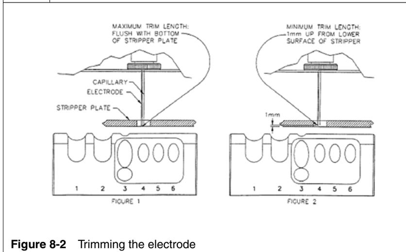
**Figure 8-2** Trimming the electrode
