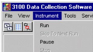
**Controlling the Run Using the Toolbar** You can also use the toolbar at the top of the 3100 Data Collection software window to control the run.
