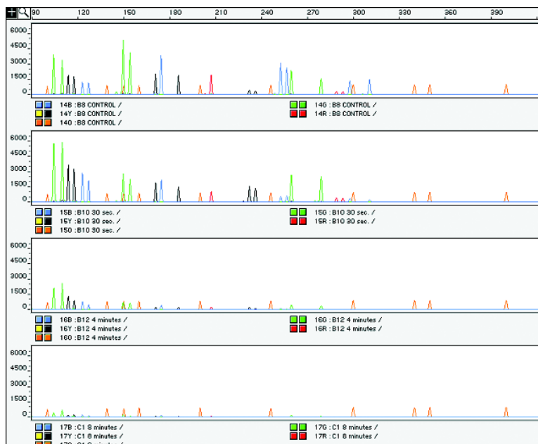
Figure 8-19 Multiplex amplifications of a DNA sample in the absence of DNase I and the sample incubated for 30 sec, 4 min, and 8 min with DNase I, analyzed using the ABI PRISM 310 Genetic Analyzer
