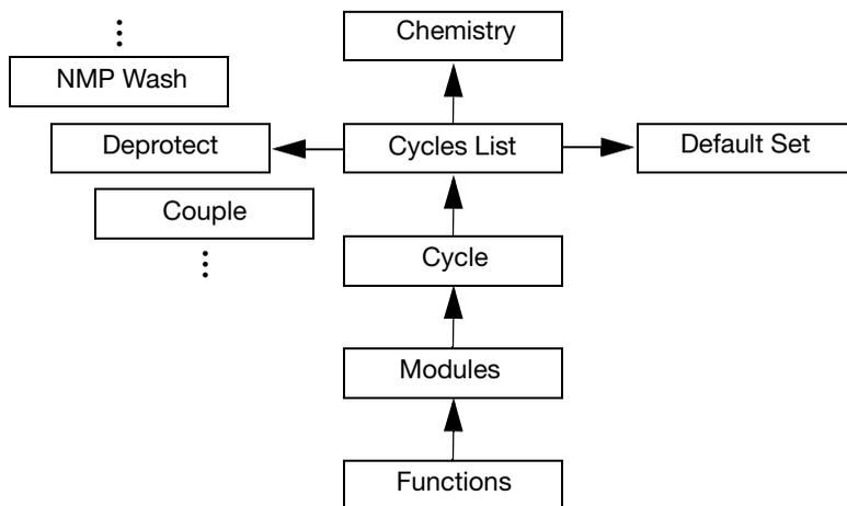
**Figure 7-1 Hierarchy of the Chemistry Software**
