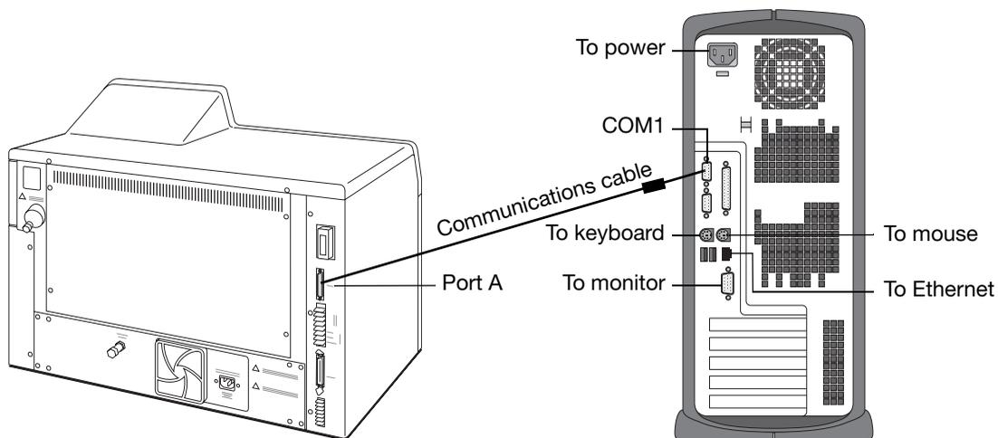
Figure 2-2 Installed Configuration
