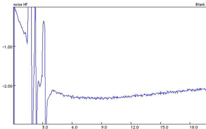
Figure A-1 High-frequency noise (the scale of the diagram has been increased to exaggerate the noise)
