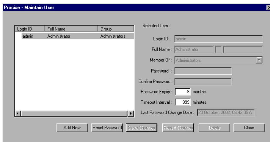
All fields will be grayed out except the Password Expiry and the Timeout Interval field. The Timeout Interval is the amount of idle time allowed before the software will log out a user. The default values are 9 months for password expiration and 999 minutes for the timeout interval. Custom default values can be set at this point or these values can be set individually as each user is set up.
