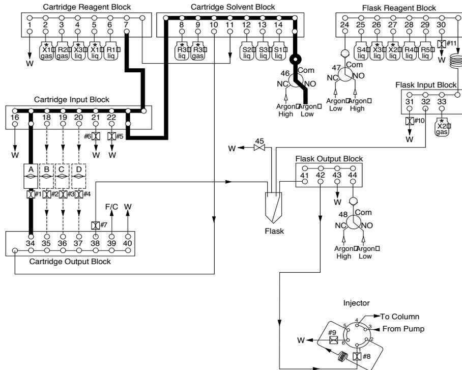
Figure 6-1 Flow path for Cartridge Leak test performed on Cartridge A
