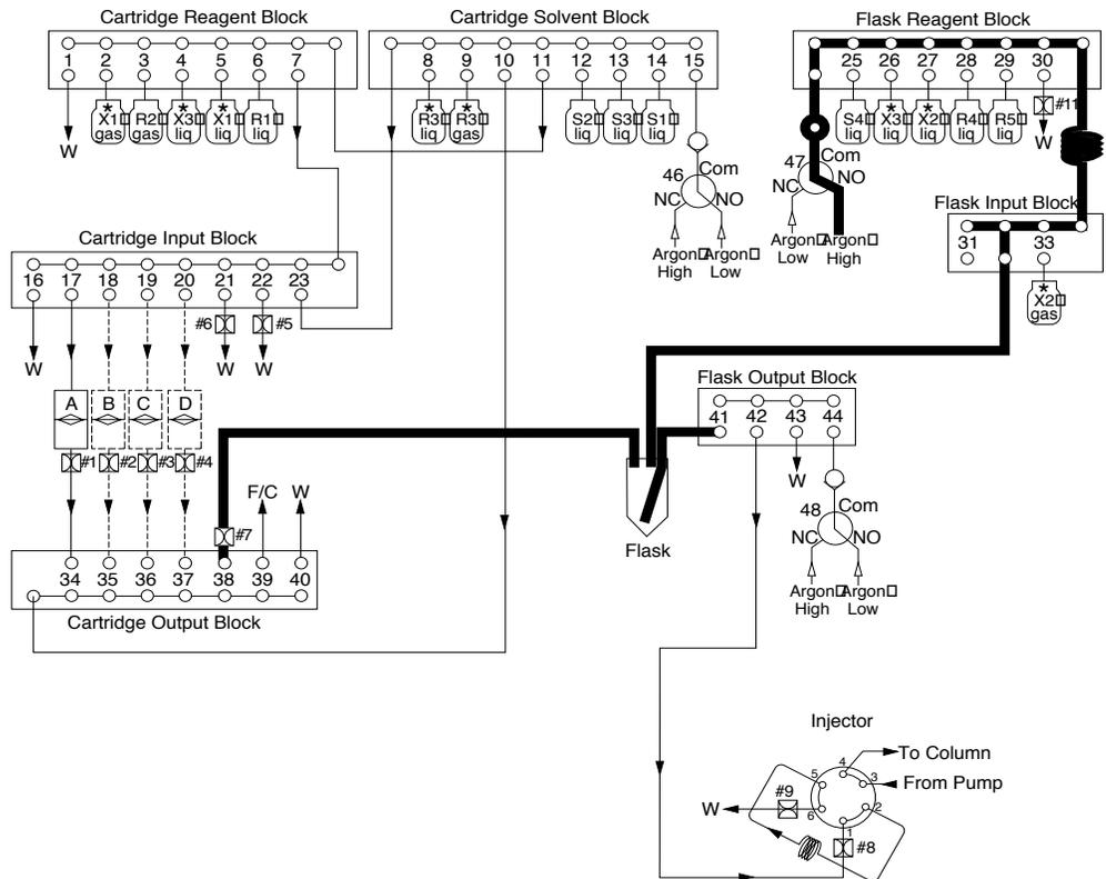
Figure 6-2 Flow path for the Flask Leak test
