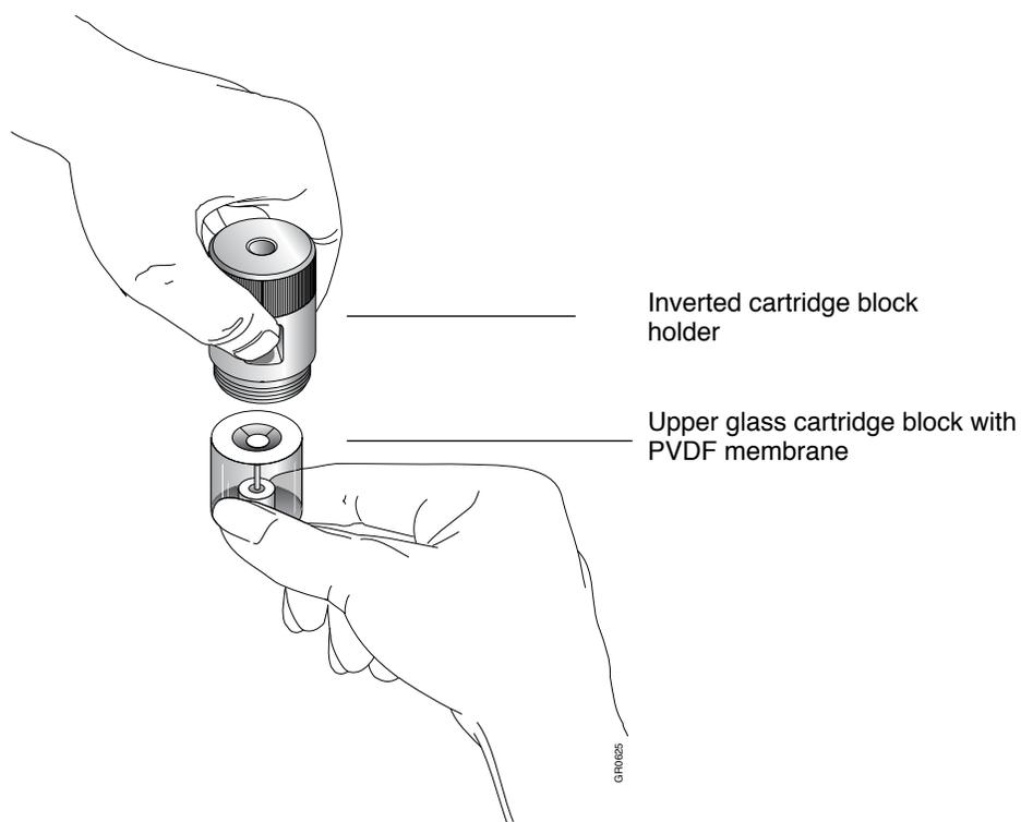
Figure 3-5 Slide the upper glass cartridge block with PVDF membrane up into the cartridge block holder
