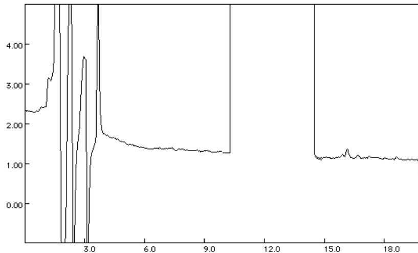
Figure A-9 Air bubble in flowcell
