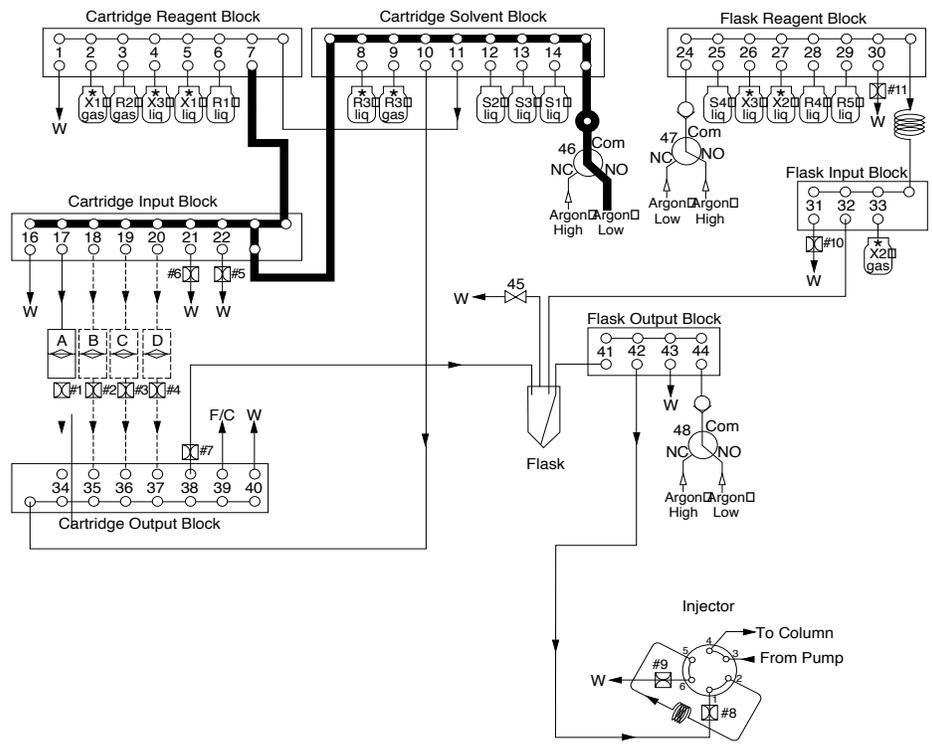
Figure 6-4 Flow path for the Cartridge Input Block Leak test
