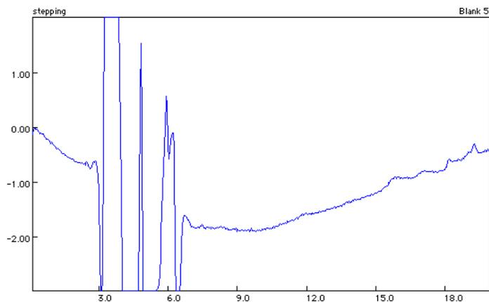
Figure A-5 Leaking pump seal
