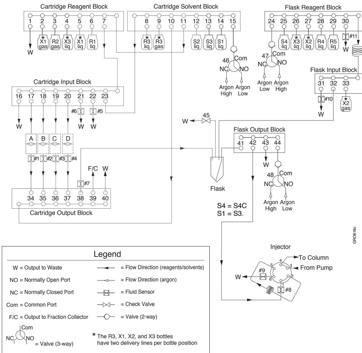
Figure C-1 Procise cLC Protein Sequencer valve diagram
