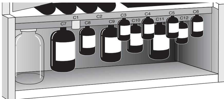
Figure 1-4 PROCISE C protein sequencer bottle configuration
