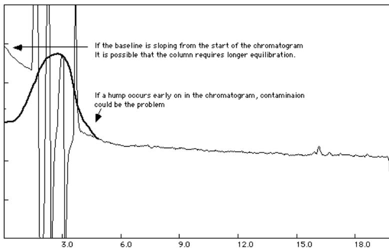
Figure A-7 Slope or hump at start of chromatogram
