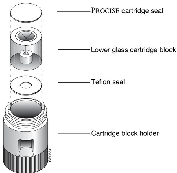
Figure 3-2 Reassembling the lower portion of the reaction cartridge
