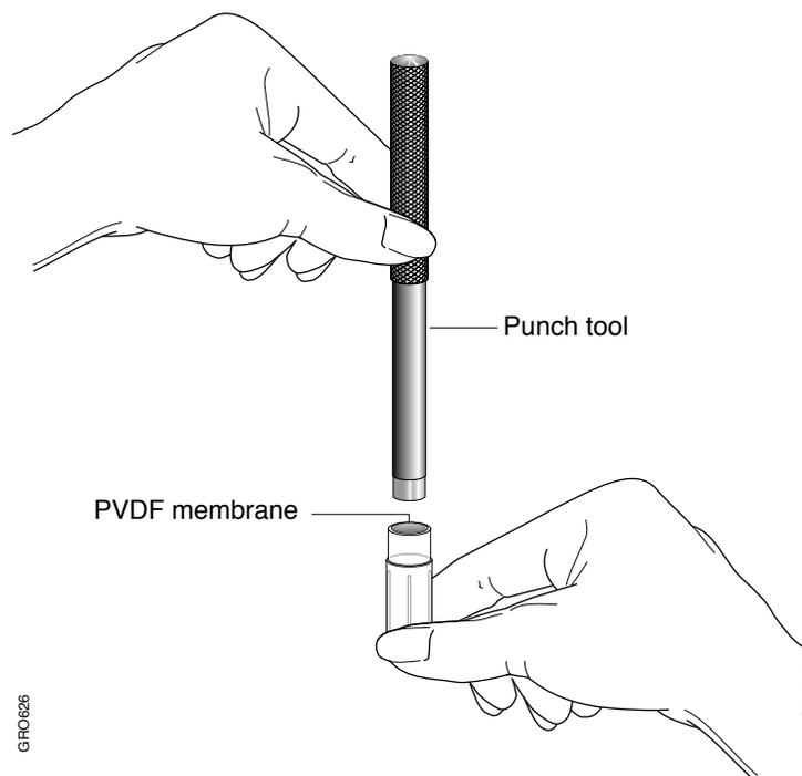
Figure 3-3 Punch the PVDF membrane into the ProSorb sample reservoir insert
