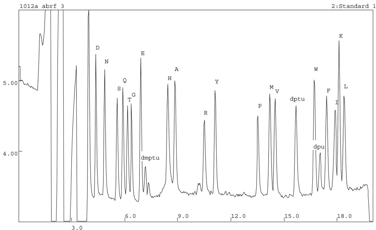
**Figure 4-4** Five pmoles of PTH-amino acid standard was analyzed using solvent B2 and solvent A3 containing Premix Buffer Concentrate. Notice that the DPU is favorably positioned between Trp and Phe.
