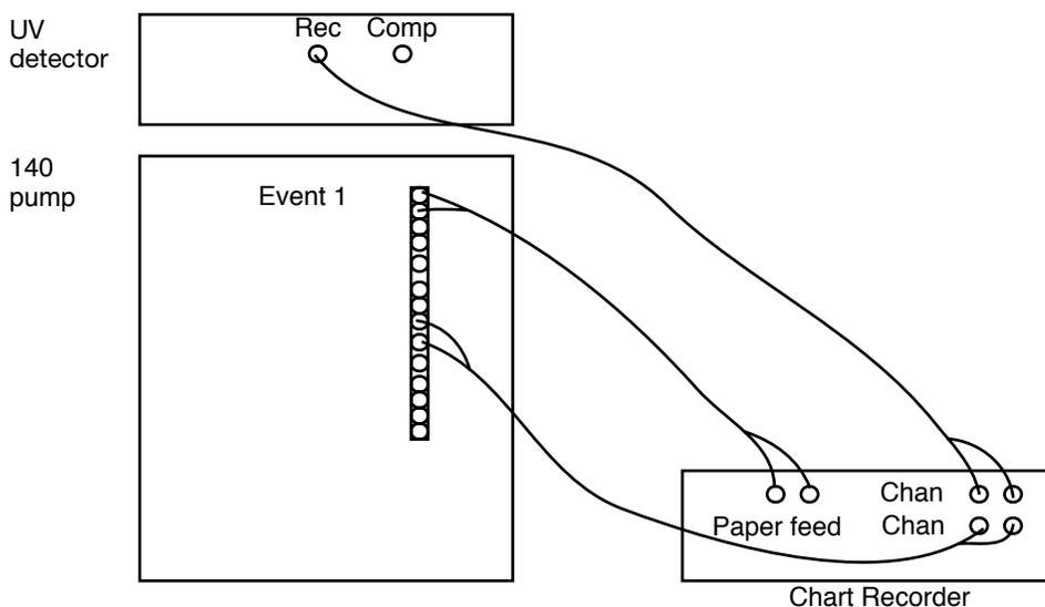
Figure 7-4 Chart recorder cable connections
