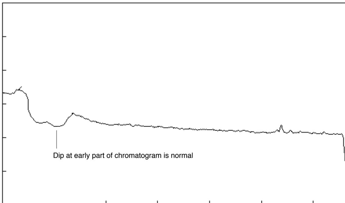
Figure 7-1 Gradient profile with no injection
