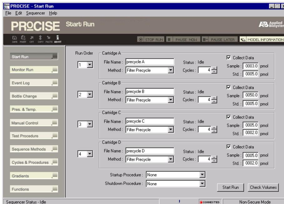
Figure 3-6 Precycling a glass-fiber filter treated with BioBrene
