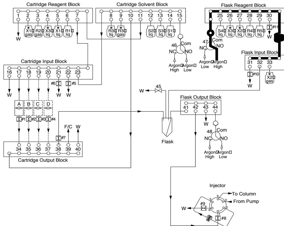
Figure 6-3 Flow path for the Flask Input Leak test
