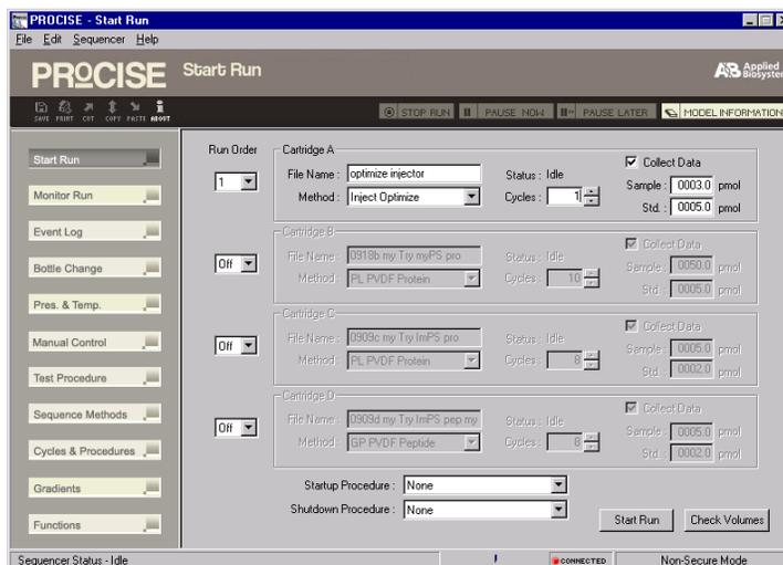
2. Enter the cartridges, methods, and cycles that will be run.
