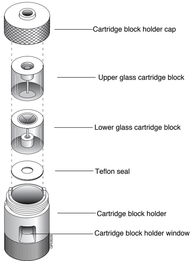
Figure 3-1 6 mm reaction cartridge components in upright position
