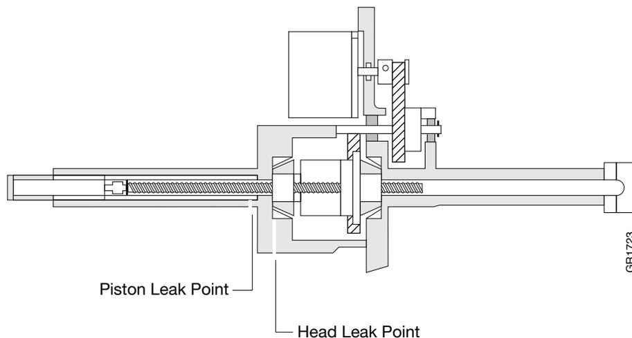
Figure A-6 Pump seal leak points
