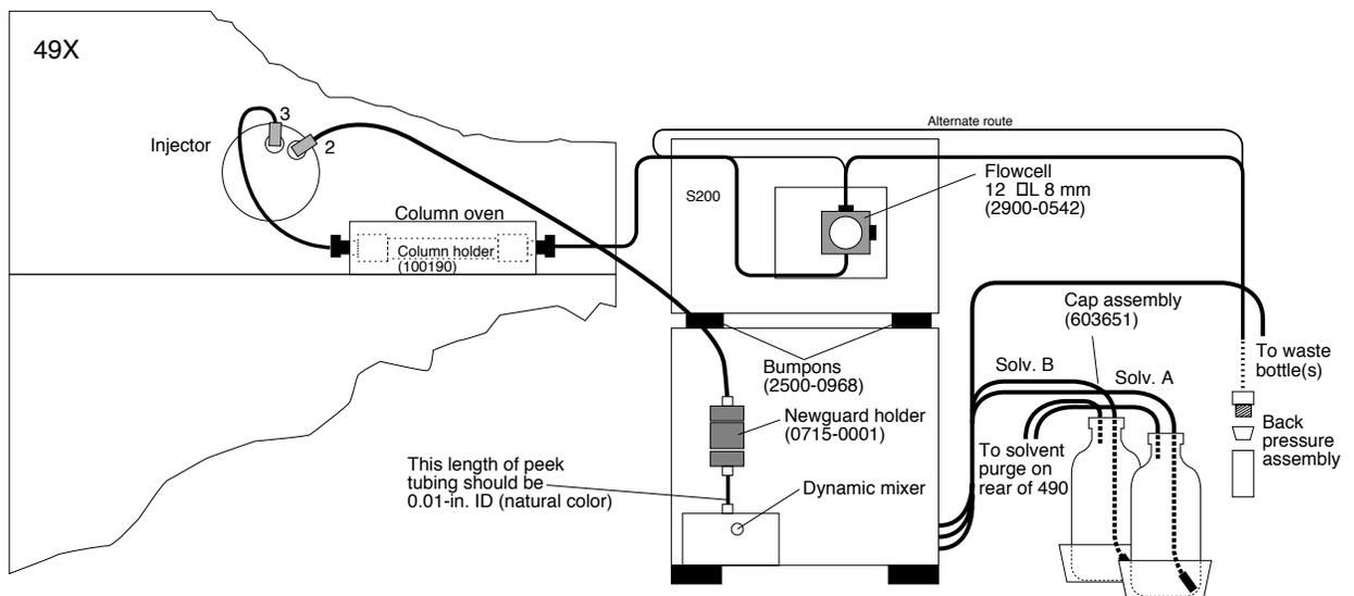
Figure 1-3 PROCISE and PROCISE C plumbing diagram
