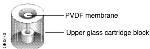
Figure 3-4 PVDF membrane centered in well of upper glass cartridge block
