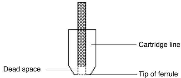
Figure A-10 Incorrectly installed cartridge ferrule
