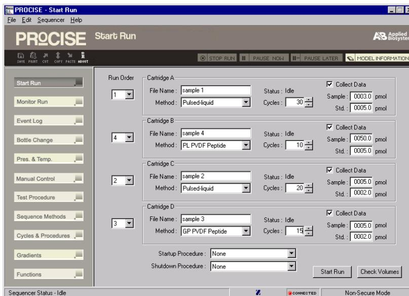
3. Select the cartridge run order. Cartridges can be run in any order. Selecting the run order for a cartridge activates the File name, Cycles and Methods fields.
