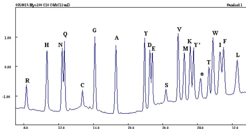
Figure 4-6 Twenty picomoles of ATH-Amino Acid Standard at 4 mAUFS. The separation shown was run with 3.5% THF, 75 mM sodium acetate, 2 mM tetrabutylammonium hydroxide as solvent A. Using tetrabutylammonium hydroxide in place of DIEA as the solvent A additive reverses the elution positions of H and R.
