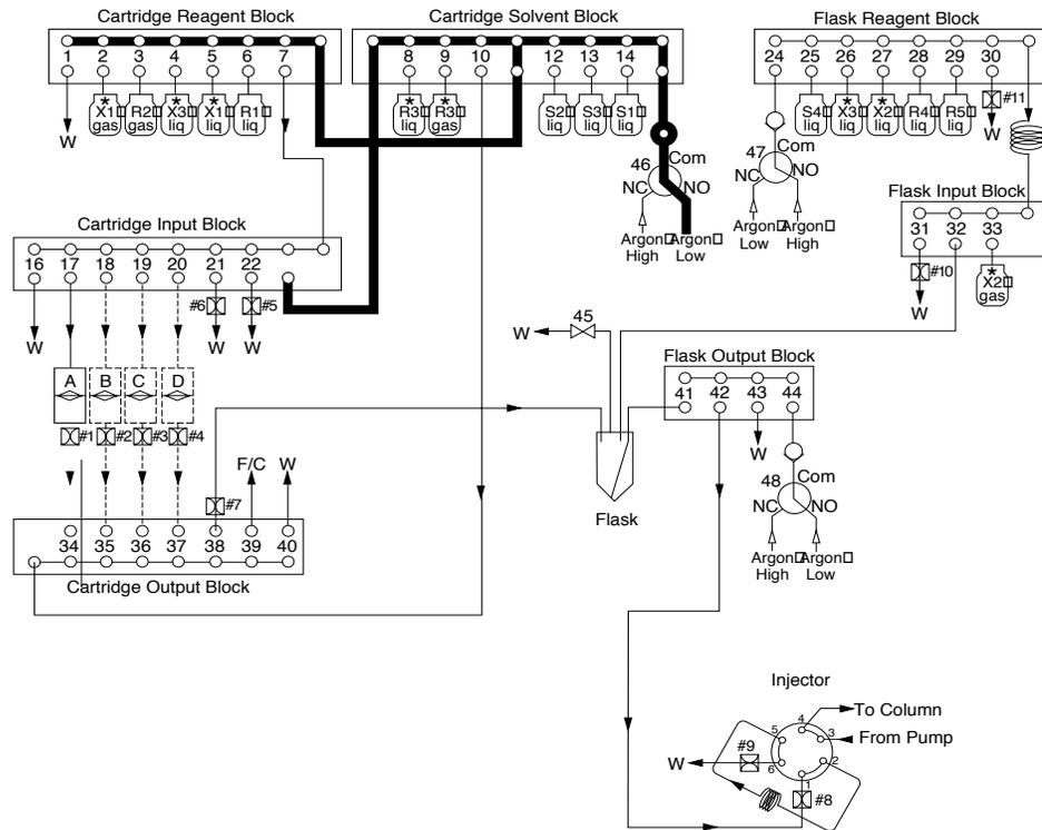
Figure 6-5 Flow path for Cartridge Reagent Block Leak test
