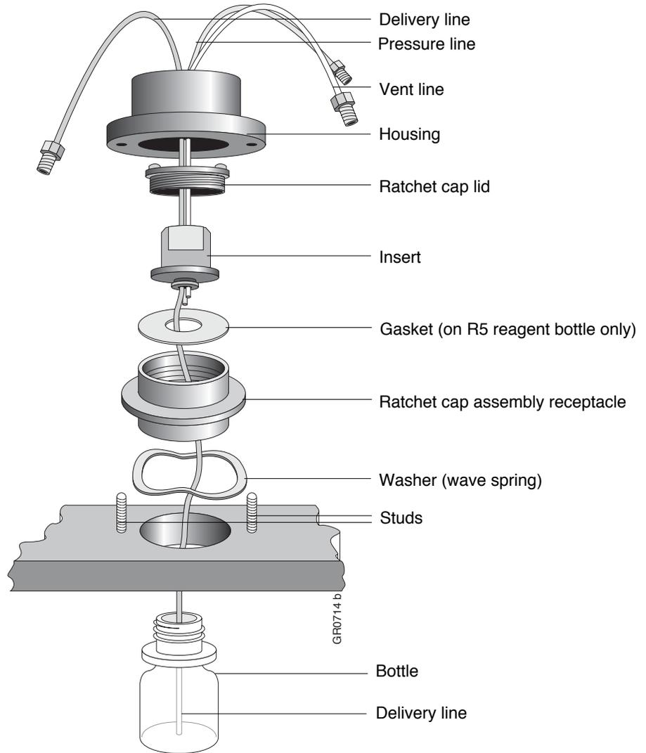
Figure 7-3 R5 reagent bottle ratchet cap assembly
