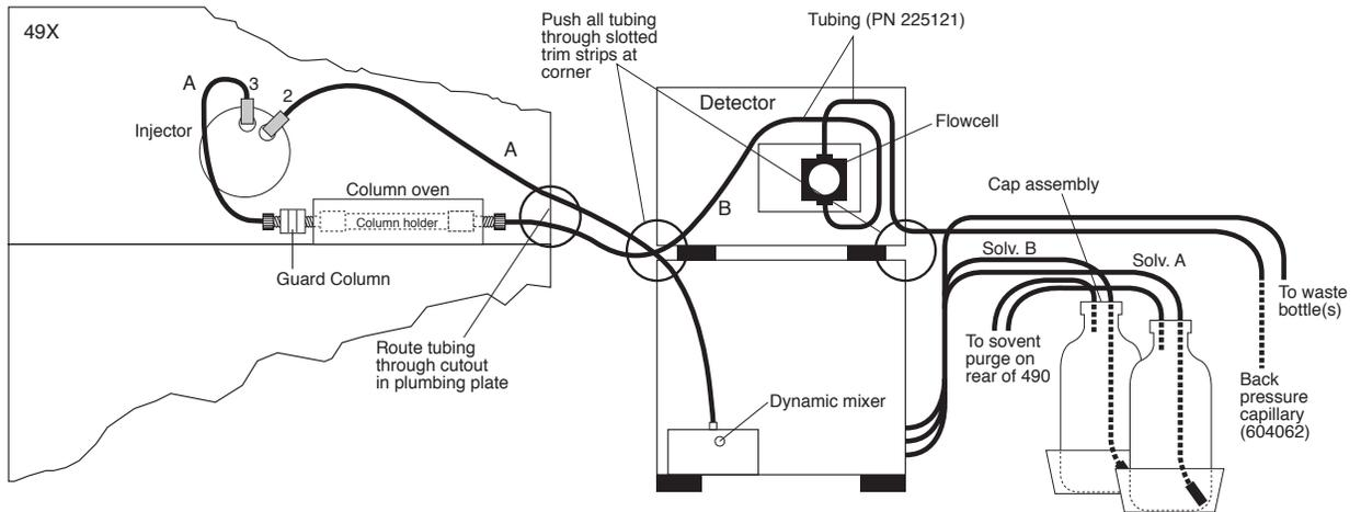
Figure 1-2 PROCISE cLC plumbing diagram
