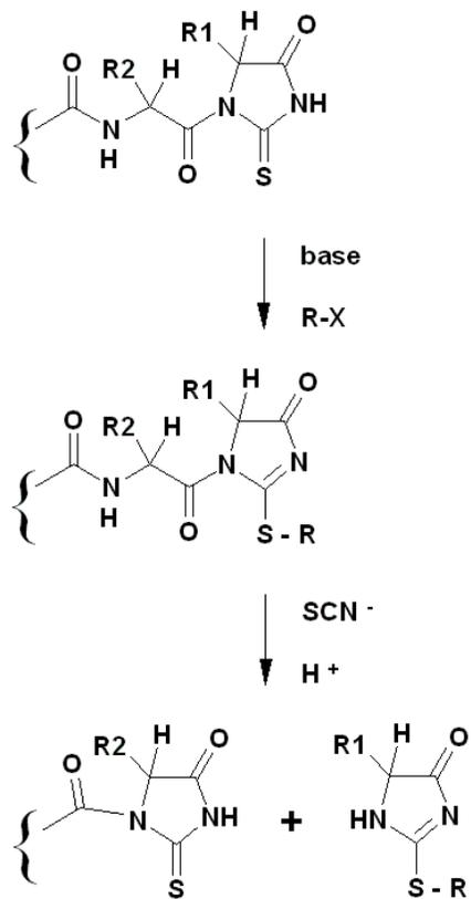
Figure B-6 The Applied Biosystems alkylation chemistry for automated C-terminal protein sequence analysis
