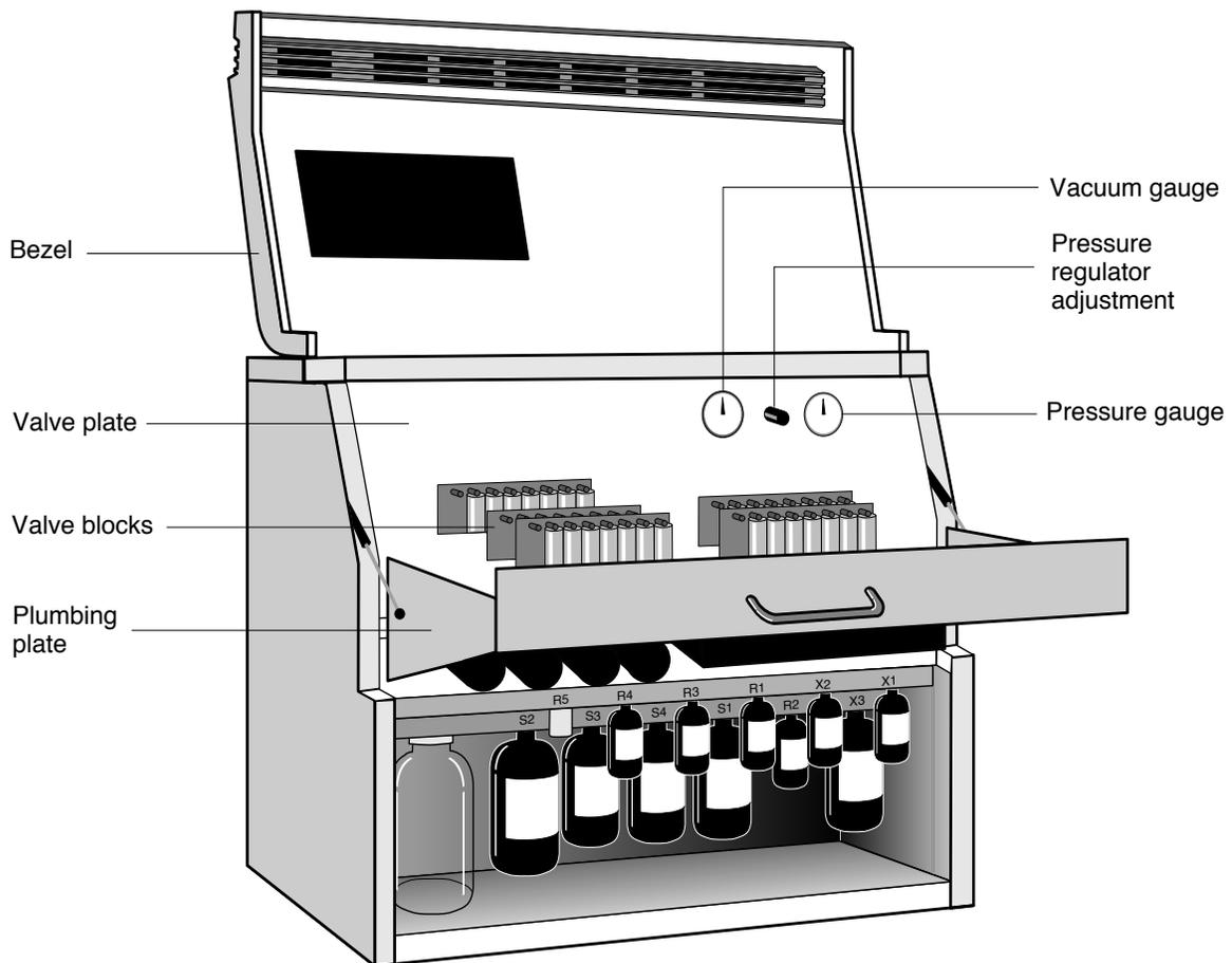
Figure 7-2 User accessibility to the internal components of the protein sequencer
