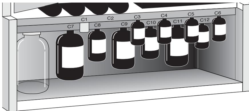
Figure 2-2 PROCISE C protein sequencer bottle configuration
