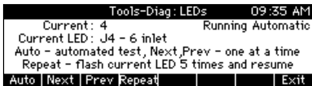
Figure 3-53 LED Test Facility
