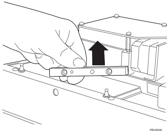
**Figure 2-4 Removing the Transport Bracket**
