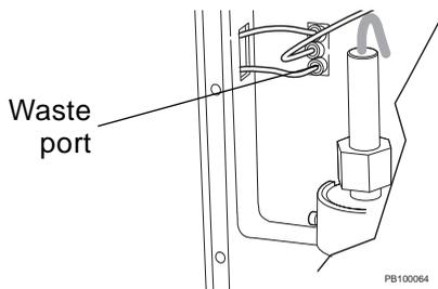
**Figure 2-12 BioCAD 700E Workstation Fraction/Waste Valve**
