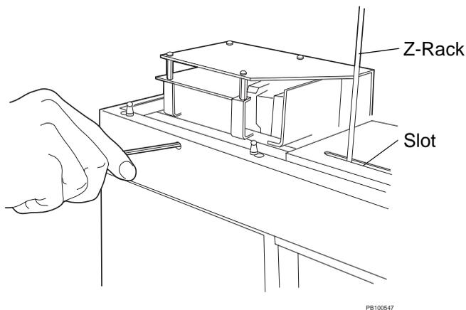
**Figure 2-3 Removing the Transport Screw**
