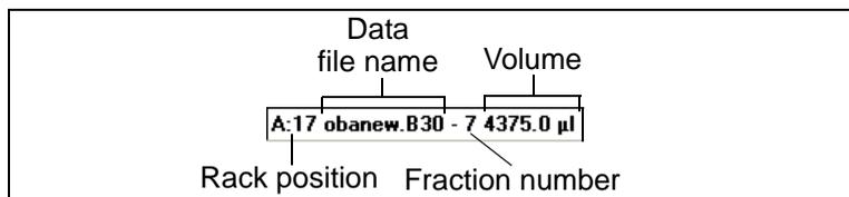
This information about collected fractions is automatically added to the system configuration. The volume is adjusted when an injection is made from that tube.
