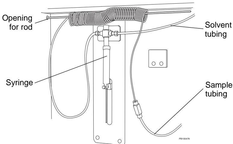
**Figure 3-4 Installing Coiled Tubing**
