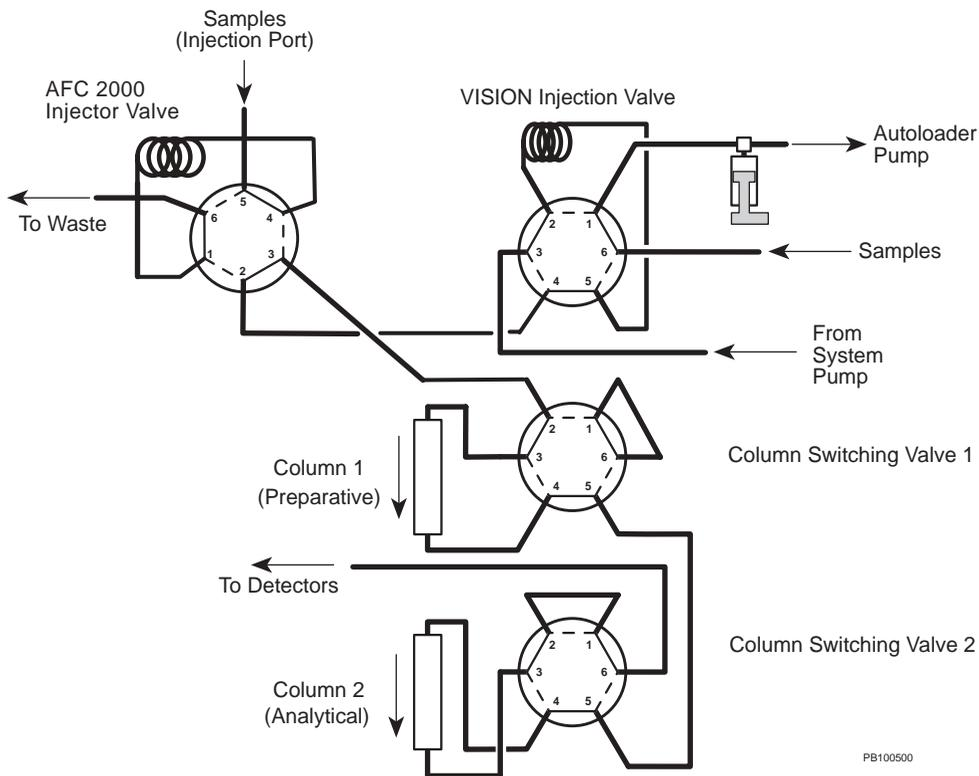
**Figure 4-4 Typical Plumbing Configuration for Automated Analysis**
