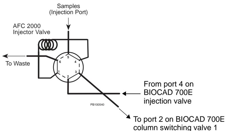
**Figure 2-10 AFC 2000 Injector Valve Plumbing**
