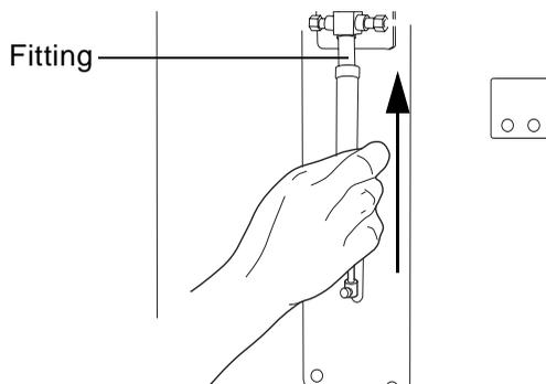
**Figure 3-3 Attaching a Syringe to the AFC 2000**
