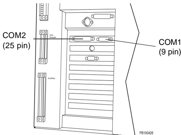
**Figure 2-7 Connecting AFC 2000**
