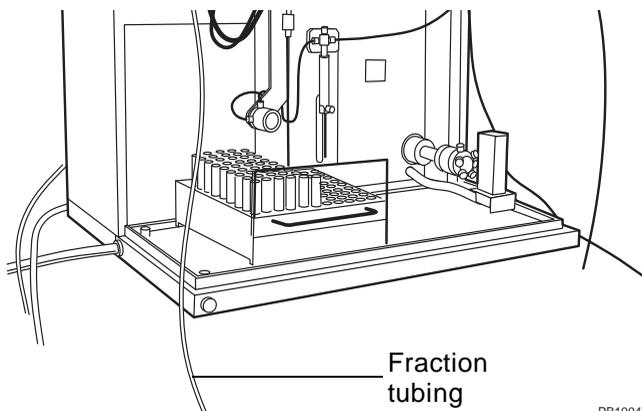
**Figure 2-11 AFC 2000 Fraction Tubing**
