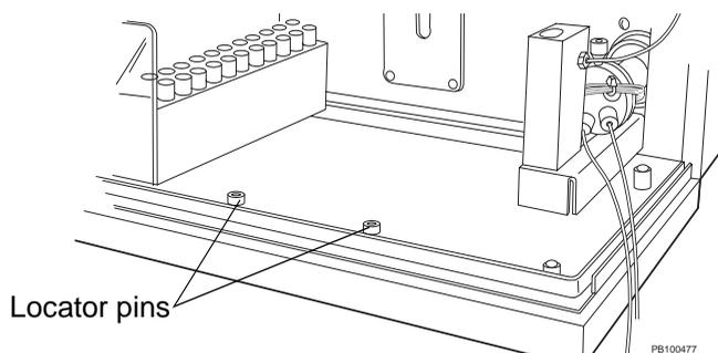
**Figure 3-2 Installing Racks in AFC 2000**
