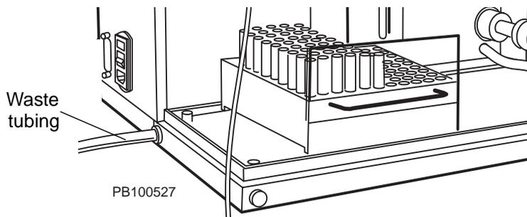
**Figure 2-1 Routing Waste Tubing**
