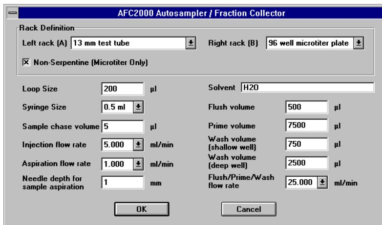
**Figure 3-8 AFC 2000 Autosampler/Fraction Collector Dialog Box**
