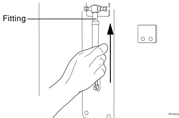
**Figure 5-2 Attaching a Syringe to the AFC 2000**
