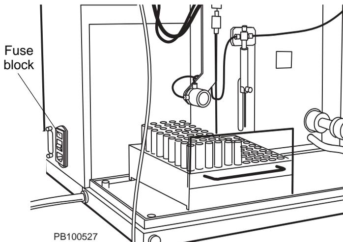
**Figure 5-1 Replacing the Fuses**
