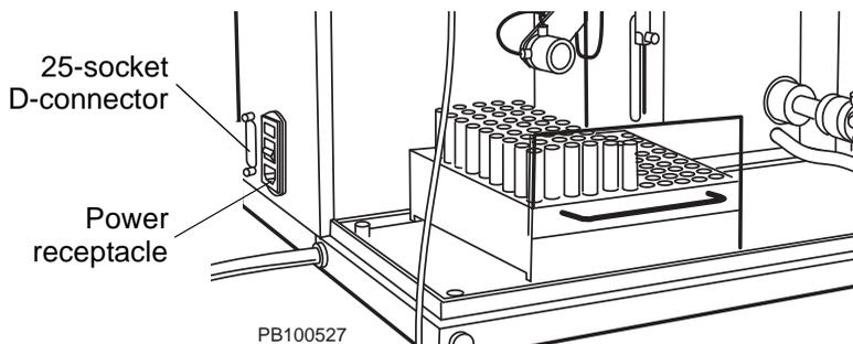
**Figure 2-6 AFC 2000 Power Receptacle and 25-Socket D-Connector**
