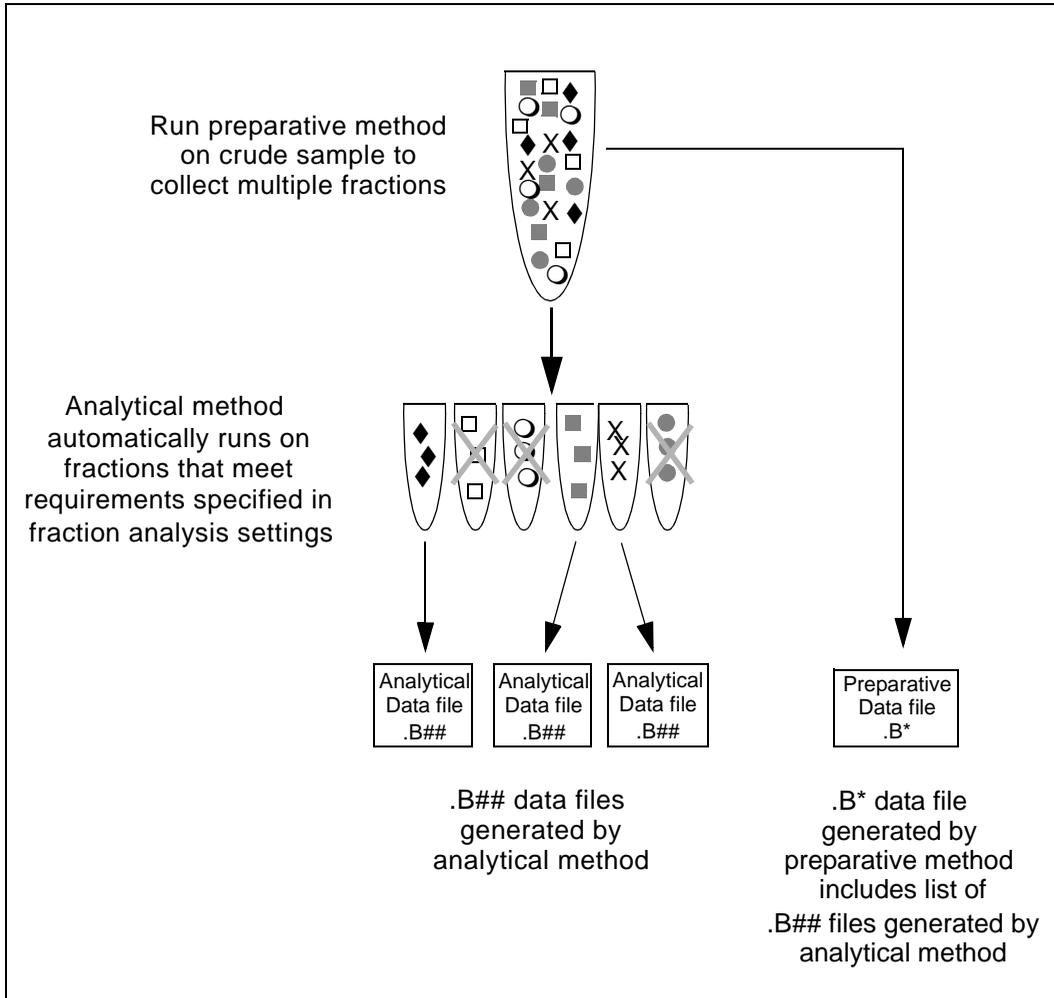
**Figure 4-2 Automated Analysis Process**
