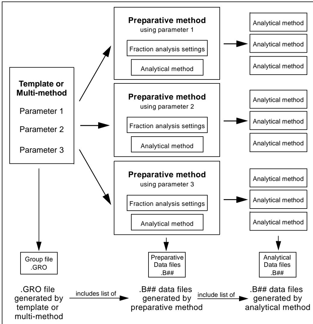
**Figure 4-3 Templates or Multi-Methods with Automated Analysis**
