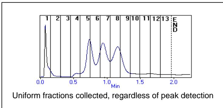
Figure 3-23 Collect Non-Peak Fractions
