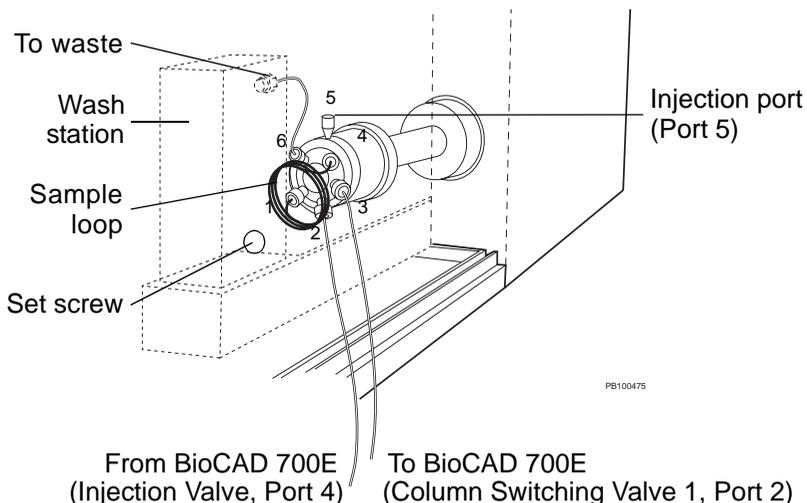
**Figure 2-9 Plumbing Injector Valve
