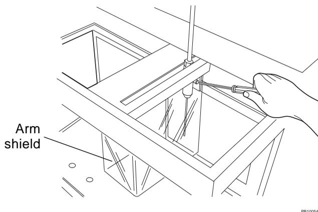
**Figure 2-5 Attaching the Arm Shield**
