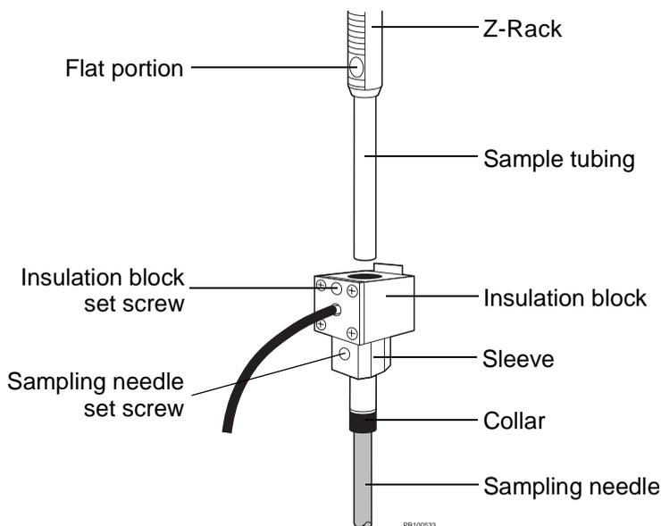
**Figure 5-3 Replacing the Sampling Needle**
