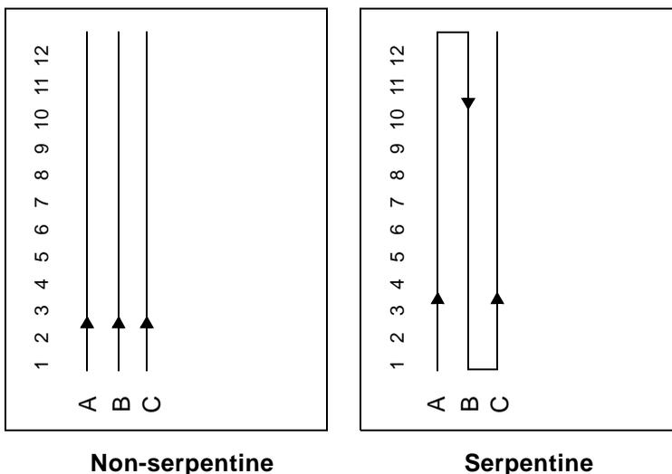
**Figure 3-9 Microtiter Plate Filling Patterns**
