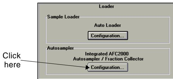
**Figure 3-7 Configuring as an Integrated Fraction Collector**
