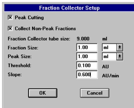
**Figure 3-20 Fraction Collector Setup Dialog Box**
