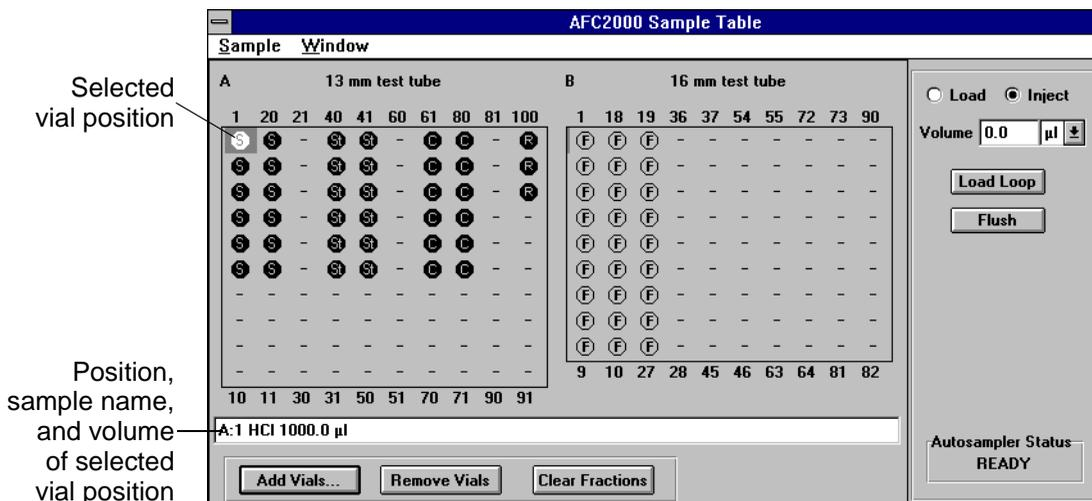
Figure 3-16 AFC 2000 Sample Table Window
