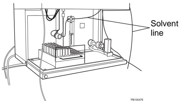
**Figure 3-5 AFC 2000 Solvent Line**
