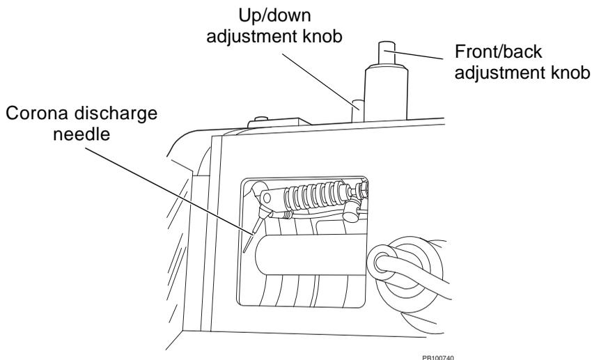
**Figure 2-12 Corona Discharge Needle Location**
