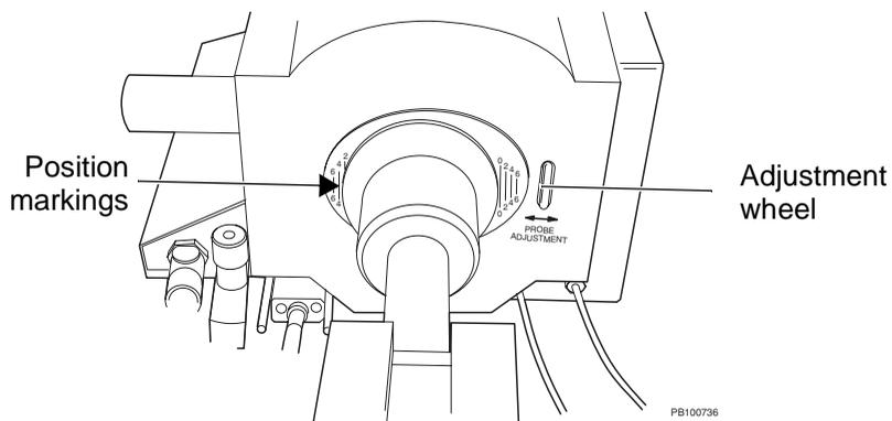
**Figure 2-11 Lateral Probe Gauge Markings on Right Side of Spray Chamber**
