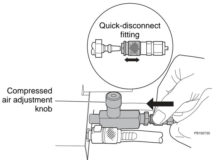
**Figure 2-7 Connecting the Compressed Air to the Spray Chamber**
