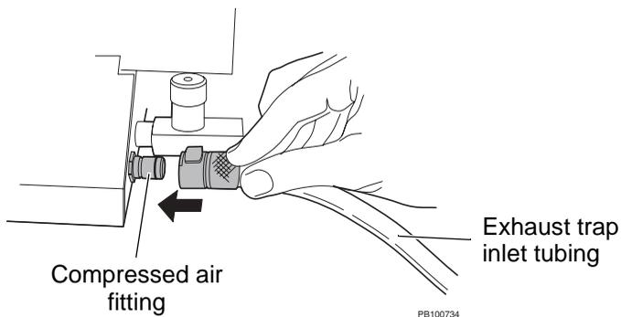
**Figure 2-4** *Connecting the Exhaust Trap Line to the Spray Chamber*
