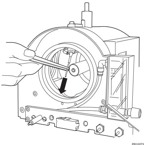
**Figure 4-1 Replacing the Corona Discharge Needle**
