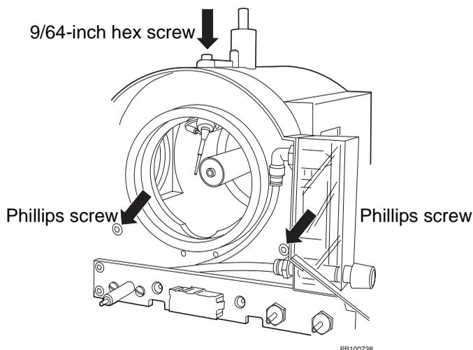
**Figure 4-2 Removing the Spray Chamber from the Base**
