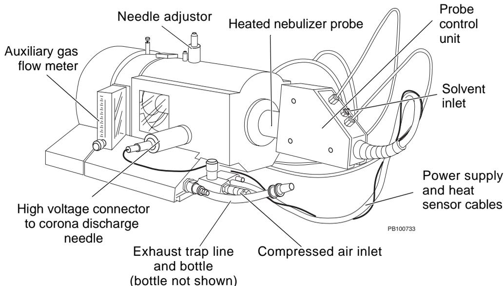
**Figure 1-2 Parts of the APCI Module**
