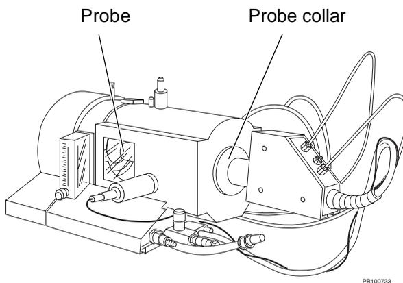
**Figure 2-10 Positioning the APCI Probe**
