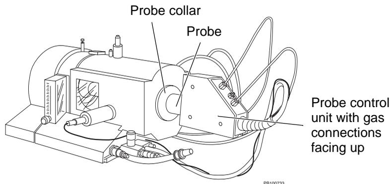
**Figure 2-3 Installing the Heated Nebulizer Probe**
