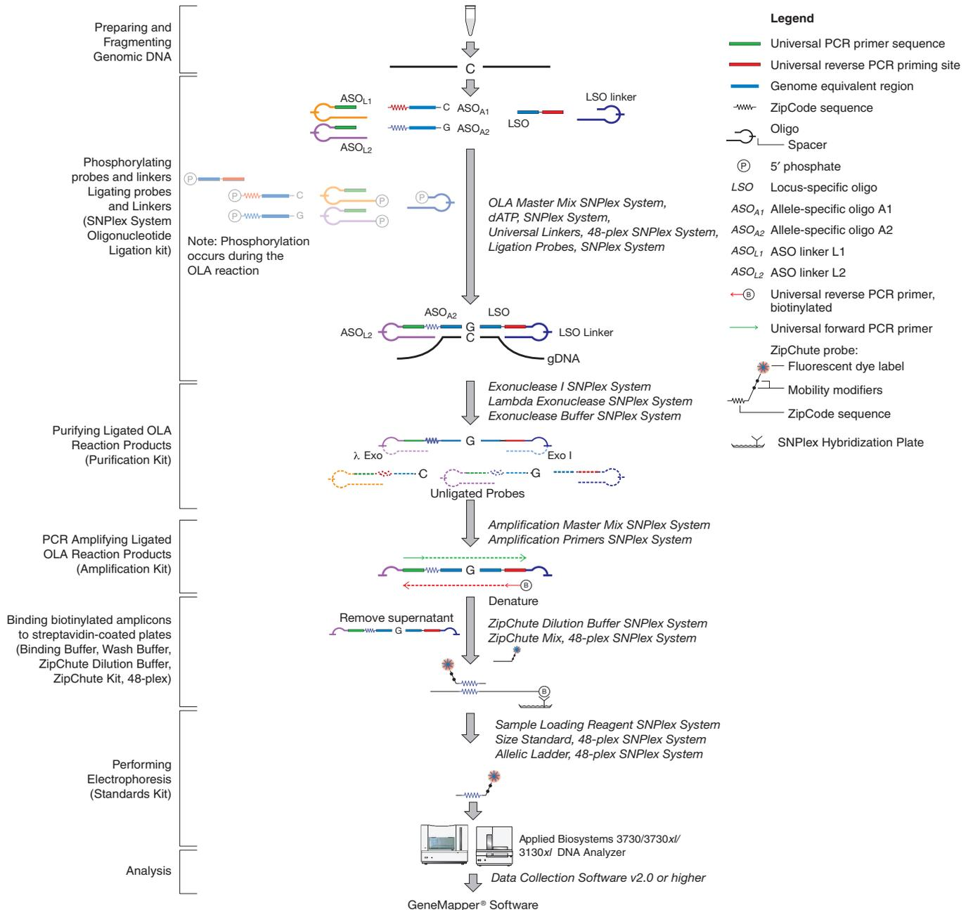
Figure 1-3 Summary of the SNiPlex System Assay process
