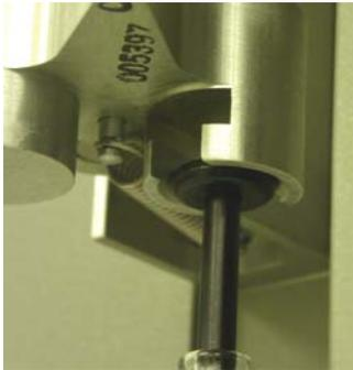
NOTE: After executing the SYRINGE HOME command, the syringe pump must be brought back down on top of the plunger. Ensure that the pump is close to but not compressing the syringe plunger. If the syringe pump is not returned to this position prior to a run – the instrument will generate a “Leak Detected” error.
