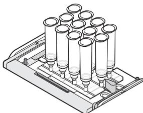
**IMPORTANT!** Make sure each reservoir sits properly on the filter vial by pressing firmly to ensure a tight seal.
