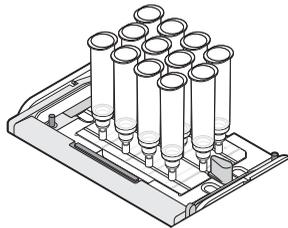
**Note:** If all the samples have not passed through the filters in the specified time, run the vacuum for additional time until all samples are completely evacuated.
