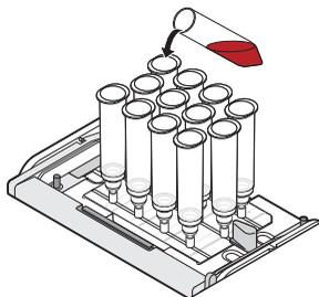
**Note:** If all the samples have not passed through the filters in the specified time, run the vacuum for additional time until all samples are completely evacuated.
