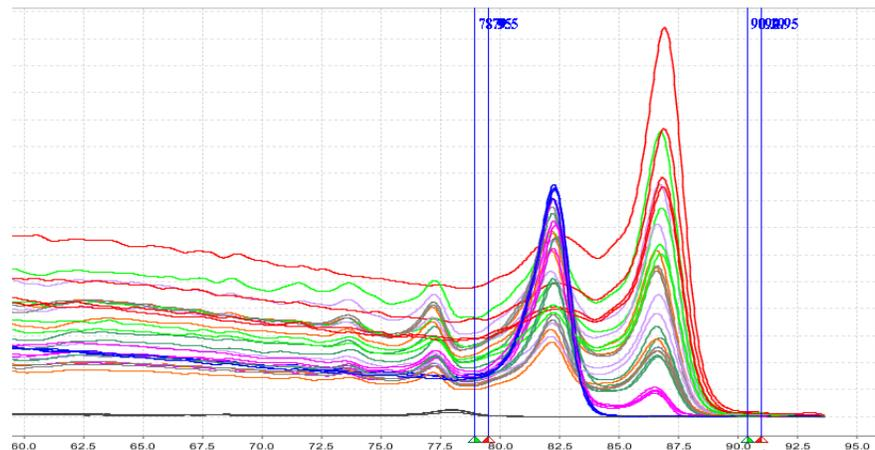
Set the post-melt Start next to the end of the melting transition
