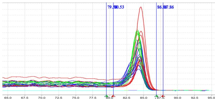
Set the post-melt Start next to the end of the melting transition
