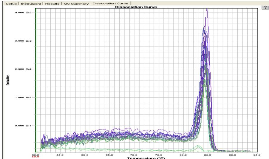
**Note:** If the Dissociation Curve contains more than 1 T<sub>m</sub> Peak, more than one PCR product was produced. Contact an Applied Biosystems representative to identify and resolve the problem.
