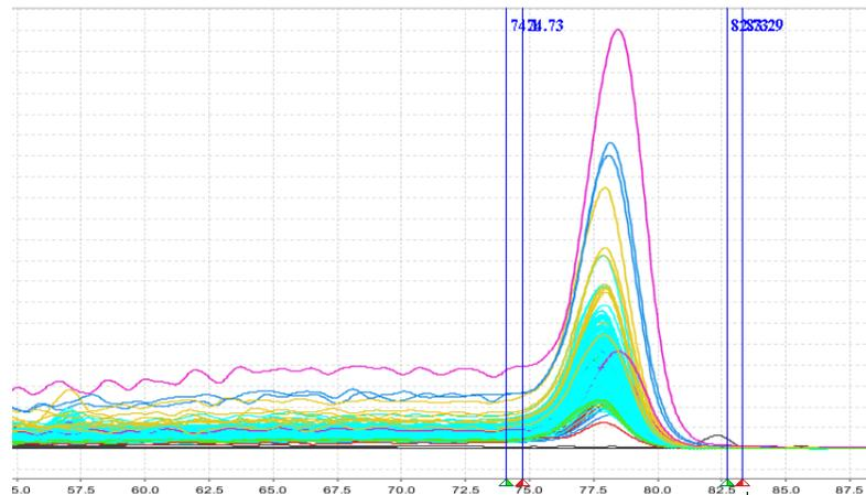
Set the post-melt Start next to the end of the melting transition
