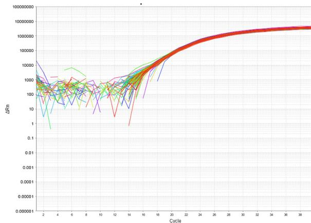
**Note:** If the Amplification Plot looks abnormal, contact an Applied Biosystems representative to identify and resolve the problem.
