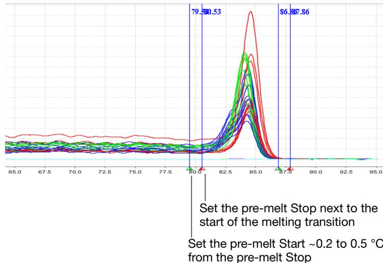
**Note:** The pre-melt region should be within a flat area where there are no large spikes or slopes in the fluorescent levels.
