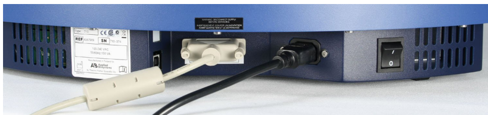
Fig. 5.8 Mains supply cable and serial cable connected
