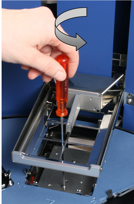
Fig. 5.20 Unfastening the transport lock screw from its storage site
