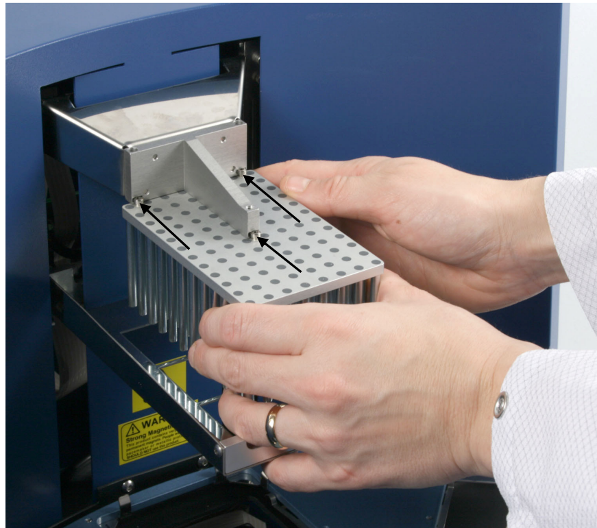
Fig. 5.17 Inserting the MagMAX™ Express 96 head
