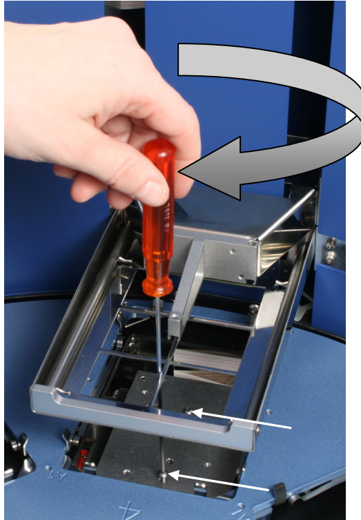
Fig. 5.7 Fastening the transport lock of the heating block to its storage site
